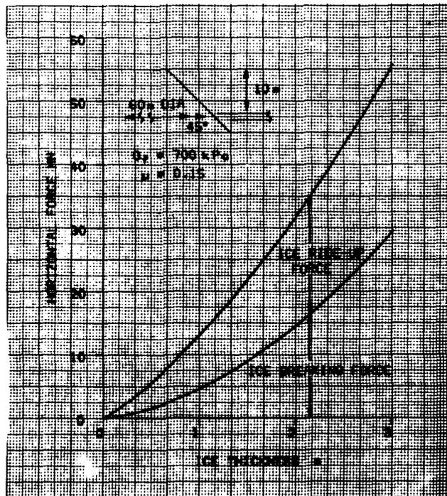
Figure 18. Horizontal force vs ice thickness - wide structure (Ralston's theory).
