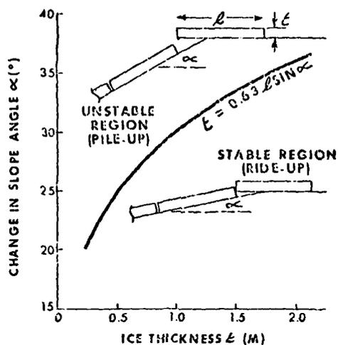
Figure 41. Criterion for ride-up past a change in slope.
