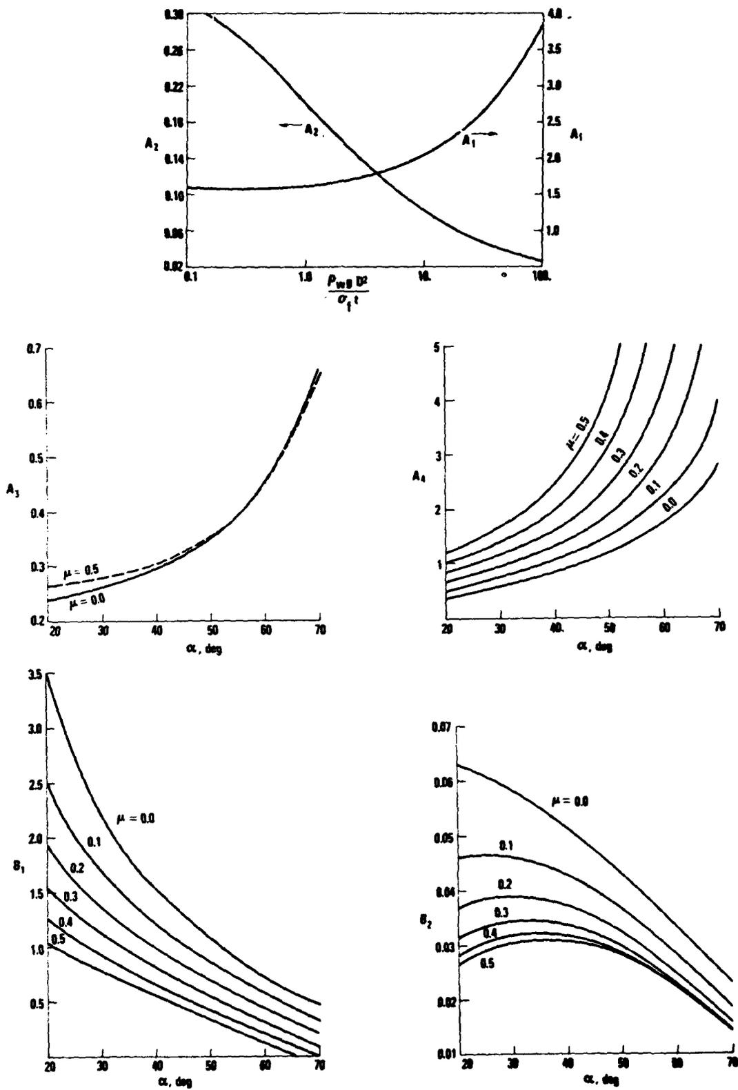
Figure 16. Ice force coefficients for plastic analysis (Ralston 1977).
