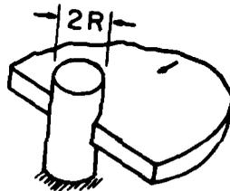
Figure 7. Geometry of a semi-infinite floating ice sheet moving against a rigid cylindrical structure.
