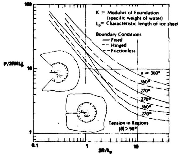
Figure 12. Plots of buckling pressure  $P/(2RKL_p^2)$  with respect to  $2R/L_p$  when wedge-angle  $\alpha$  is greater than  $\pi$  and when  $P$  creates a compressive as well as tensile stress field.
