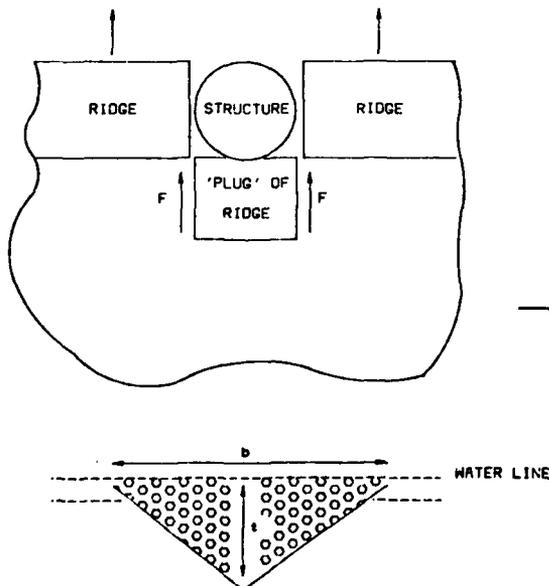
Figure 21. Simple interaction model for unconsolidated ridge.
