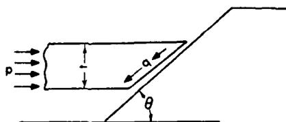
Figure 37. Adfreeze bond failure.
