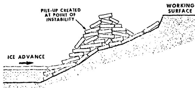
Figure 44. Design to resist ice ride-up.
