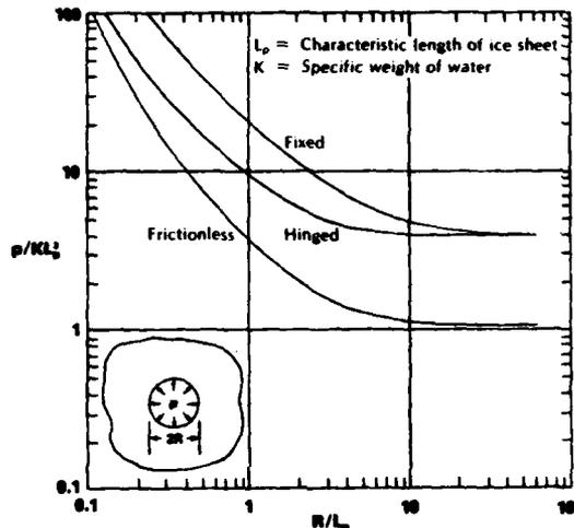
Figure 5. Plots of the lowest buckling pressure  $p/(KL_p^2)$  with respect to  $R/L_p$  for an infinite ice sheet stressed uniformly along the periphery of an internal hole (Takagi 1978).
