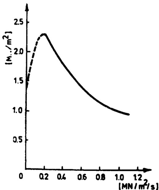
Figure 3.3 Crushing strength vs. strain rate, Peyton (17)
