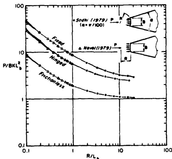
Figure 4. Plot of nondimensional buckling pressure  $P/(BKL_b^2)$  of a tapered beam with respect to  $R/L_b$ .
