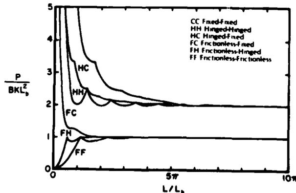
Figure 2. Lower envelope plots of nondimensional buckling pressure  $P/(BKL_b^2)$  with respect to the ratio of length to characteristic length,  $L/L_b$ .
