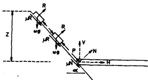
Figure 7. General interaction between ice and sloping structure.
