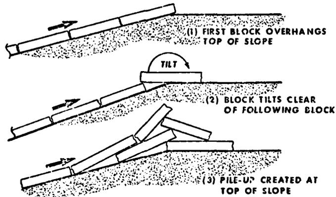
Figure 40. Kinematic instability (pile-up at top of slope).
