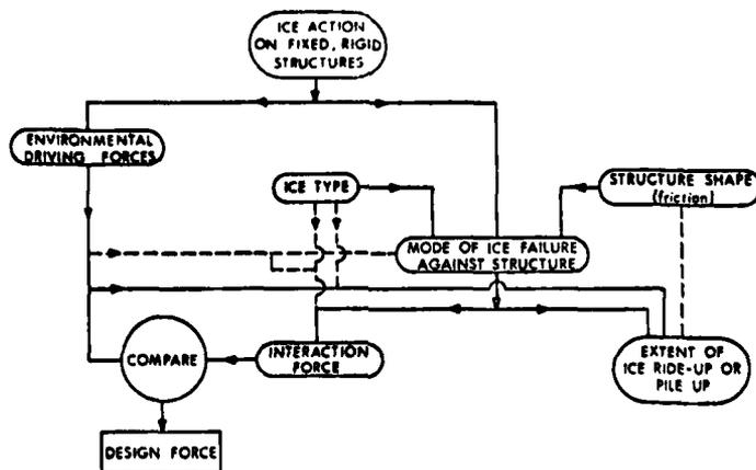
Figure 5. Logic for considering ice action on fixed, rigid structures.
