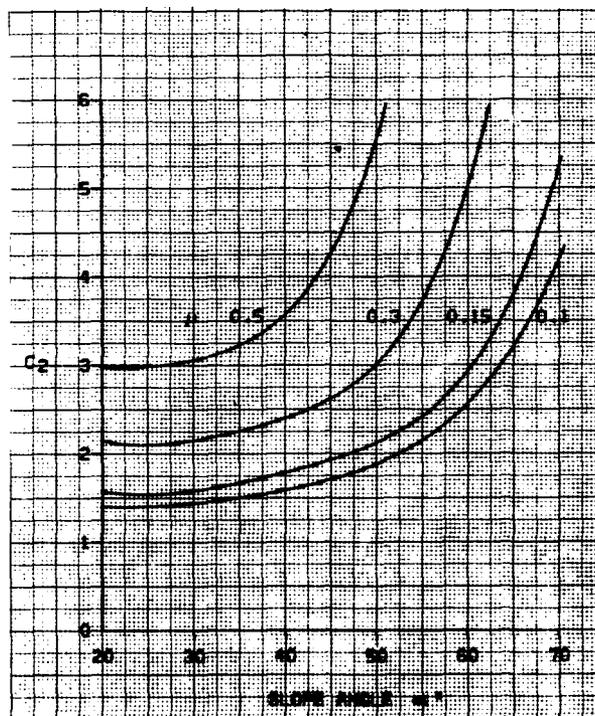
Figure 9.  $C_2$  vs slope angle and friction.
