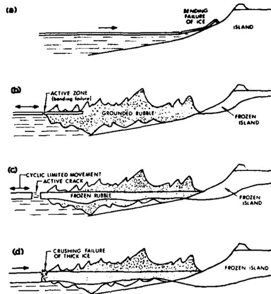
Figure 34. Sequence of ice action on island beach (exposed island): (a) initial movements of thin ice, (b) extensive ice movement causes grounded rubble, (c) active zone remains outside rubble that freezes, (d) thick ice fails in crushing.
