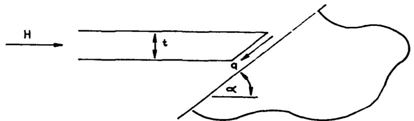
Figure 22. Adfreeze bond failure.
