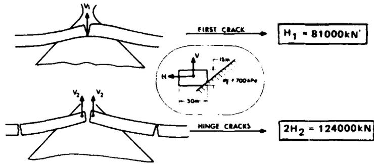
Figure 19. Ridge failure on cone.
