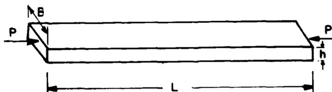
Figure 1. Geometry of a beam with a rectangular cross section resting on an elastic foundation with compressive axial load P.
