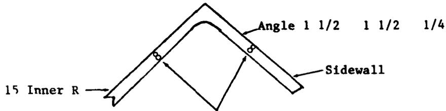
Full Penetration Butt Weld--Typical
