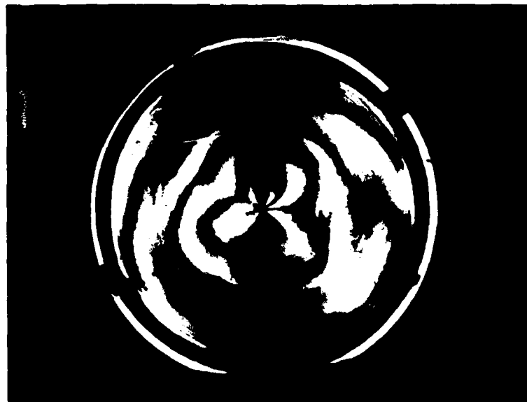
Fig. 7. Alignment interferogram for the annular leg of the HSURIA with a rear flat
