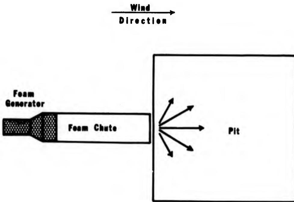
FIGURE 20. PLAN VIEW OF PIT SHOWING PLACEMENT OF HIGH EXPANSION FOAM GENERATOR AND FOAM CHUTE.
