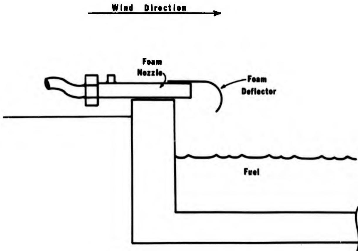
FIGURE 19. CROSS SECTION OF PIT SHOWING PLACEMENT OF LOW EXPANSION FOAM NOZZLE AND DEFLECTOR.
