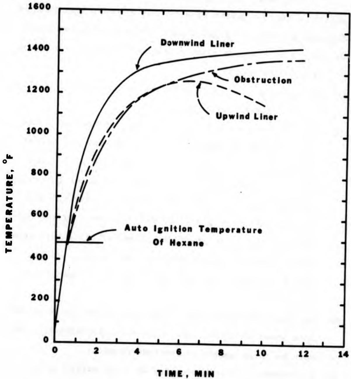
FIGURE 37. TYPICAL PIT LINER AND OBSTRUCTION TEMPERATURES.
