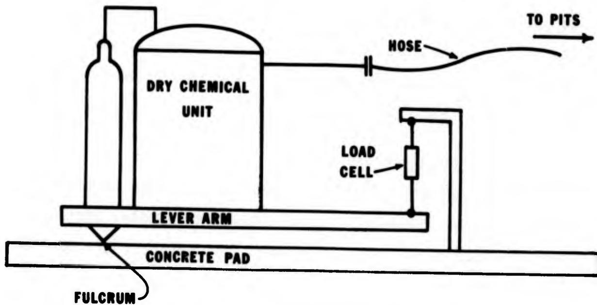
FIGURE 16. DRY CHEMICAL UNIT WEIGHING SYSTEM TO OBTAIN FLOW RATE DATA.
