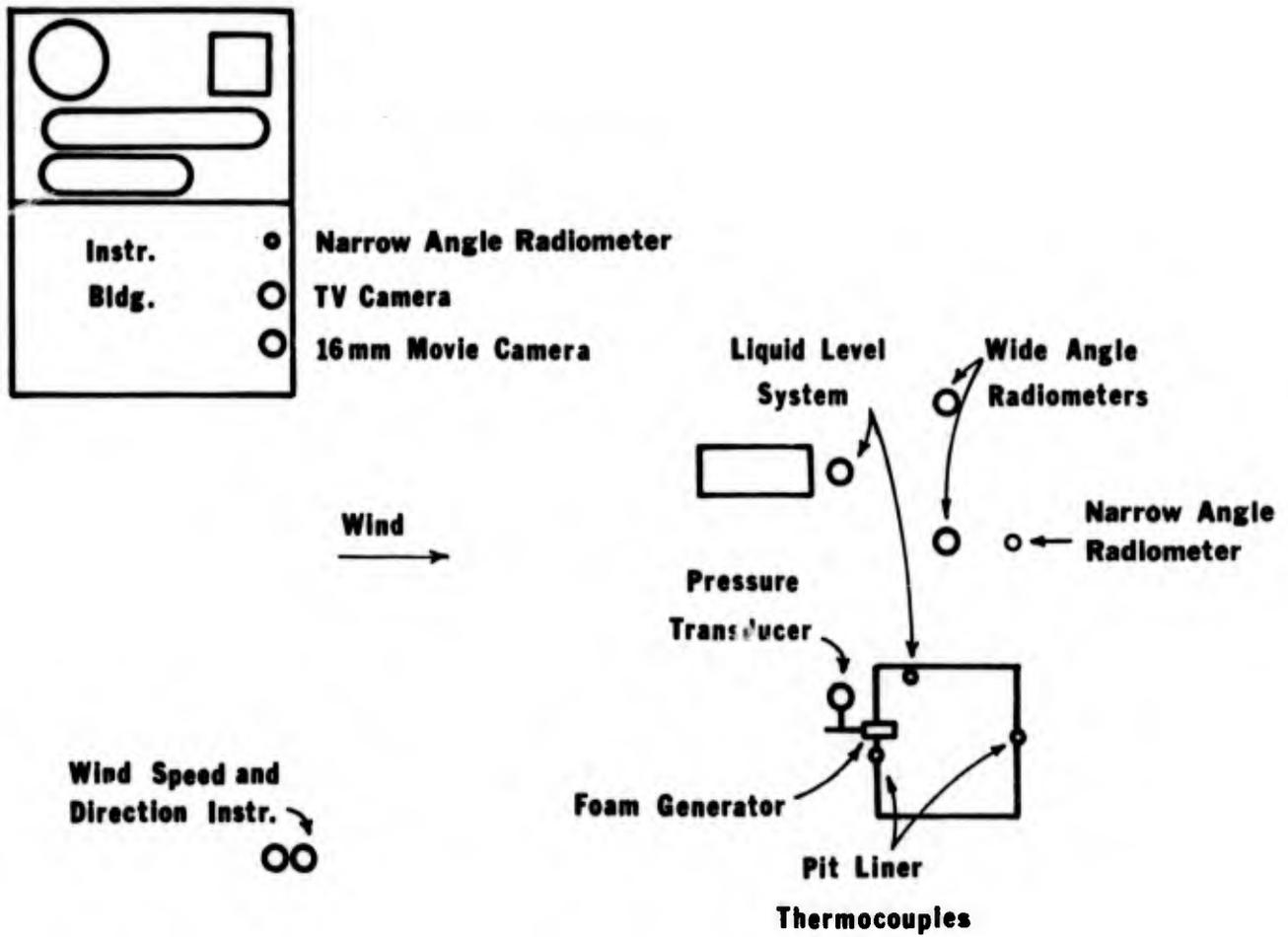
FIGURE 18. EQUIPMENT PLACEMENT FOR TYPICAL FOAM TEST.
