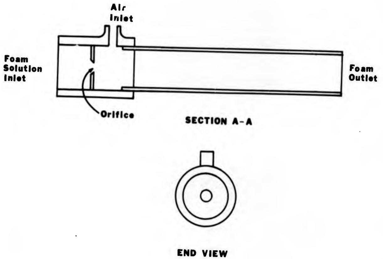
FIGURE 7. DESIGN OF TANK SIDE LOW EXPANSION FOAM NOZZLES.
