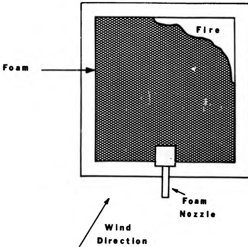
FIGURE 28. PLAN VIEW OF FIRE PIT SHOWING LOW EXPANSION FOAM COVERAGE AND LAST AREA OF FIRE TO BE EXTINGUISHED UNDER WINDY CONDITIONS.
