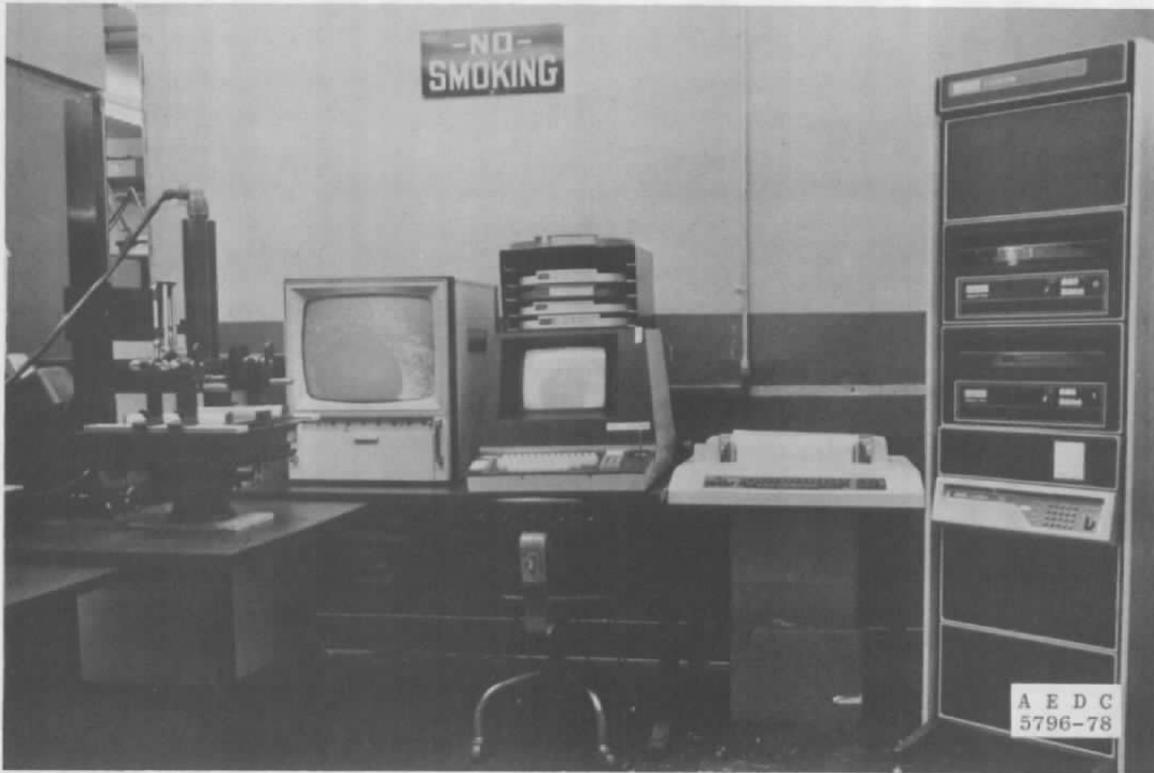
Figure 19. Image analyzer-digitizer system.
