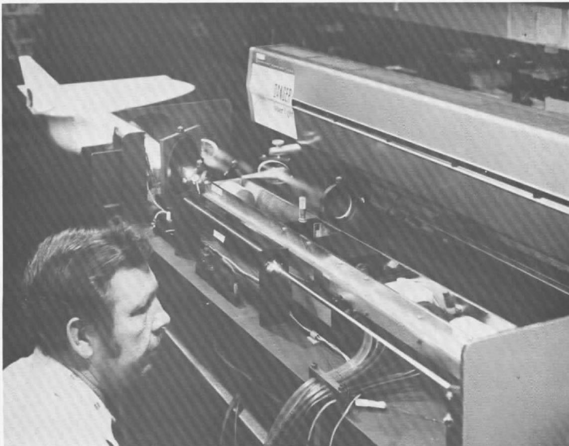
**Figure 8. Lab setup - diffuse reflection holographic flow visualization system.**
