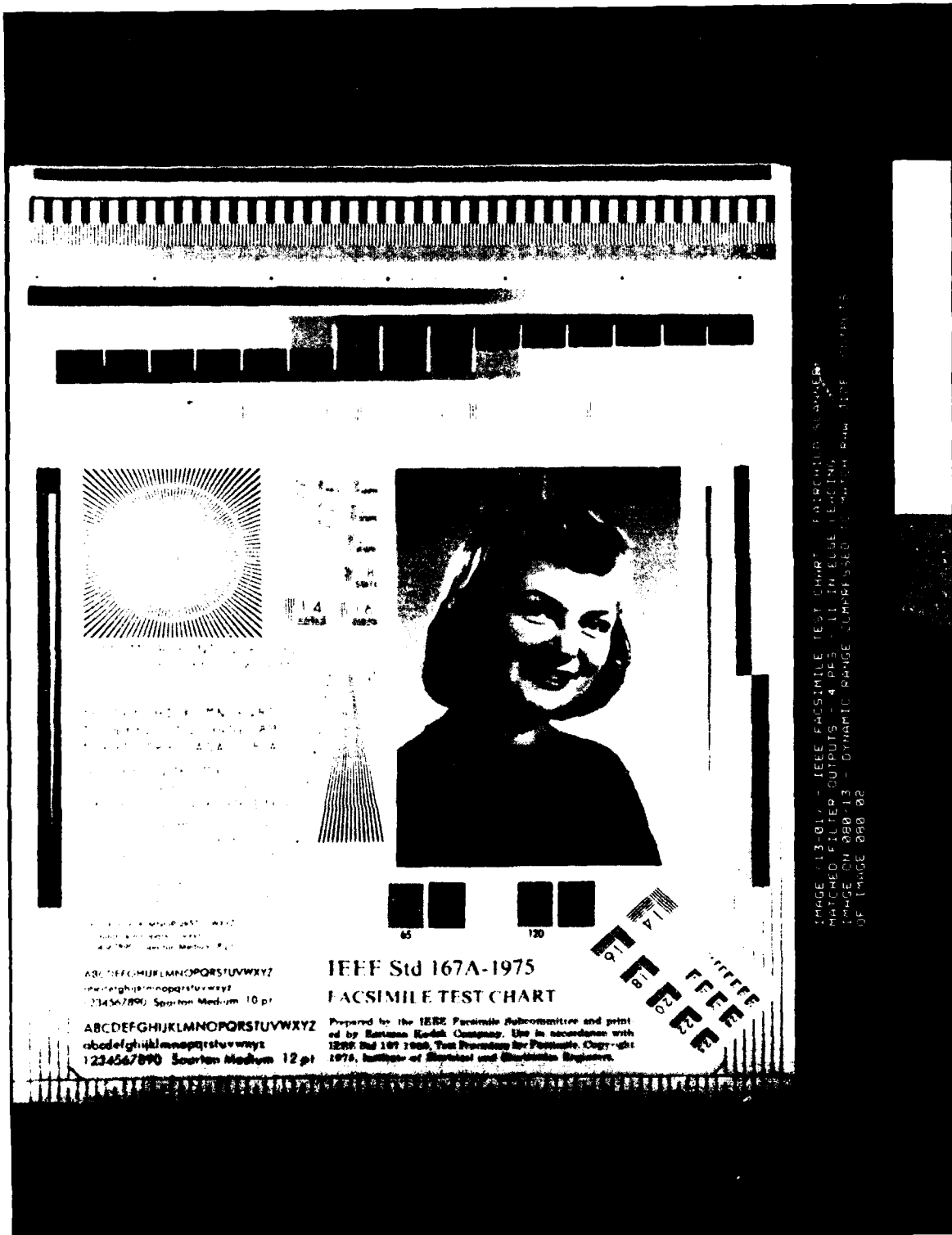
Figure D76. Dynamic range compressed.
