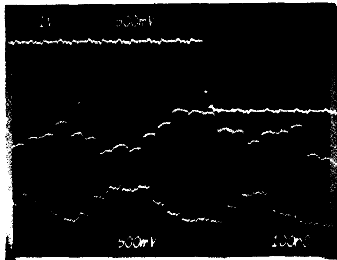
14. Top trace - Video Valid, second trace - channel 1 combined video, third trace - channel 2 combined video. This is intended to show the overlap or left right alignment of an expanded scale. Video Valid signal is active high true.
