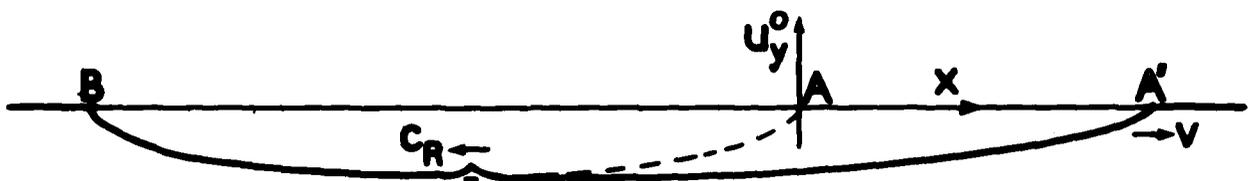
Fig. 2: The displacement of the lower half of the crack surface,  $u_y^0 = u_y(x, y \rightarrow 0^-, t = l/c_L)$ . The dashed curve shows the initial crack opening. A' is the current position of tip A. The depth of the crack relative to its length was determined by setting  $\sigma(1-\nu)/2\mu = 1$ .
