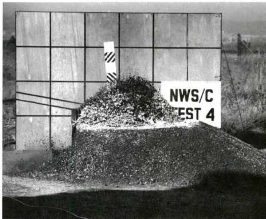
Figure B-2. View of test magazine near time of maximum roof response -- Test 4.
