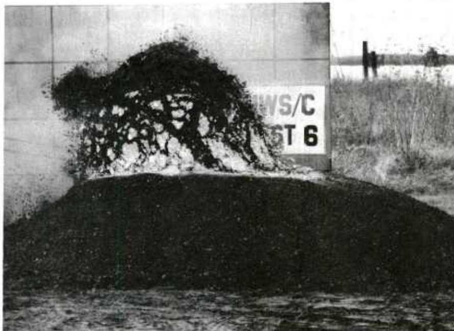
Figure B-10. View of test magazine near time of maximum roof response -- Test 6.
