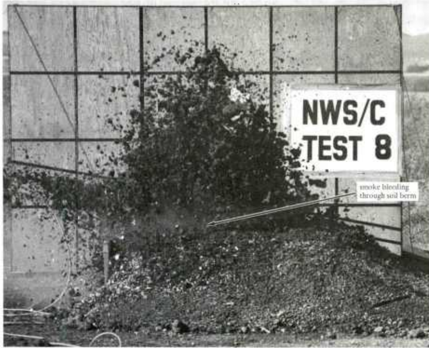
Figure B-19. View of test magazine showing escape of gases through soil berm – Test 8.
