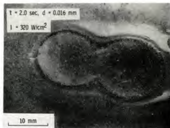
Figure 5. Damage to a 0.016-mm-thick coating of silicon nitride after exposure to a CW 10.6- \mu m laser for 2 seconds at intensity I = 320 \text{ W/cm}^2 . Mag. 3.5X.
