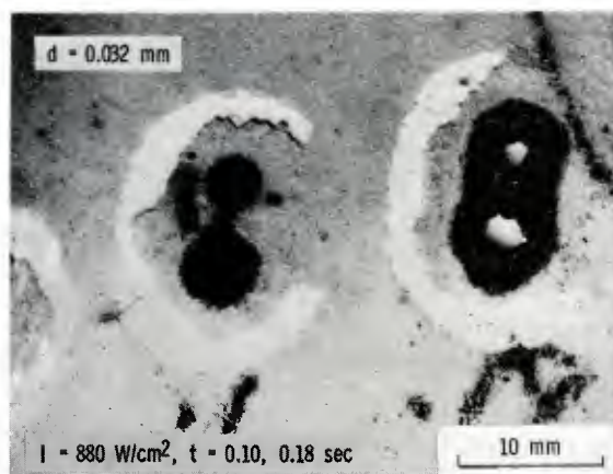
Figure 6. Damage to a 0.032-mm-thick coating of silicon nitride after exposure to a CW 10.6- \mu m laser for 0.10 second (left) and 0.18 second (right) at intensity I = 880 \text{ W/cm}^2 . Mag. 3.5X.
