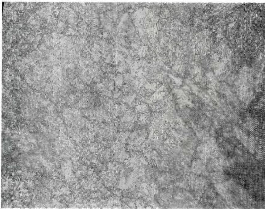
FIG. 6 - Photomicrograph showing recrystallization at the prior austenitic grain boundaries in Forging 6303 for the 732°C (1350°F) treatment.
