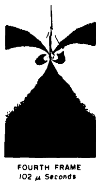
Fig. 6 Typical Crack Branching Dynamic Photoelastic Patterns Homalite-100 Single Edge Notched Specimen (Fixed Grip Loading) Specimen No. B8.
