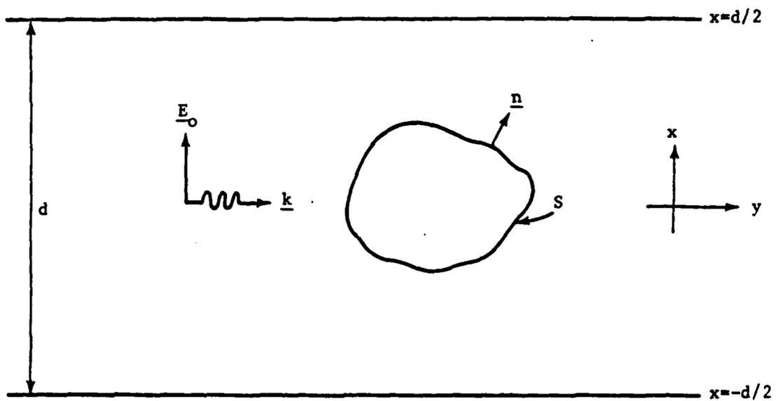
Figure 4. A perfectly conducting body within a parallel plate region.
