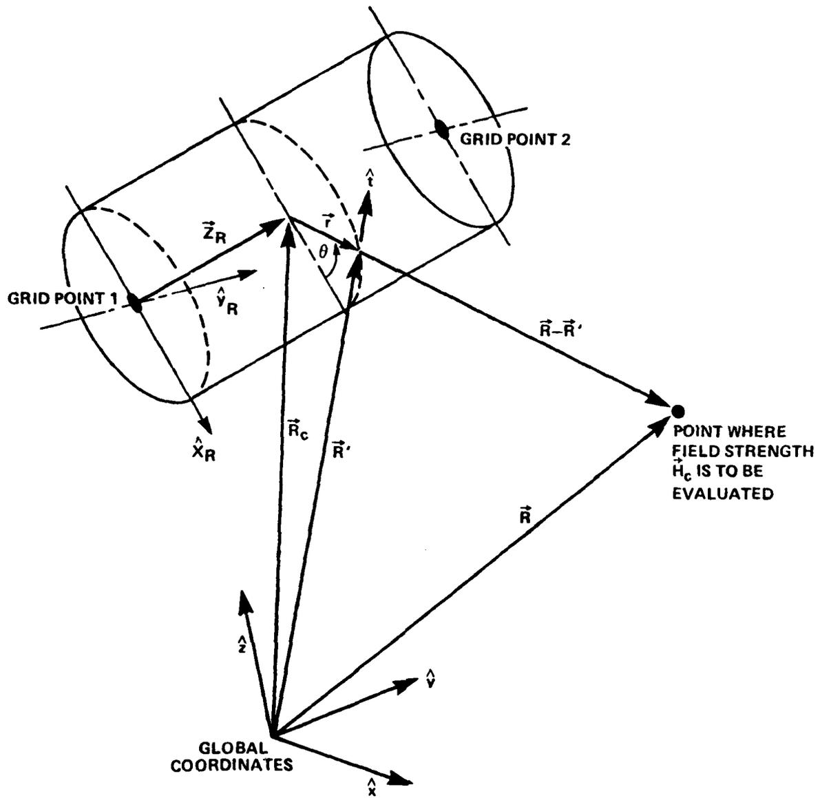
Figure 2. Rod Geometry and Coordinate Systems
