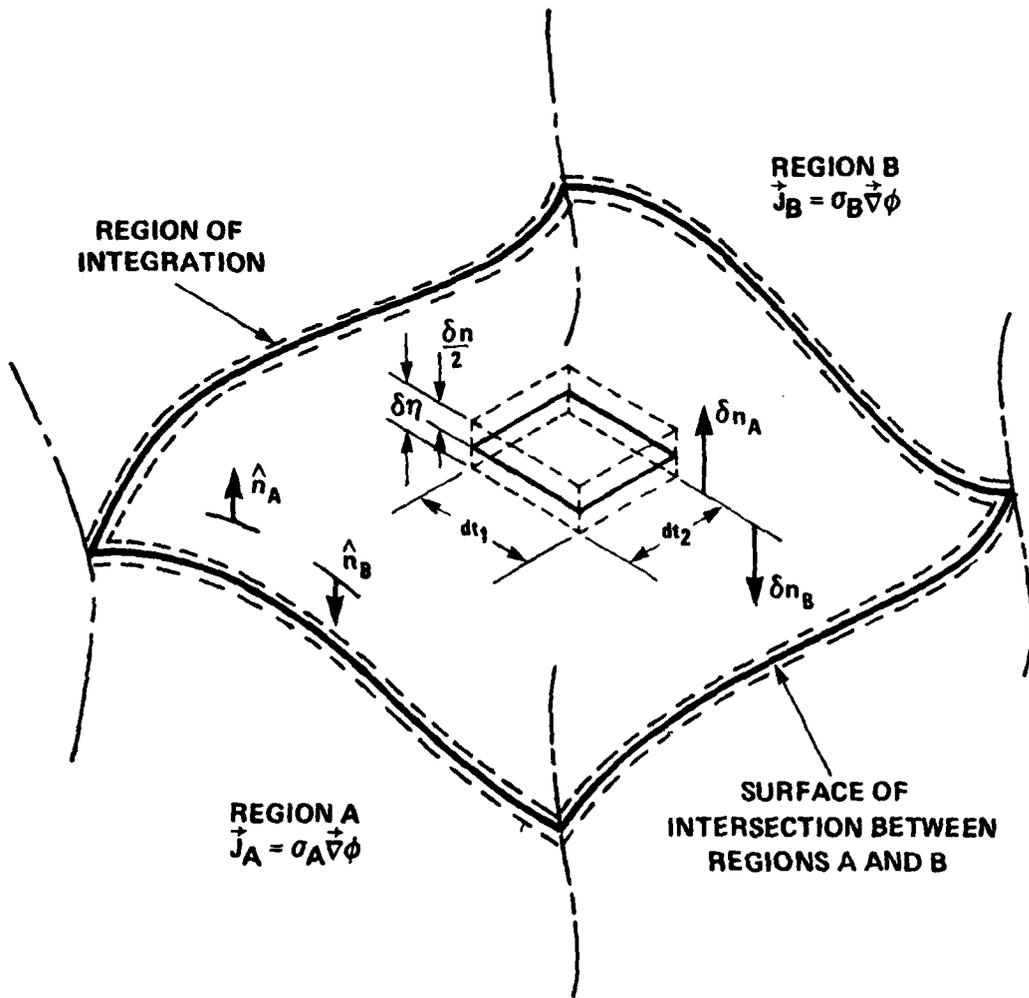
Figure 8. Surface Between Two Regions of Differing Conductivity
