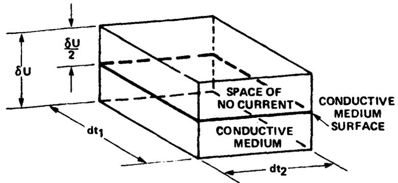
Figure 7. Elemental Volume of Integration on the Surface Region of a Volume
