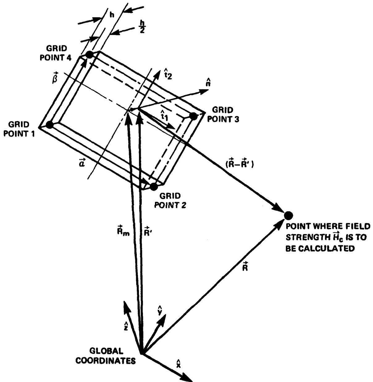
Figure 4. Coordinate Systems for Integrating Over the Region of Plates
