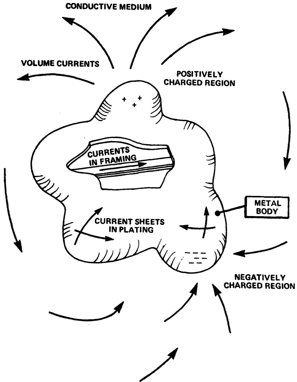
Figure 1. Problem of Internal and External Currents
