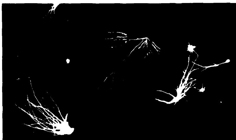
Fig. 5 - Surface streamer produced by charging the fuselage.
