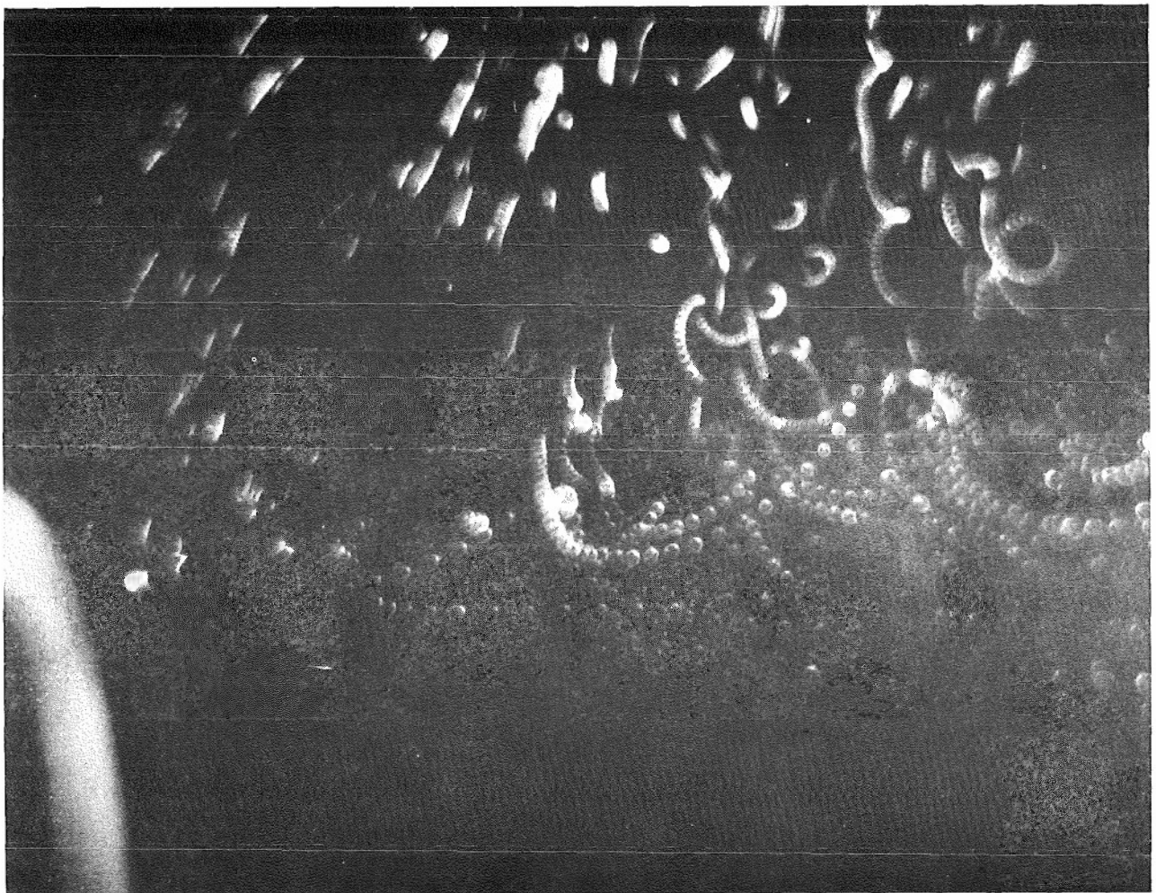
Fig. 17 - Set-up of the rotating laser beam and example of trajectories in a mixing layer (SCHON, DANIEL, MELINAND, REY & CHARNAY 1979)
