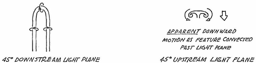
FIGURE 9 VIEWS SEEN BY CAMERA AS FEATURE CONVECTED PAST LIGHT PLANES
