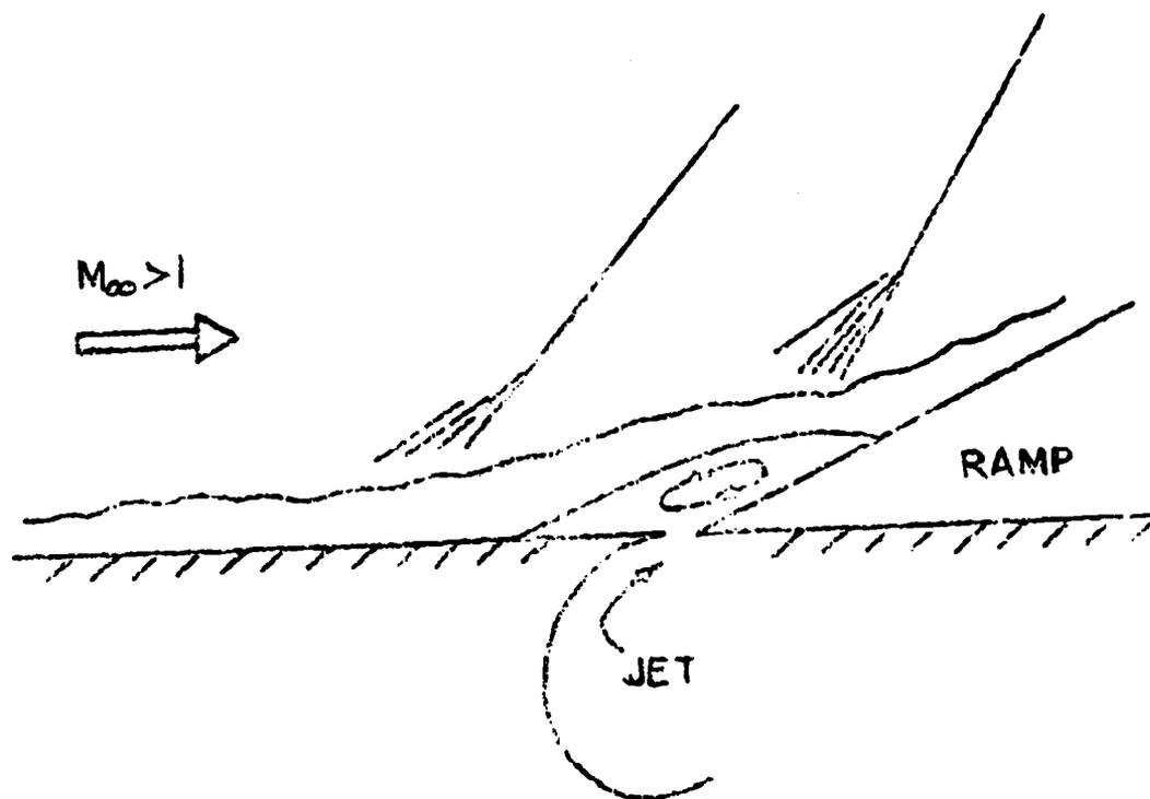
FIG. 5. PROPOSED INJECTION CONFIGURATION
