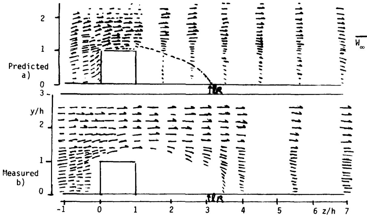
Fig. 7 Prediction of the velocity field in the longitudinal symmetry plane of a flow past a surface-mounted cube, from Vasilic-Melling (8)
