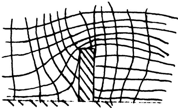
Fig. 13 Illustration of a flow-oriented grid arrangement.
