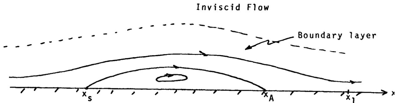
Figure 1. Schematic sketch of a small separation bubble.
