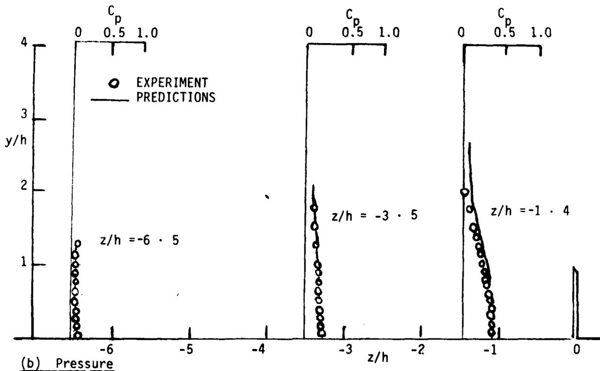
Fig. 5 Comparisons measured and predicted profiles upstream velocity and pressure correspond to Fig. 4.
