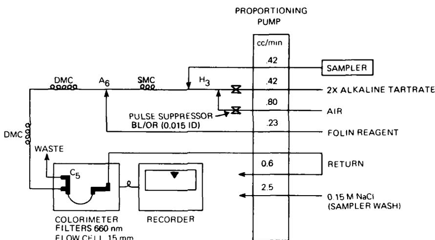
Figure 1. Flow manifold for the automated Lowry assay. Assay uses components of the Technicon AutoAnalyzer I system. The sampling rate is 50/hour with a sample-to-wash ratio of 2:1. All glass connections were used after connector H3. Both pulse suppressors were 0.005 inch inner diameter.
