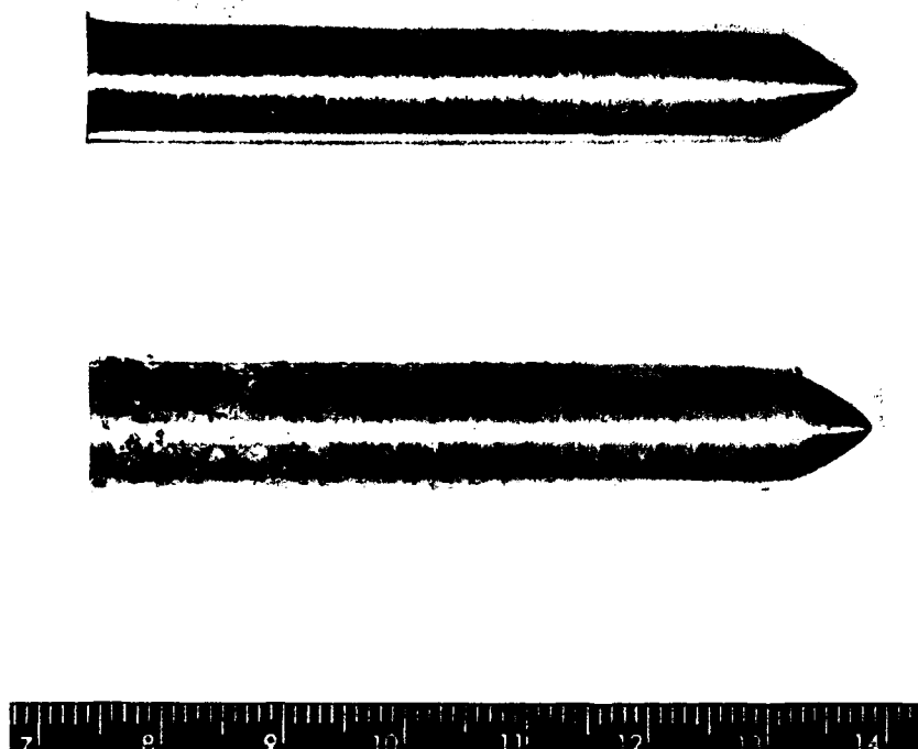
FIGURE 18. PHOTOGRAPH OF POLISHED STEEL SPECIMENS FROM NACE PIPELINE CORROSION TEST COMPARING BASE FUEL SPECIMEN (LEFT) WITH FRF SPECIMEN (RIGHT)
