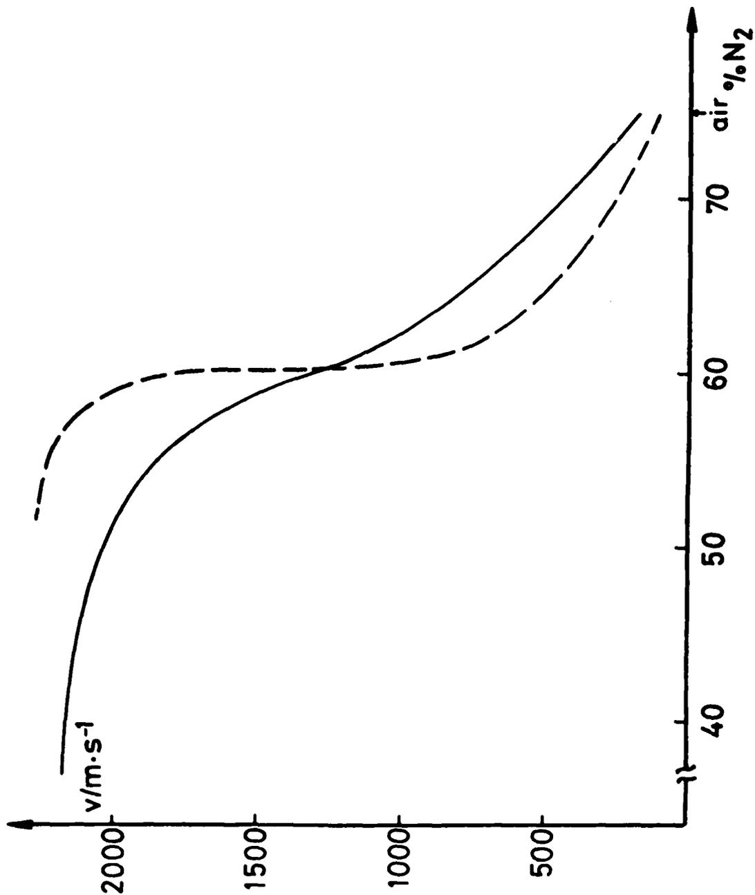
Fig.5 Mean flame velocities in the downstream section
