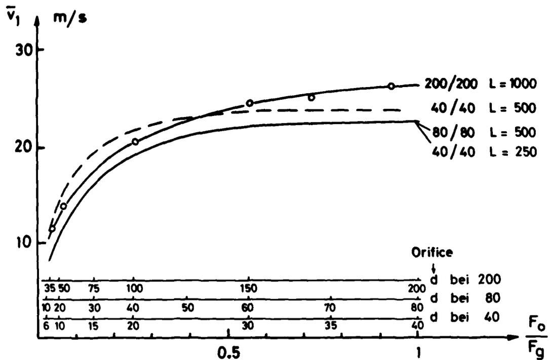
Fig. II.2 Mean velocity of flames in driver section
