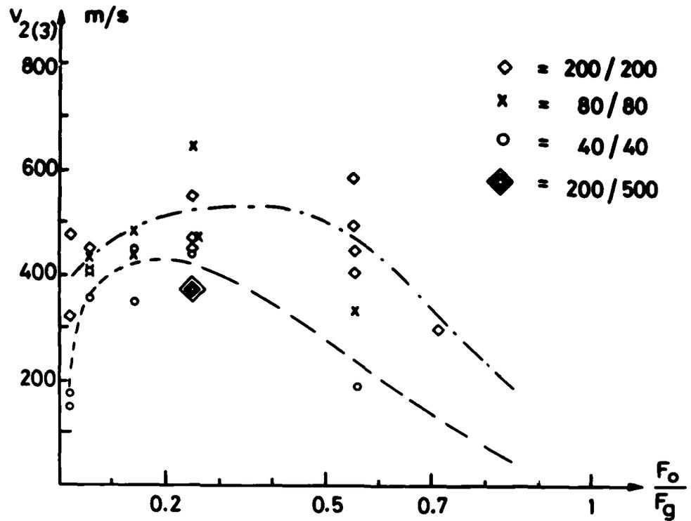
Fig. II. 6 Flame velocity in downstream section (m/sec)
