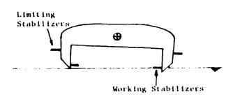
Hydrodynamic stabilizers can be used to retain adequate roll stability and to limit sidehuli immersion depths at high speeds.
