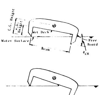
With appropriately small cushion height/beam and C.G. height/beam ratios, the roll angle at which the wet deck contacts the water surface will be relatively small and at this point the moment arm of the hydrostatic restoring force will still be reasonably large.
