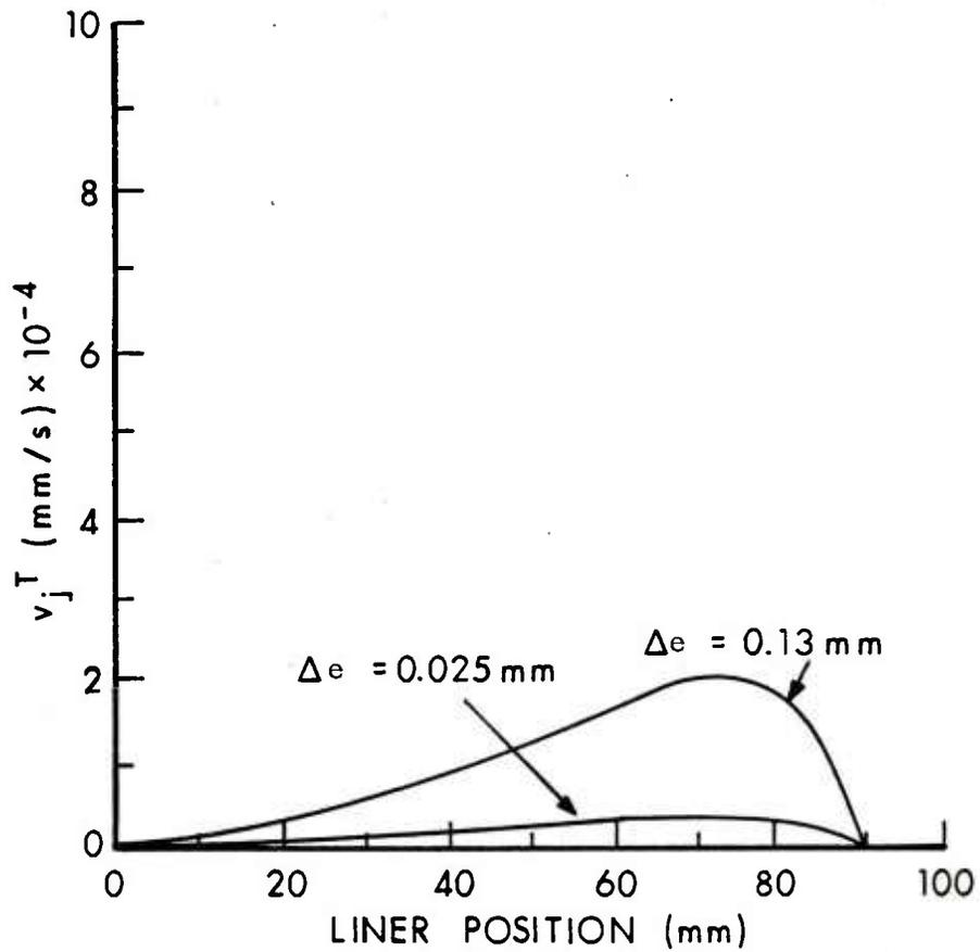
Figure 7. Transverse Jet Velocity vs. Liner Position for Different Explosive Centering Asymmetries Around Liner
