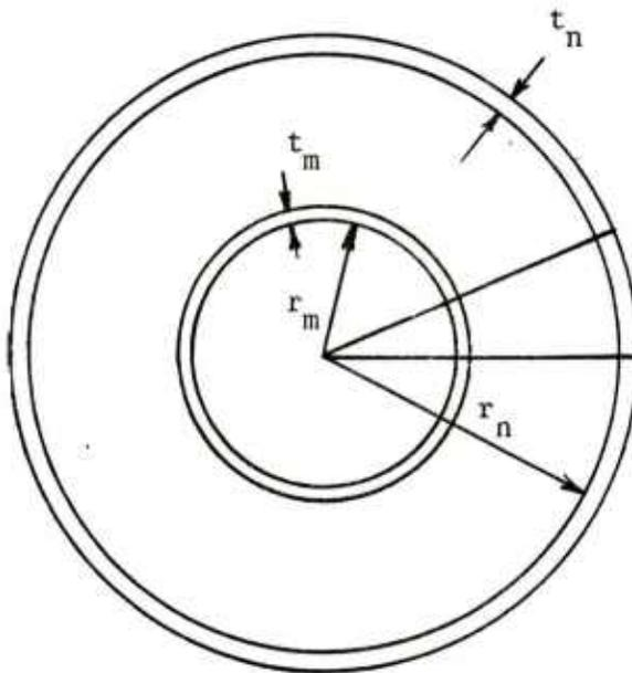
Figure 11. Charge Geometry Used to Estimate Relative Importance of Gurney Estimates
