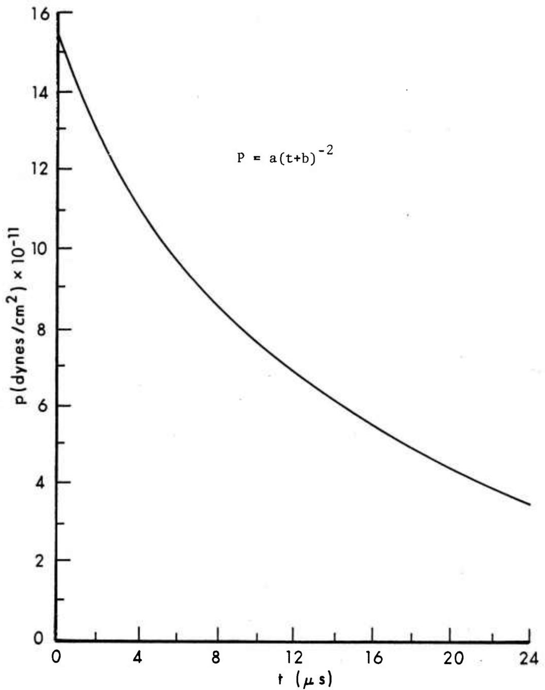
Figure 3. Pressure Function Assumed to Drive Liner
