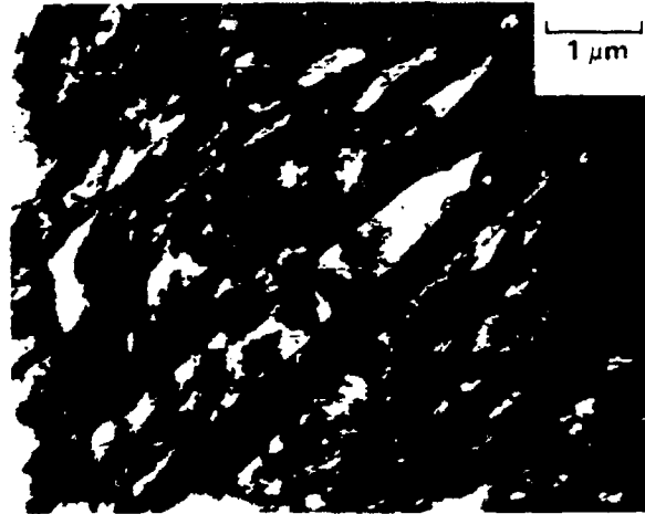
TRANSVERSE SECTION ROLLED 90%
