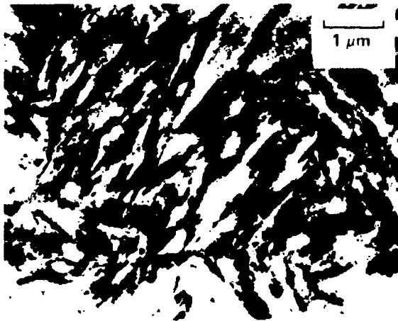
LONGITUDINAL SECTION ROLLED 60%
