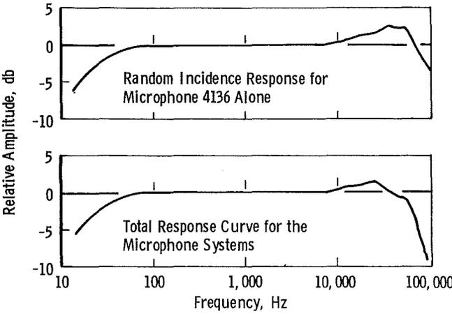
Figure 6. Typical measured frequency response for installed microphones.
