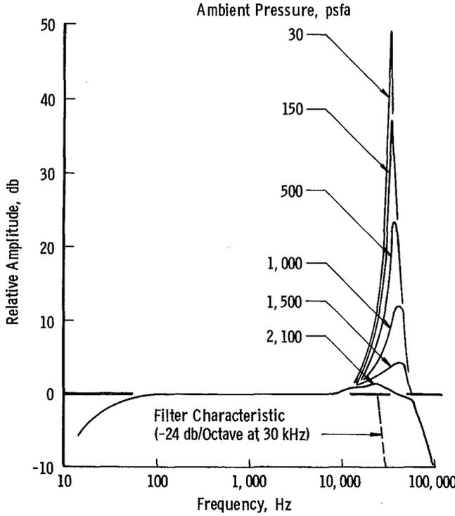
Figure 7. Influence of absolute pressure level on microphone frequency response.
