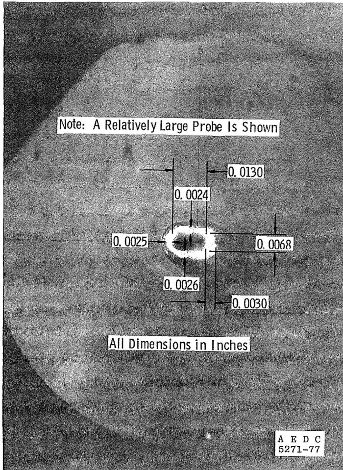
c. Microscopic photograph of a typical probe opening
