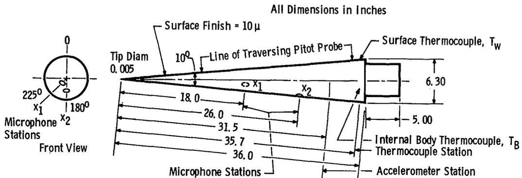
Figure 1. AEDC 10-deg transition cone model.
