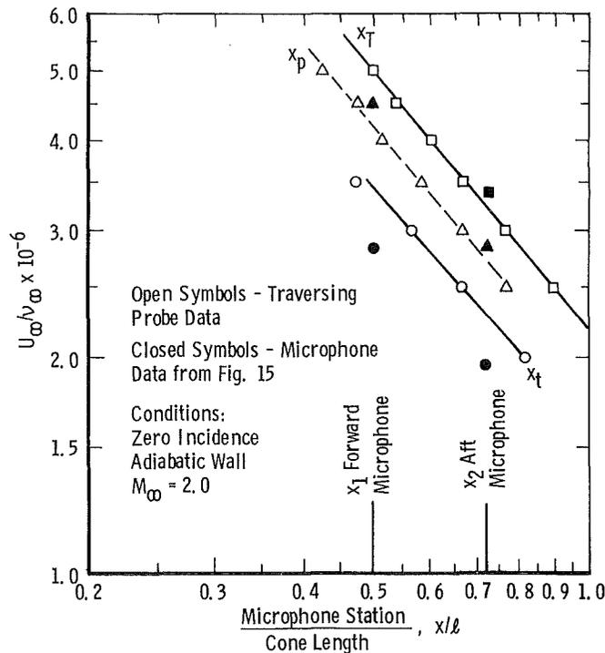
Figure 14. Comparison of transition location between pitot pressure probe and microphone data.
