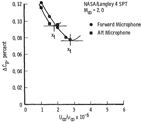
b. Expanded scale of the laminar condition
