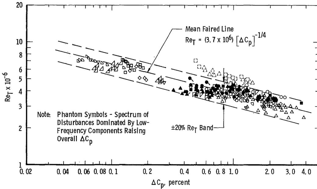
Figure 20. Overall correlation of end-of-transition location ( $Re_T$ ) with rms noise level ( $\Delta C_p$ ).
