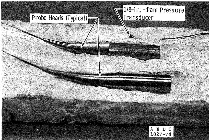
**b. Photograph of probes and transducer**
