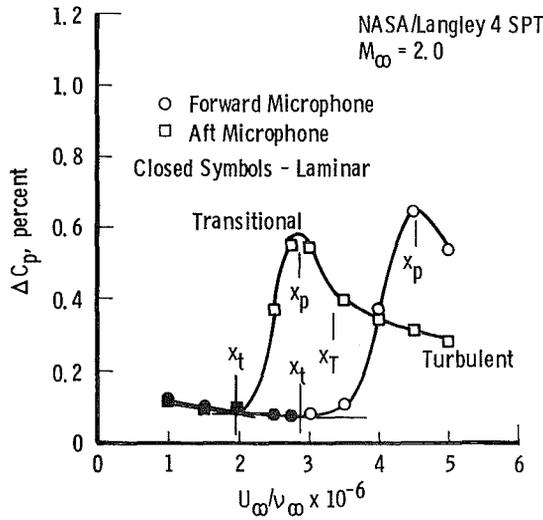
a. Laminar, transitional, turbulent conditions
