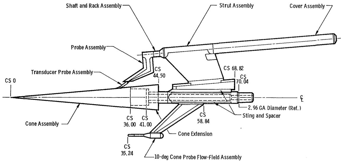
b. Configuration with flow angle probe and cone extension
