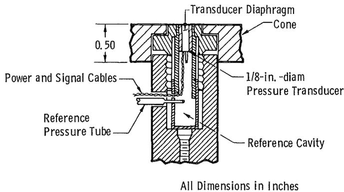
b. Transducer installation details at  $X_1 = 18$  in.
