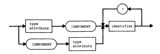
If an identifier is declared to be a component according to component declaration 1, and the component field is a proper part of a word, then this identifier must appear in all three lists; the component list, the offset list, and the field list. For whole word and double word components the field definition may be omitted.
