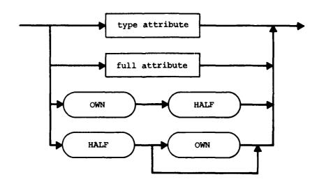
Type Declarations. Type declarations specify variables to be INTEGER, DOUBLE, REAL, or POINTER. The variable specified by an identifier can only assume values of the declared type by assignment or preset declaration. If the variable receives an assigned value, automatic type conversion will have occurred.
