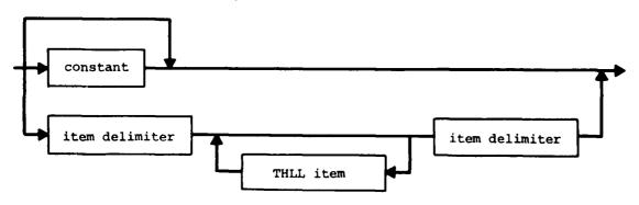
A THLL item is a constant, an identifier, an operator or a delimiter. An item delimiter is a THLL item that is not a constant and not the semi-colon. The right-end item delimiter is the first occurrence of the source THLL item that functions as the left-end item delimiter.
