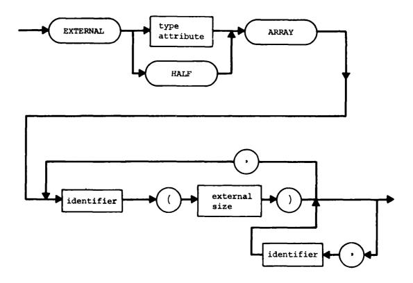
Stack Declarations. Stack declarations provide information concerning the type, name, and size of a stack, as well as indicating its allocation mode.
