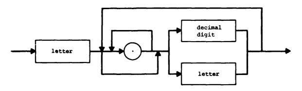
component id, array id, stack id, device id, procedure id,
