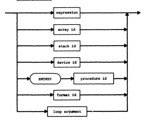
Although it is syntactically correct to use a loop argument anywhere in a function parameter list, it is semantically correct to use a loop argument only after the fifth parameter in a READ/WRITE statement.
