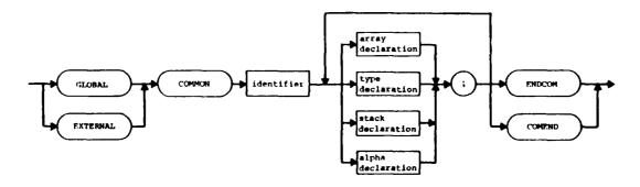
Preset Declaration. The preset declaration is used to initialize OWN variables at compile time. Simple and subscripted variables may be preset. Subscripted variables using a stack identifier cannot be preset.
