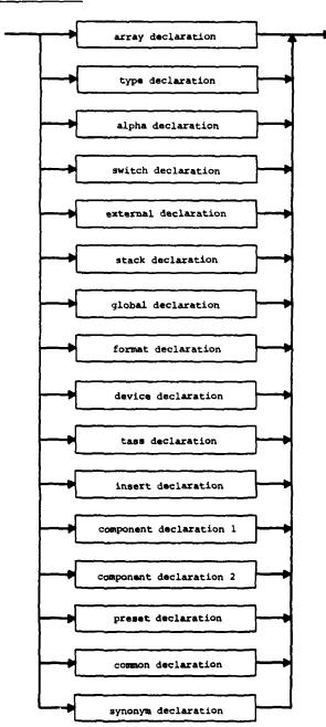
Array Declarations. Array declarations provide information concerning the type, name, and size of an array, as well as indicating its allocation mode. Array subscripting starts with zero. For example, an array named TAB which is to be one-dimensional and contain 10 elements would be indicated by TAB(9). Arrays may be one-, two-, or three-dimensional with the maximum size of each dimension being specified by an integer constant in the declaration statement.
