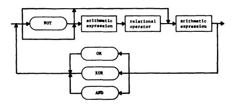
Arithmetic Expression. An arithmetic expression is a primary or basic element or a combination of basic elements connected by arithmetic or bit operators.
