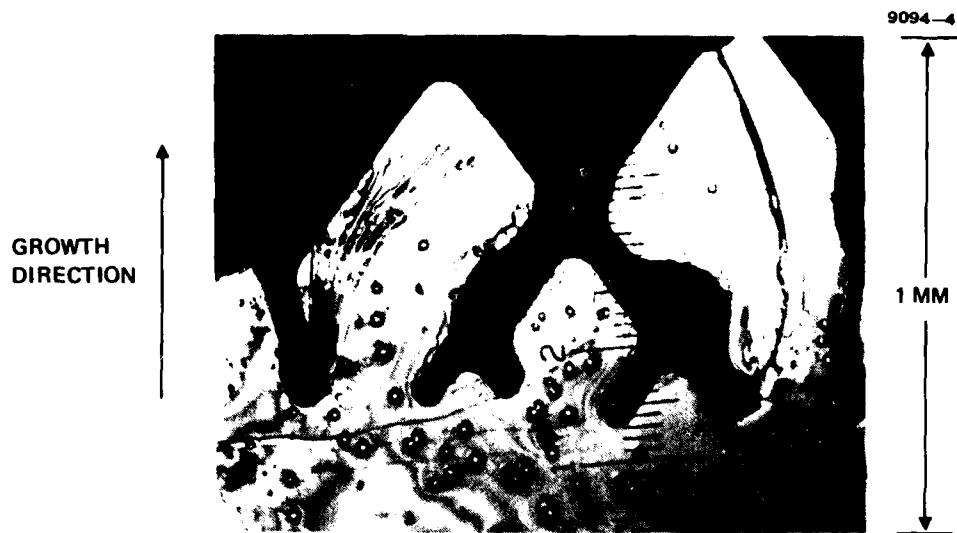
Figure 7. Micrograph of crystal cross section showing interface breakdown.
