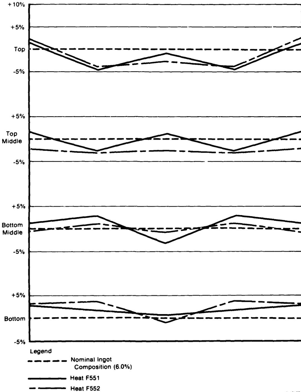
Figure 144. Variation in Aluminum Content vs Ingot Position
