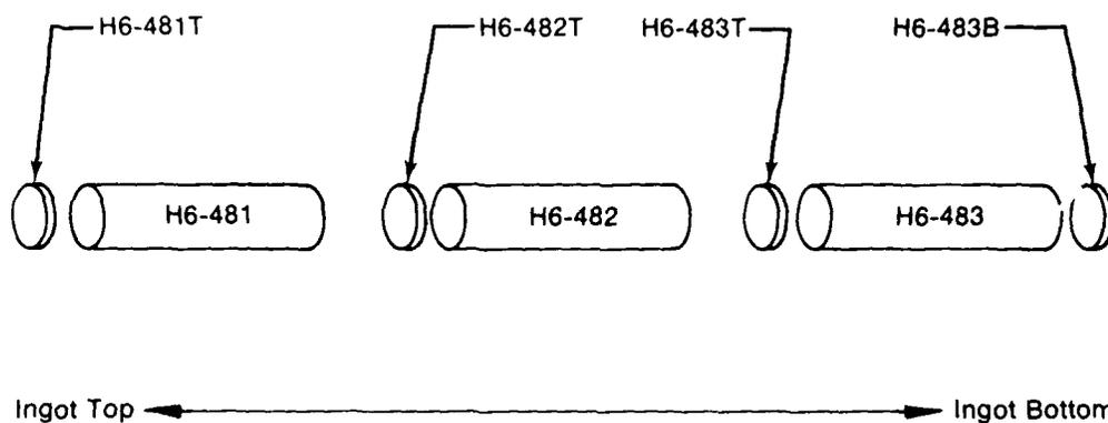
Figure 125. Billet Cut-Up of Master Heat BBA. (Teledyne — ALLVAC F552, Lot B Chips)
