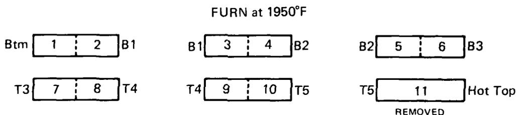
3 3/4 in. RCS      Cut on Dotted Lines and Rolled to 2 1/2 in. RCS
