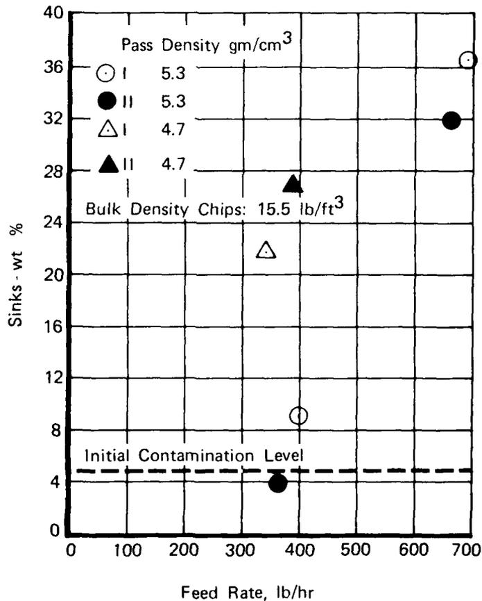
Figure 15. AVCO Ferrofluid Separation Test Series D. Weight-Percent Sinks vs Feed Rate of Contaminated Titanium Chips (Lot 04) at Various Feed Rates and Operating Densities
