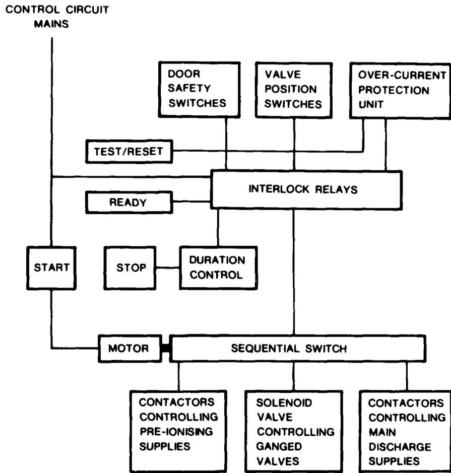
FIG. 9 - SCHEMATIC DIAGRAM OF CONTROL SEQUENCE.
