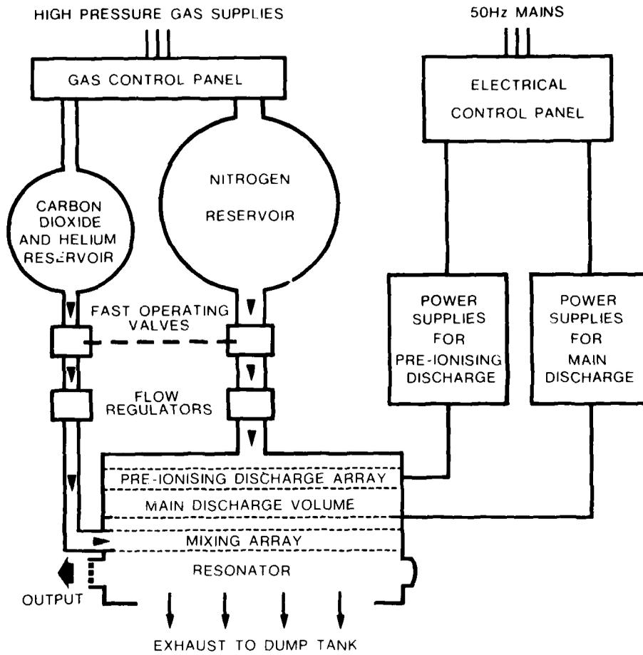
FIG. 2 - SCHEMATIC OF LASER AND ANCILLARY SYSTEMS.
