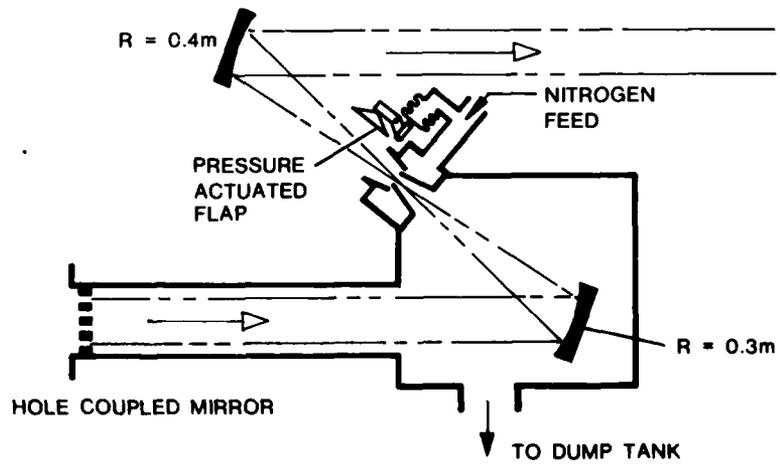
FIG. 6 - SYSTEM USED TO COUPLE POWER FROM THE LASER.
