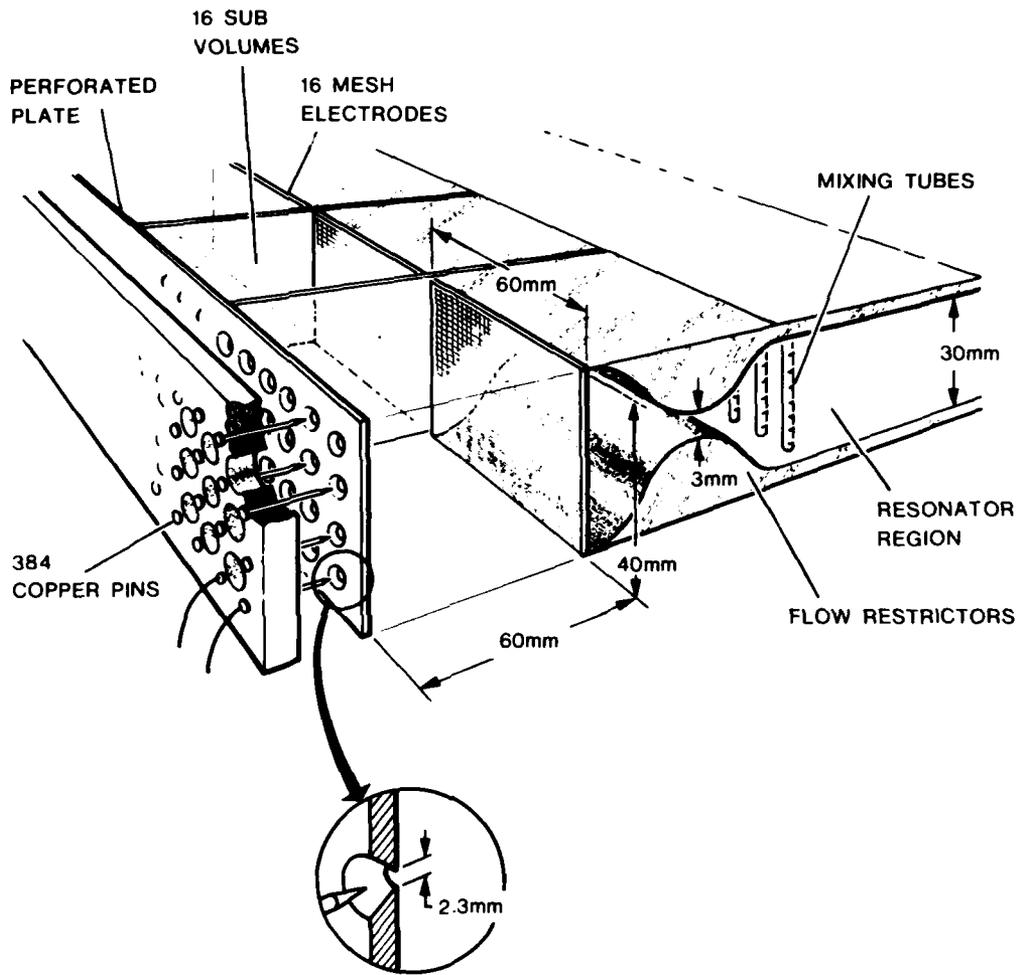
FIG. 4 - ARRANGEMENT OF ELECTRODES AND RELEVANT DIMENSIONS.
