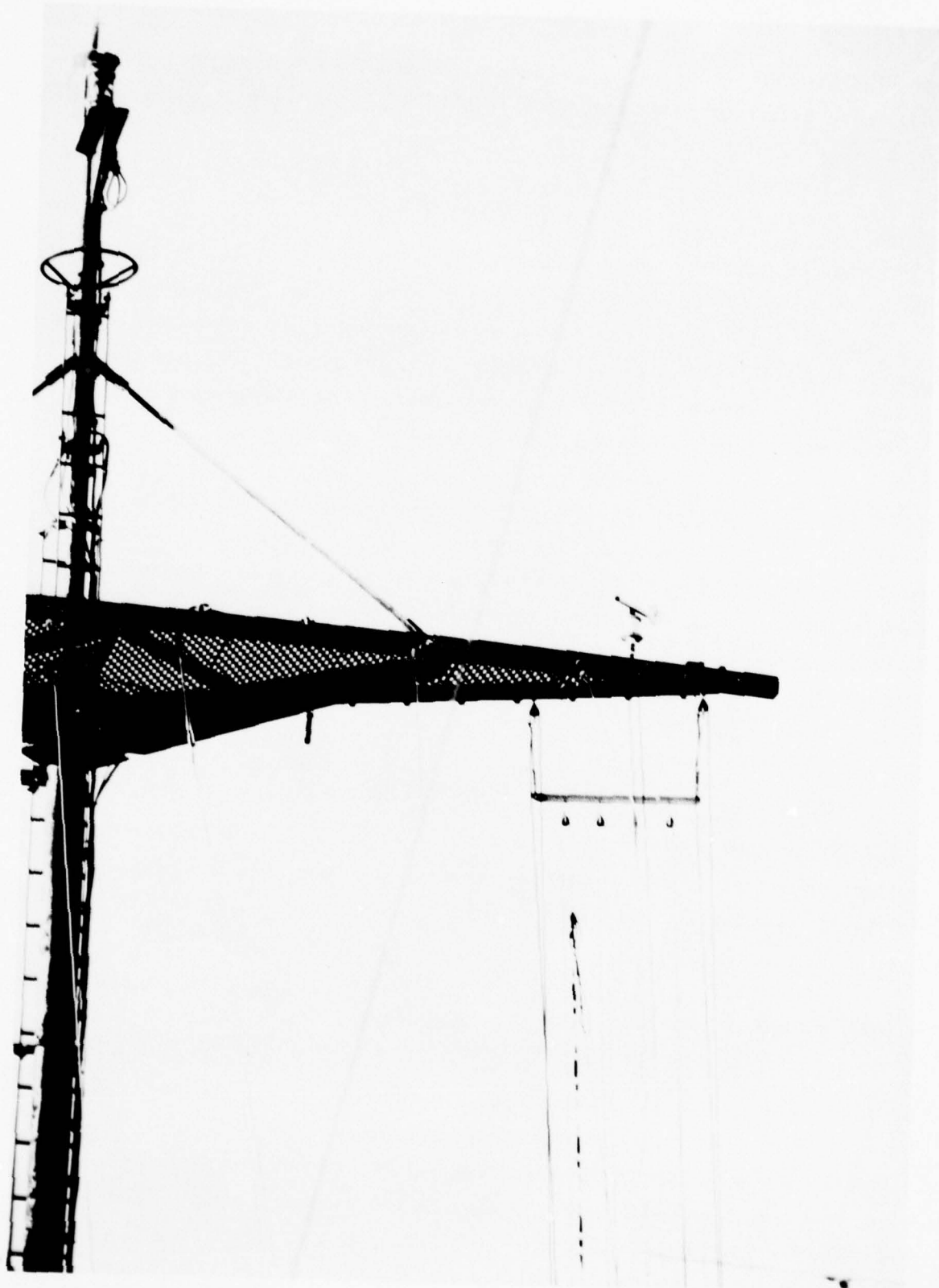
Figure II-4: One of two anemometers mounted on after mast catwalk.
