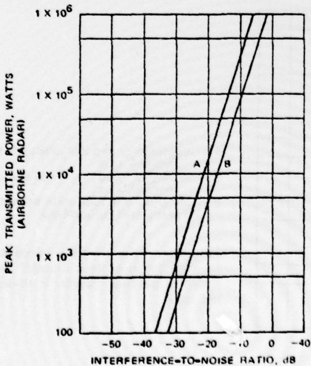
A - RECEIVED THROUGH SPACE STATION MAIN BEAM. Satellite at 10-deg elevation angle
