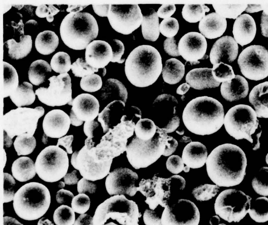
(c) SEM photograph of MAR-M200 RSR powder particles at 100X.
