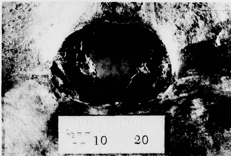
Figure 5. Exit Hole in Drilled Target.
