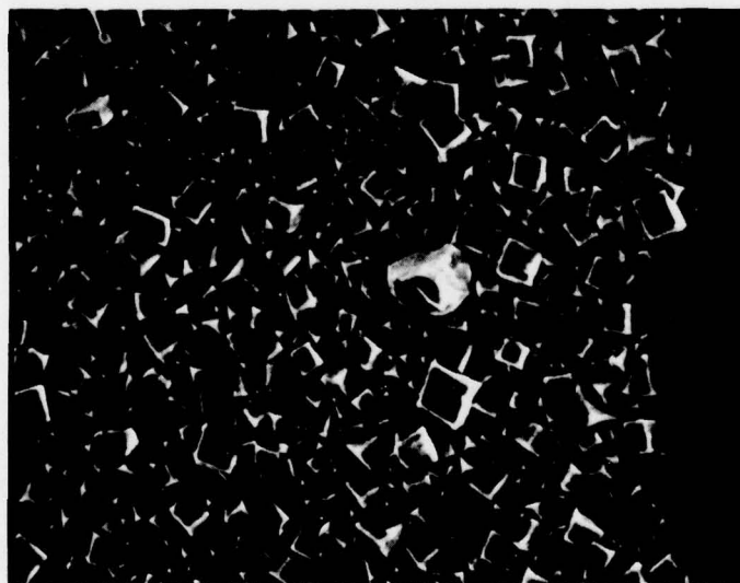
Figure 28 - SEM of Lithium Surface Exposed to 1.8 M \text{LiAlCl}_4/\text{SOCl}_2 For 17 Days at 55°C; X300.
