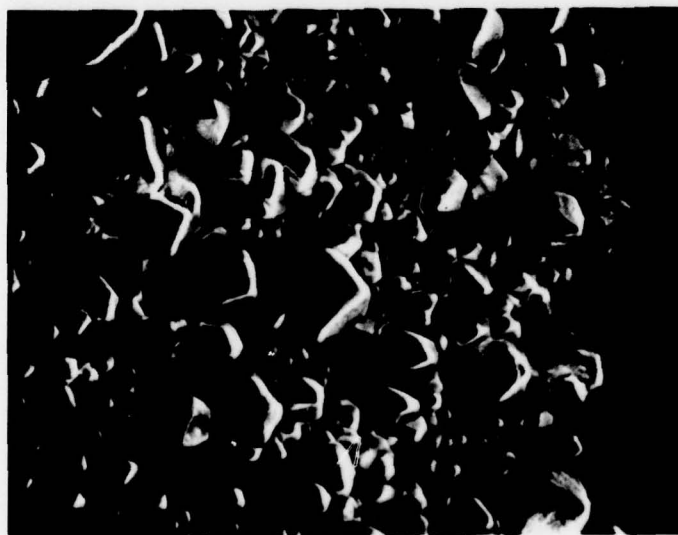
Figure 30. SEM of Lithium Surface Exposed to 1.8 M \text{LiAlCl}_4/\text{SOCl}_2 for 17 Days at 72°C; X300.
