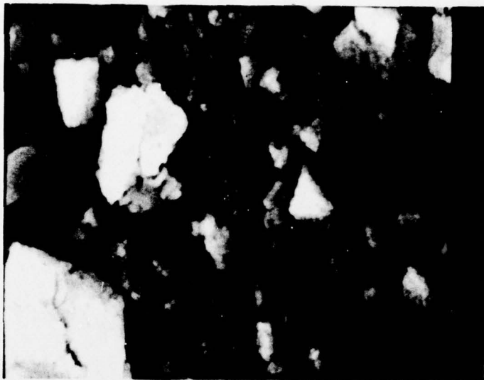
Figure 14. SEM of Lithium Surface Exposed to \text{SOCl}_2 for 80 Days at 55^\circ\text{C} . X3,000
