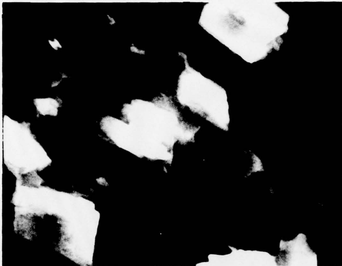
Figure 20. SEM of Lithium Surface Exposed to \text{SOCl}_2 for 83 Days at 72^\circ\text{C} , X3000.
