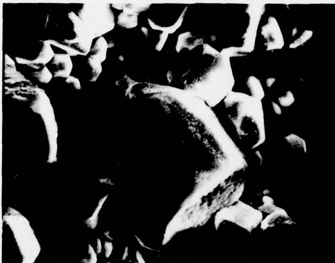
Figure 31. SEM of Lithium Surface Exposed to 1.8 M LiAlCl 4 /SOCl 2 For 17 Days at 72°C; X1000.
