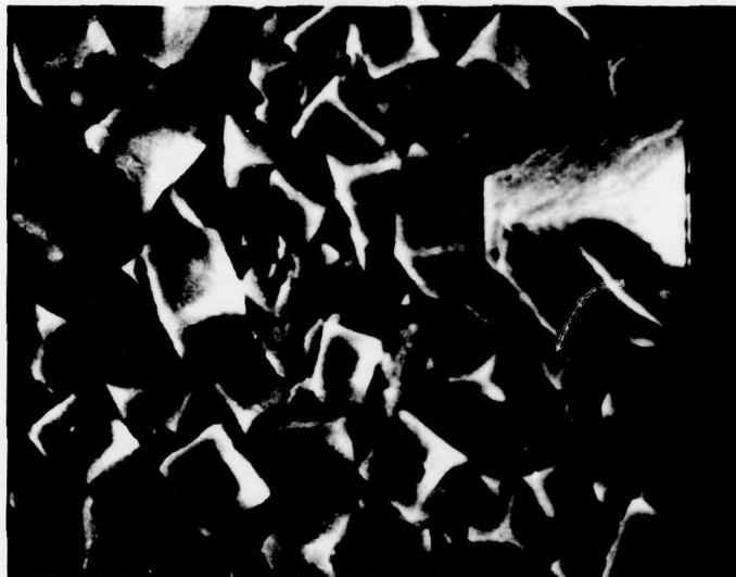
Figure 29. SEM of Lithium Surface Exposed to 1.8 M \text{LiAlCl}_4/\text{SOCl}_2 for 17 Days at 55°C; X1000.
