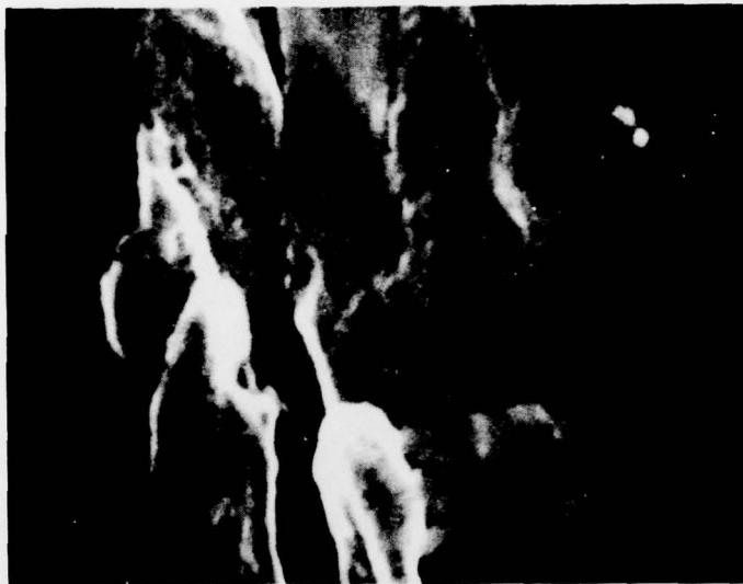
Figure 50. SEM of Lithium Surface Exposed to 0.25 M \text{Li}_2\text{B}_{10}\text{Cl}_{10}/\text{SOCl}_2 for 19 Days at Room Temperature; X10,000.
