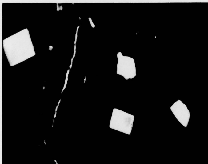
Figure 47. SEM of Lithium Surface Exposed to 0.25 M \text{Li}_2\text{B}_{10}\text{Cl}_{10}/\text{SOCl}_2 for 19 Days at Room Temperature; X10,000.
