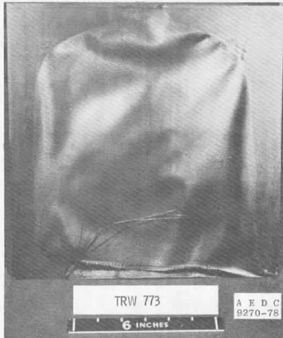
a. t \approx 0.096 in., total exposure time = 32.8 sec
