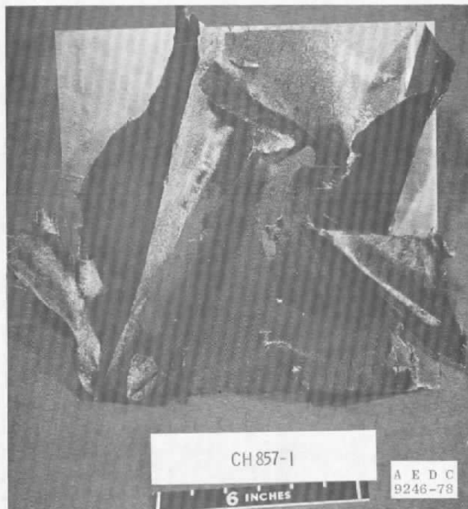
d. t \approx 0.112 in., total exposure time = 33.3 sec Figure 15. Continued.
