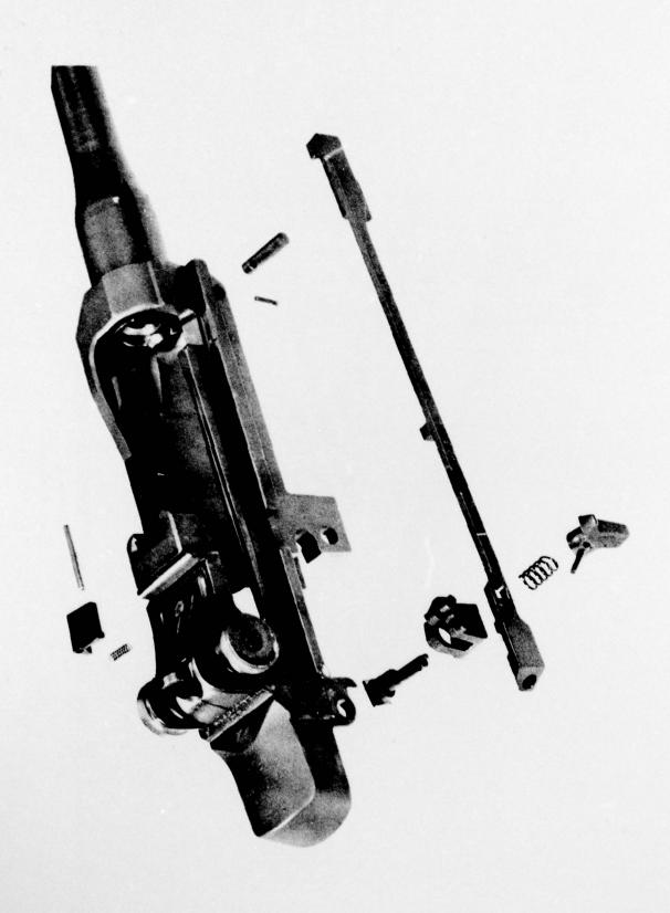
13 June 1955 Disassembled Connector Assembly, Connector Lock, Selector and Bolt Lock SPRINGFIELD ARMORY - ORDNANCE CORPS RIFLE, CALIBER. 30, T44E4 10915-8A
