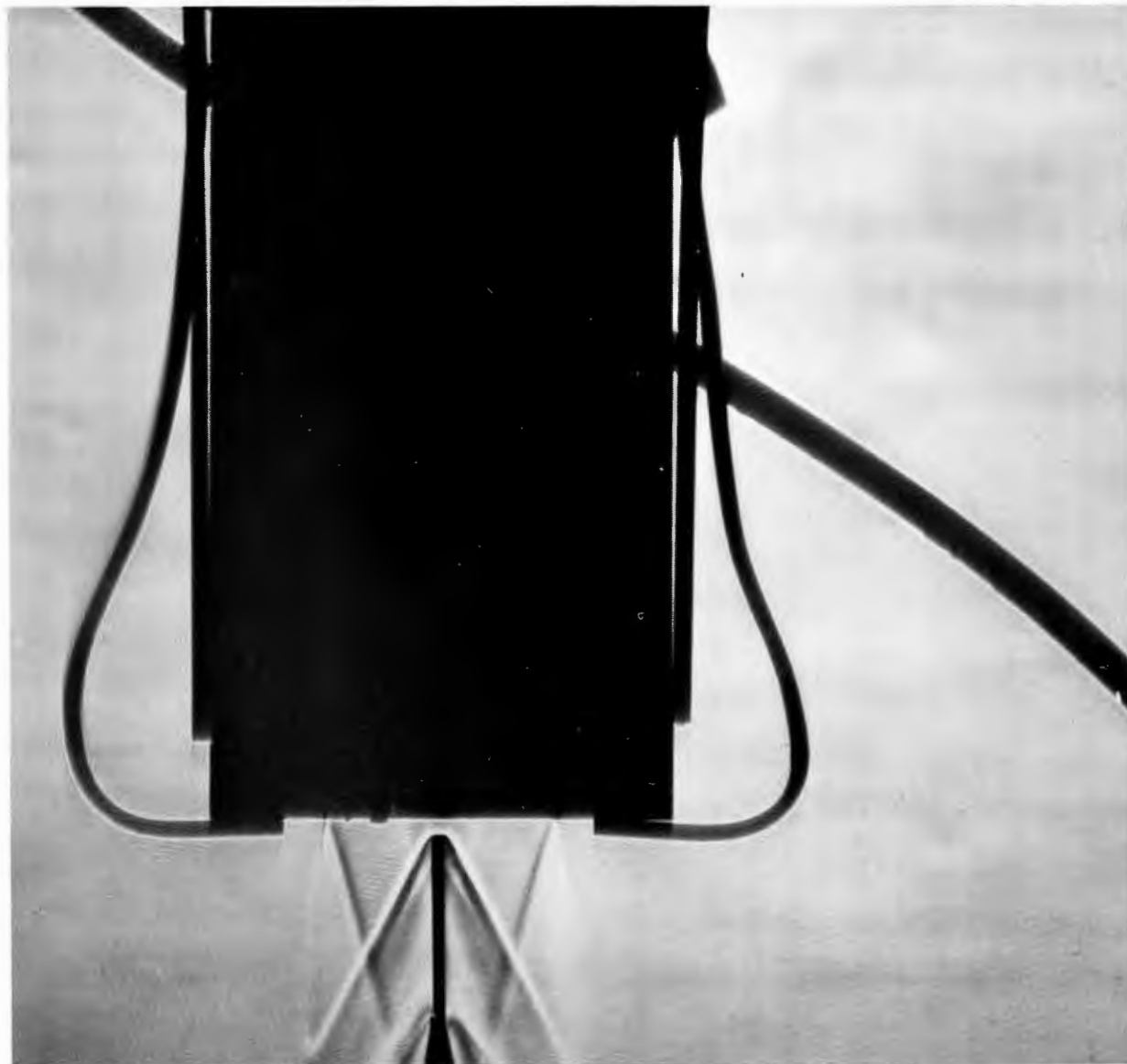
FIGURE 30 SCHLIEREN PHOTOGRAPH OF PITOT SURVEY: NOZZLE NO. 2 (RUN 6)
