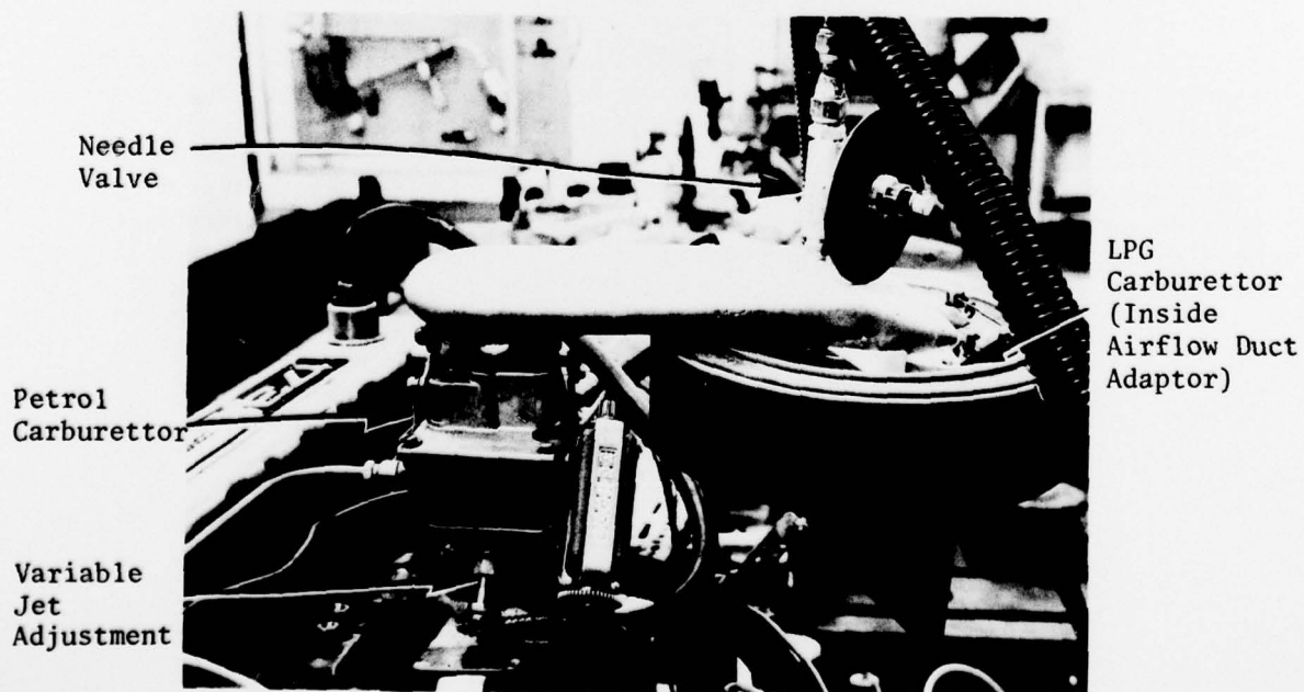
FIG 2 - VARIABLE JET ADJUSTMENT (PETROL) AND SUBSIDIARY NEEDLE VALVE (LPG)
