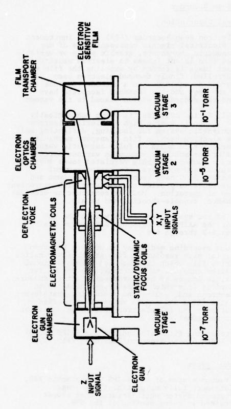
Figure 6-1. Schematic Layout of Cartographic EBR
