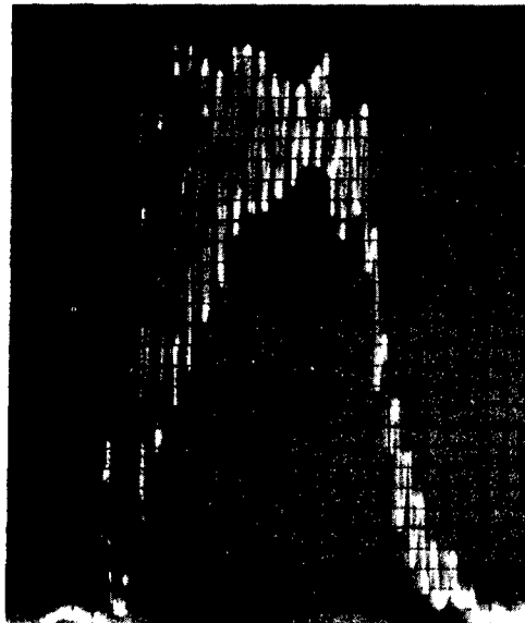
Secondary High-frequency Oscillations Observed During Fatigue Test Work on Tubing
