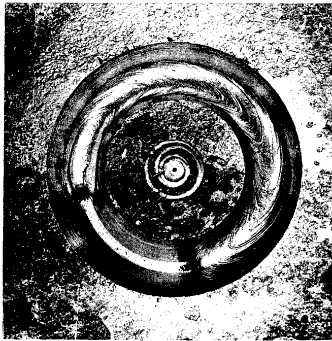
B. Weld-Metal Composition 0.25% C, 2.56% Mn, 0.05% Si
