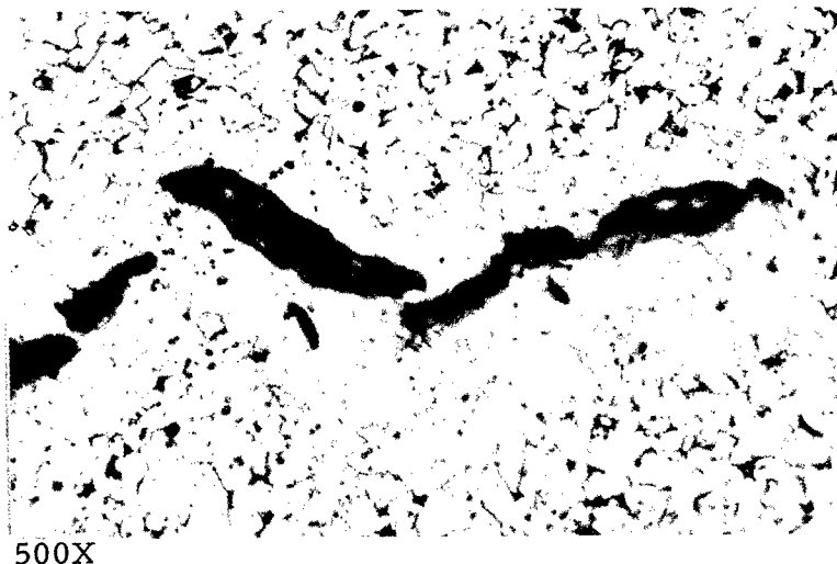
FIGURE 28. PHOTOMICROGRAPH OF FISSURE IN WELD METAL DEPOSITED WITH AWS CLASS E6011 ELECTRODES (H37)
