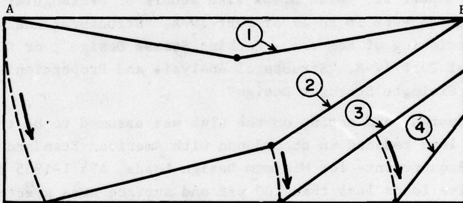
(b) Unsymmetric Collapse Mode for Simply-Supported Slab
