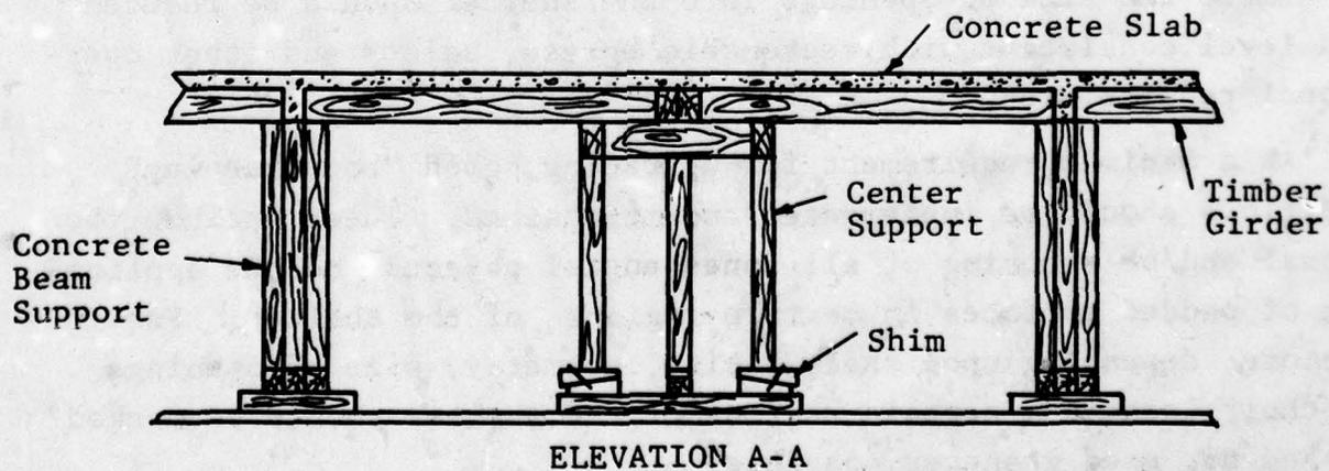
Figure 62. Two-Way Slab Upgrading System
