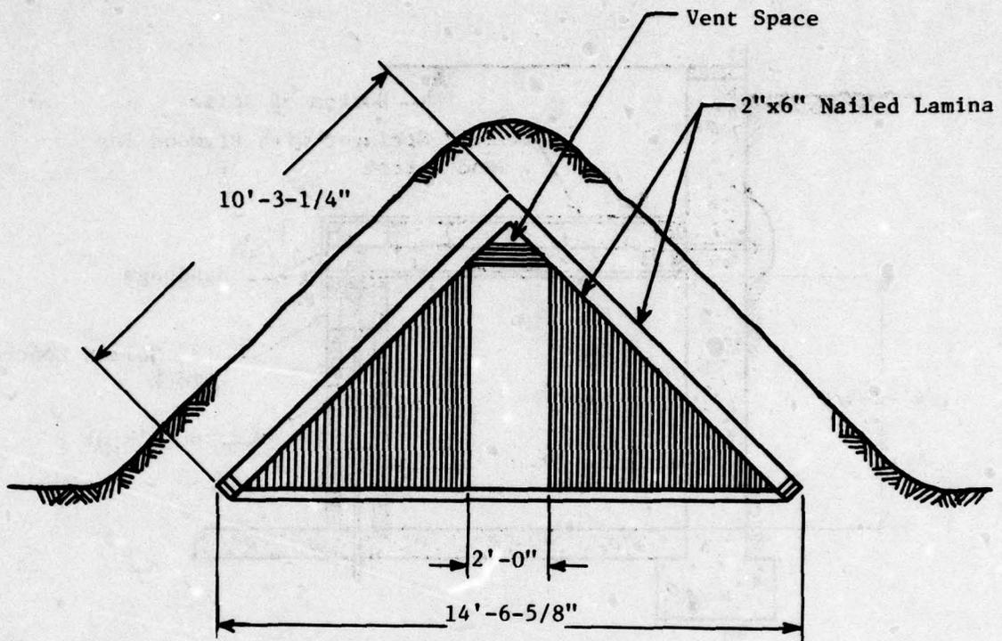
Figure 57. Aboveground A-Frame Shelter
