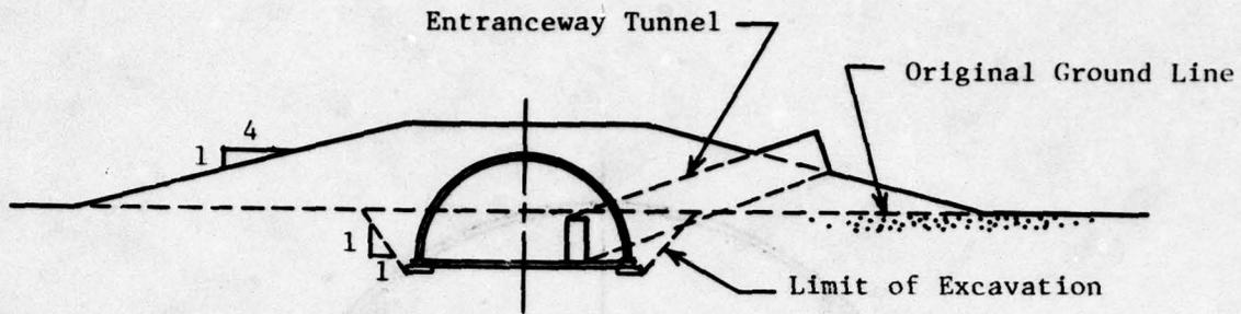
Figure 21. Arch Shelter Location Relative to Ground Surface
