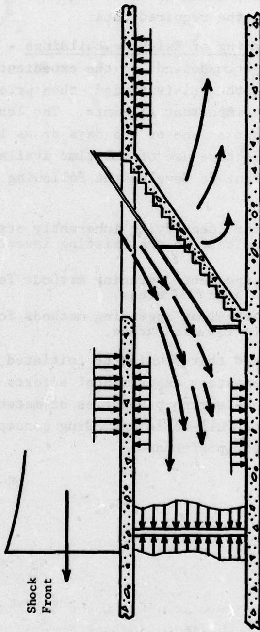
Figure 68. Blast Loading of Basement Areas
