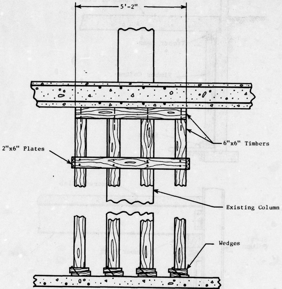
Figure 64. Concrete Column Upgrading
