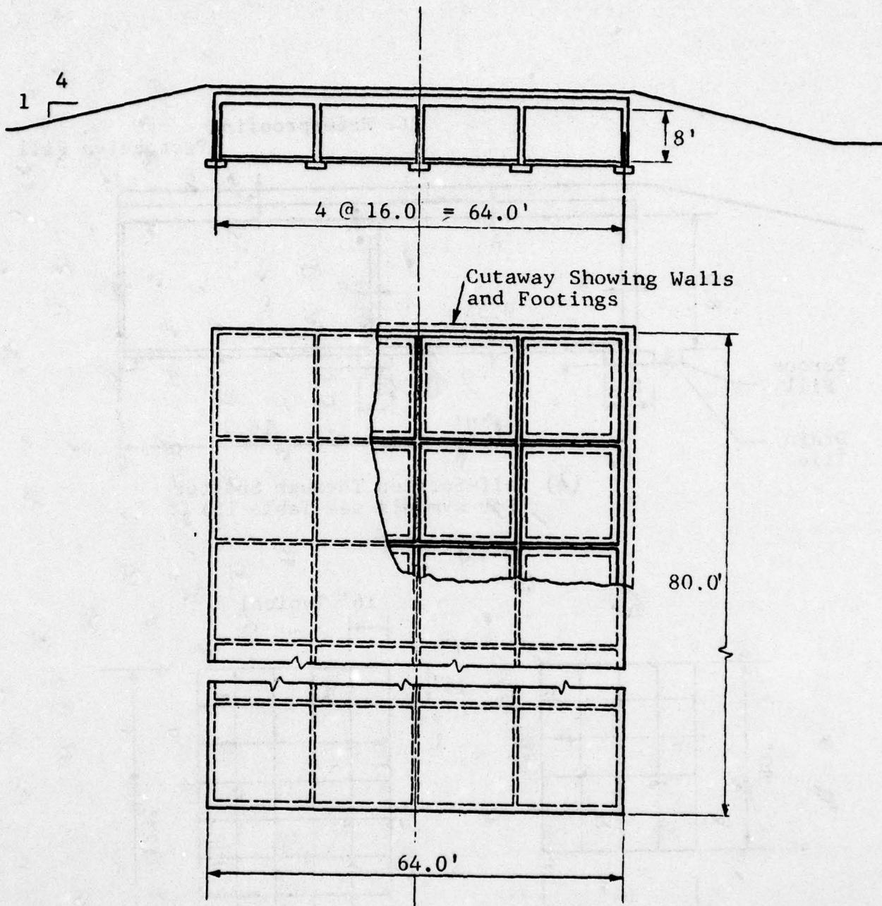
Figure 23. General Configuration of Basic 500-Man Rectangular R/C Shelter
