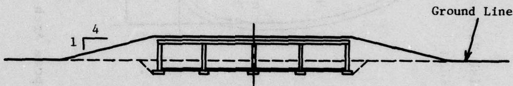
Figure 25. Rectangular Shelter Location Relative to Ground Surface
