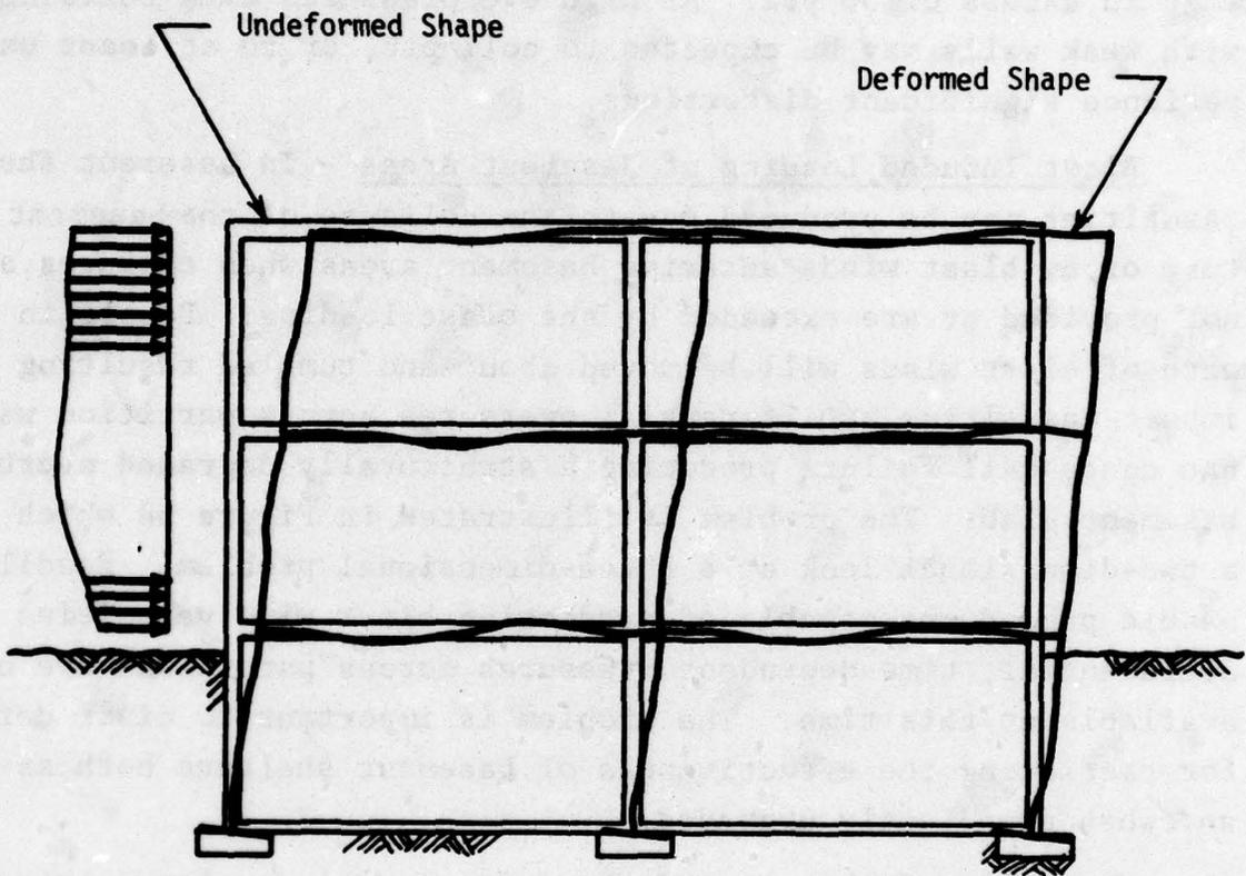
Figure 67. Building Frame Deformation Due to Lateral Load
