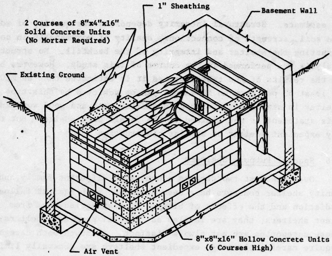
Figure 53. Concrete Block Shelter
