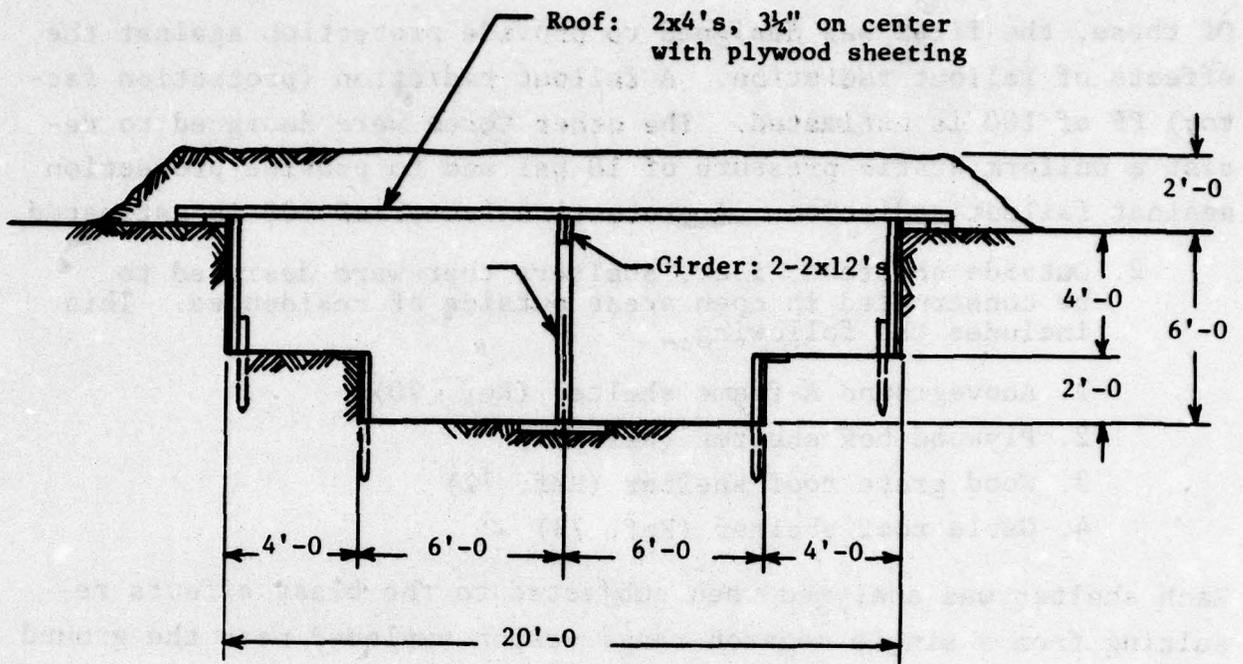
Figure 59. Wood Grate Roof Shelter
