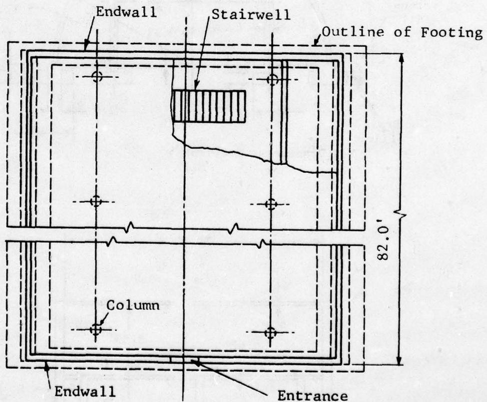
Figure 20. General Configuration of Basic 500-Man Arch Shelter
