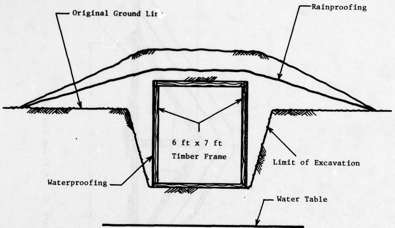
Figure 50. Timber Frame Trench Shelter
