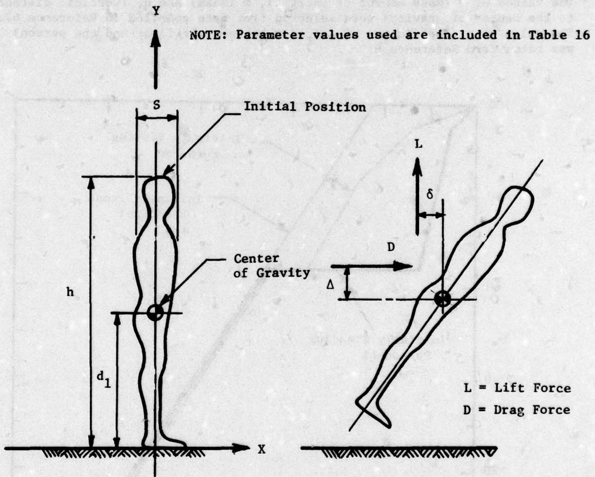
Figure 37. Tumbling Man Simulation Model (Standing Configuration)
