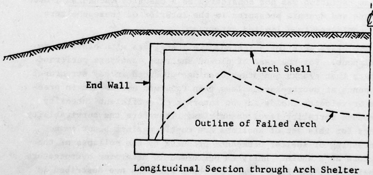
Figure 31. Definition of Arch Structure Failure
