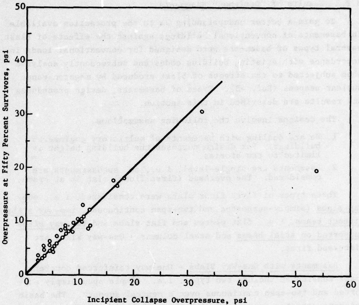
Figure 11. Comparison of Free Field Overpressure at Fifty Percent Survivors with Basement Overhead (First) Floor Strength
