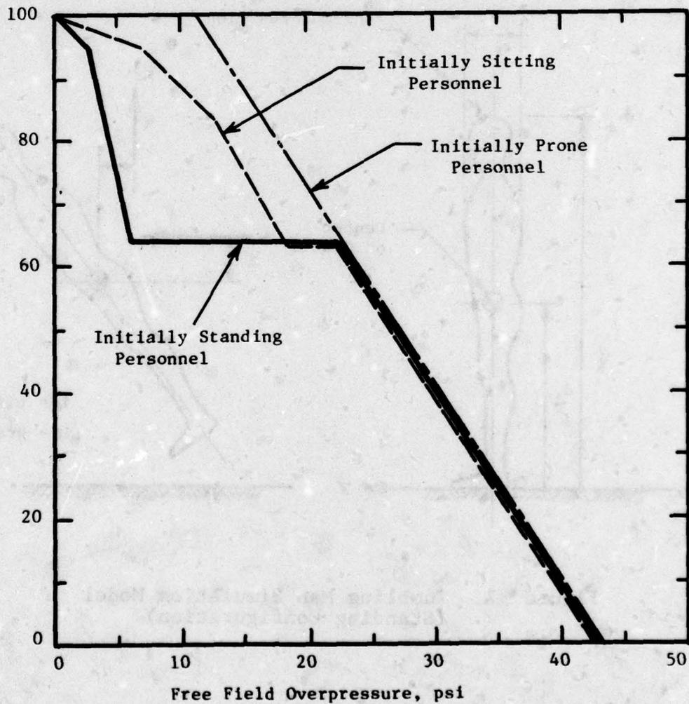
Figure 38. People Survivability Estimate for an Open Steel Arch Shelter (Fallout Radiation Design)
