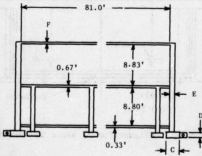
Figure 22. Basic Dimensions of Arch Shelter
