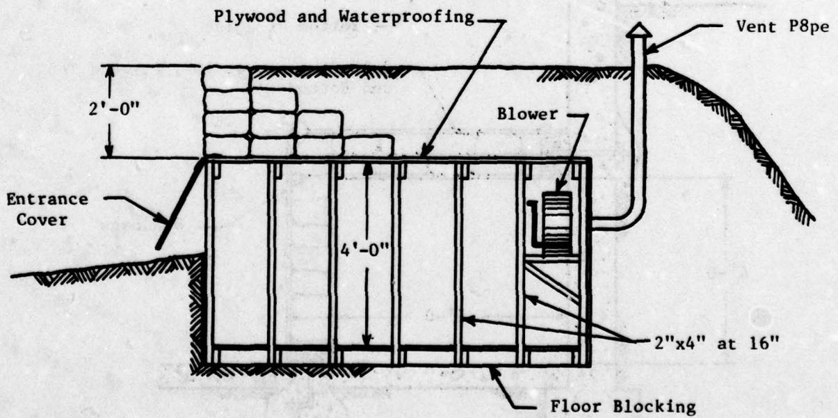
Figure 58. Plywood Box Shelter
