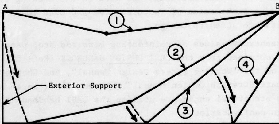
(c) Collapse Mode for Two-Span Continuous Slab
