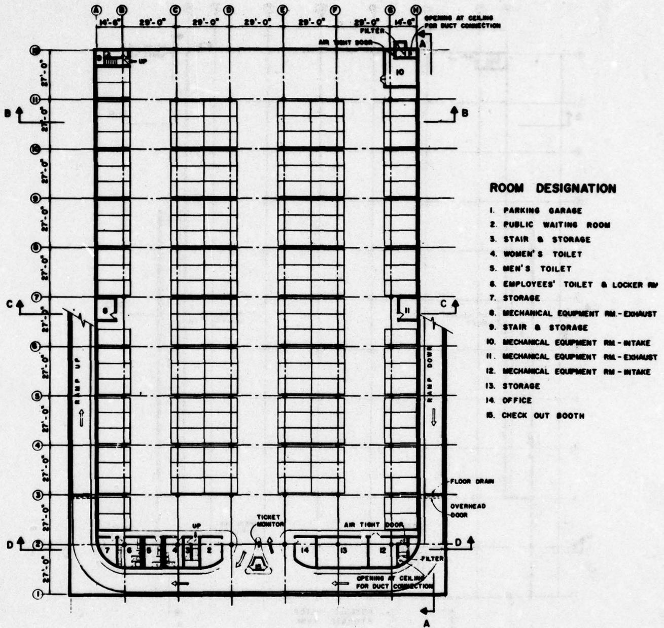
Figure 47. Parking Garage Shelter - Lower Level Plan
