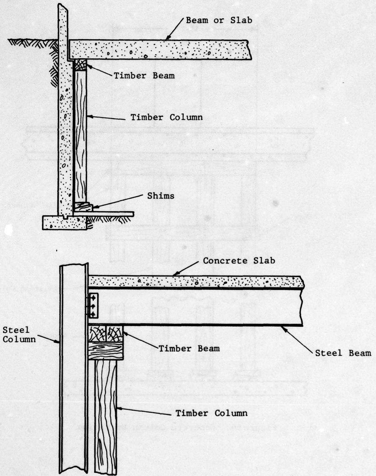
Figure 63. End Support Expedient Upgrading Concepts
