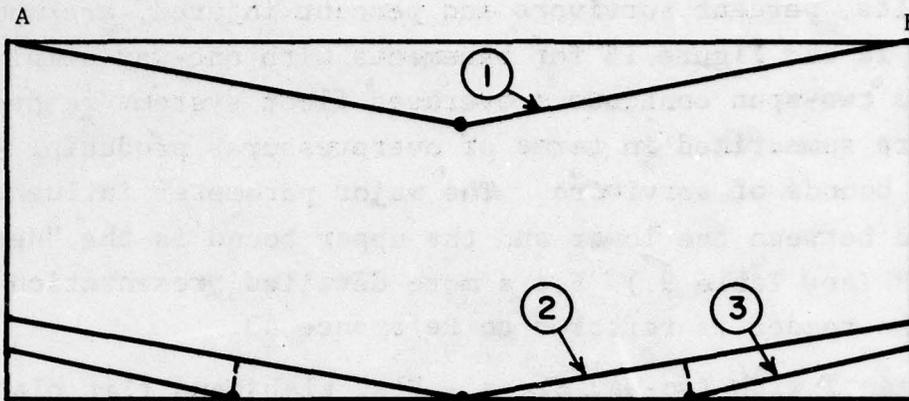
(a) Symmetric Collapse Mode for Simply-Supported Slab
