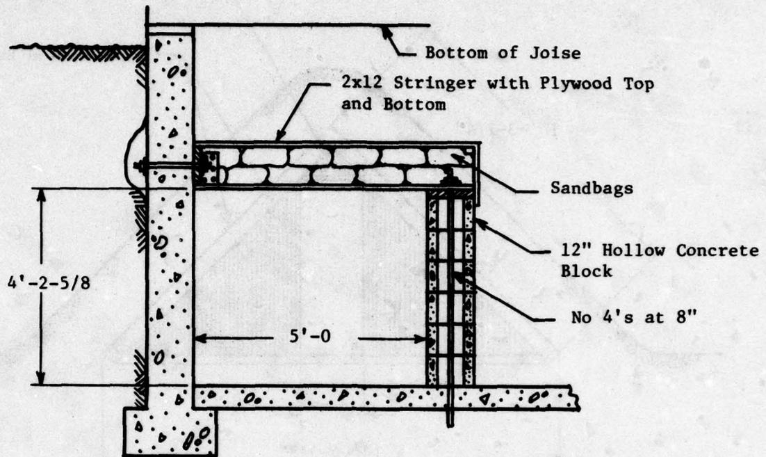
Figure 55. Reinforced Concrete Block Shelter
