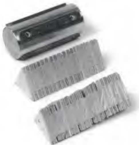
Figure 12. MEM, fresh mitigator, and a crushed mitigator.
