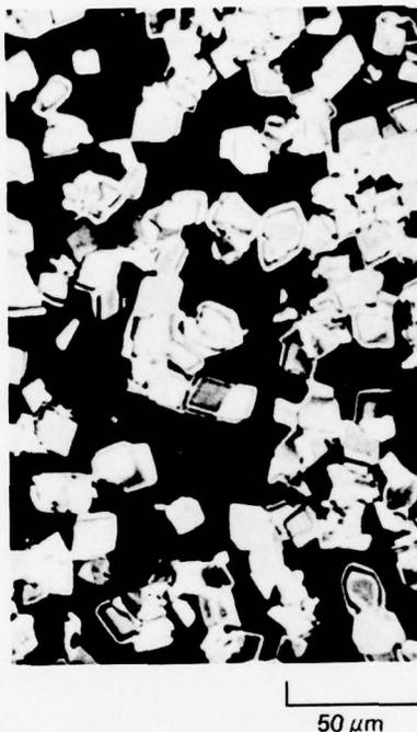
Fig. 14. Optical micrograph of pure DGEBA crystals suspended in an unreacted commercial epoxide.
