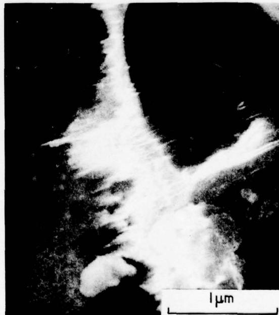
Figure 2 Scanning electron micrograph of fibrils that have swept onto the fracture surface of polycarbonate that deformed and failed under a strain-rate of  $\sim 10^{-2} \text{ min}^{-1}$
