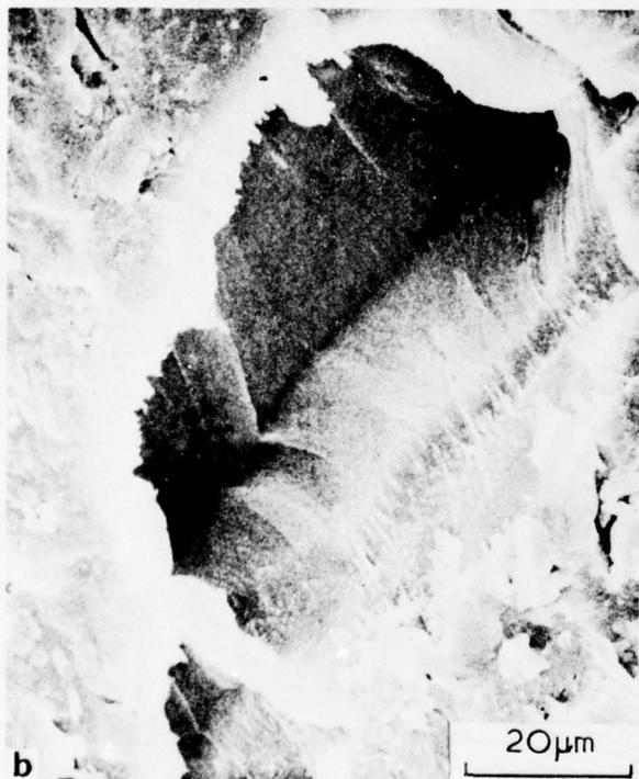
Figure 3 Scanning electron micrographs of the edge of cold drawn polycarbonate that deformed and failed under a strain-rate of  $\sim 10^{-2}$   $\text{min}^{-1}$  illustrating (a) numerous edge cavities and (b) the topography within a cavity
