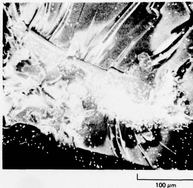
**Fig. 11.** X-ray emission scanning spectroscopy map of sulfur distribution in the fracture surface of TGDDM-DDS (27 wt% DDS) epoxy which was fractured at 250°C.
