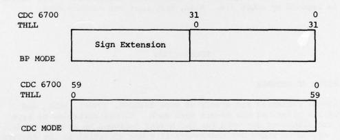
In BP mode, bit 31 on the CDC 6700 is THLL bit 0, while in CDC mode, bit 59 on the CDC is THLL bit 0. Functions such as TEST.BIT, CLR.BIT, SET.BIT, TGL.BIT, and FIND.BIT use the THLL bit number as an input parameter, and FIND.BIT can also output a THLL bit number. These functions are implemented for both compiler modes and will, in general, yield different results since THLL bit assignments are different in both modes.
