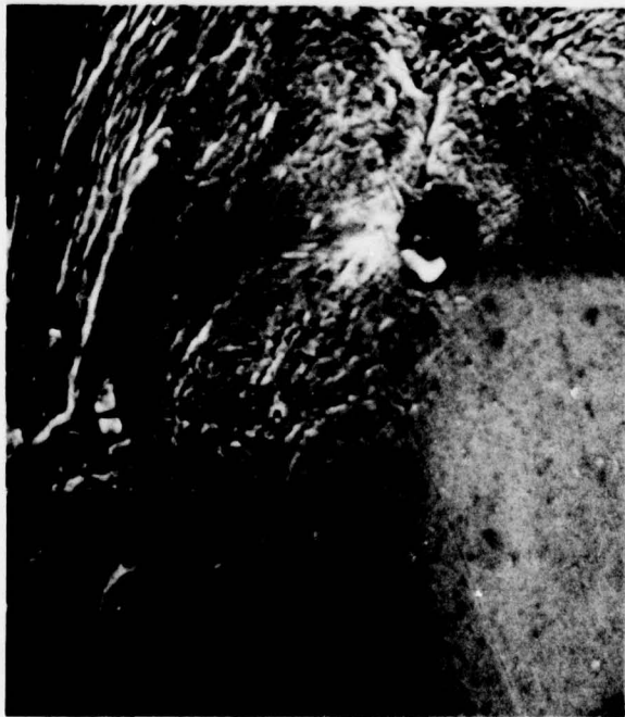
Figure 1. These two photographs are of low-carbon steel, with the fatigue crack grown at \Delta K = 11 \text{ MN/m}^{3/2} in a vacuum of 10^{-5} torr. The photograph on the left (a) was made at K = 2 \text{ MN/m}^{3/2} and the photograph on the right (b) at K = 13 \text{ MN/m}^{3/2} . By imaging these photographs in a stereoscope, the crack tip displacements may be visualized.
