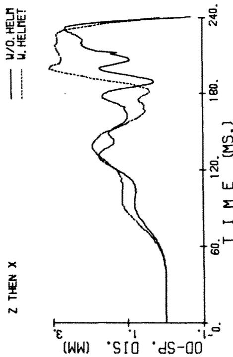
Fig. 18 Odontoid Process Displacement into the Spinal Canal with & without Helmet, Case 2
