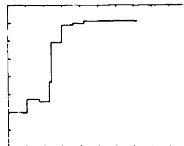
Figure 27. Voltage waveform at the load end of wire 4 of tube 1 with wire 4 of tube 3 driven. Vertical scale is 0.5 V/div; horizontal scale is 5 ns/div.
