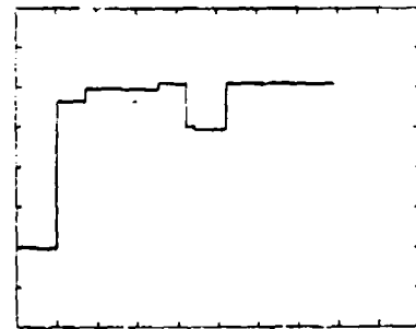
Figure 23. Voltage waveform at the load end of wire 5 of tube 3 with wire 1 of tube 2 driven. Vertical scale is 0.05 V/div; horizontal scale is 5 ns/div.
