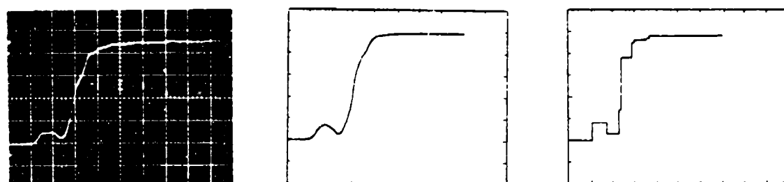
Figure 15. Voltage waveform at the load end of wire 4 of tube 3, with wire 4 of tube 1 driven. Vertical scale is 0.5 V/div; horizontal scale is 5 ns/div.
