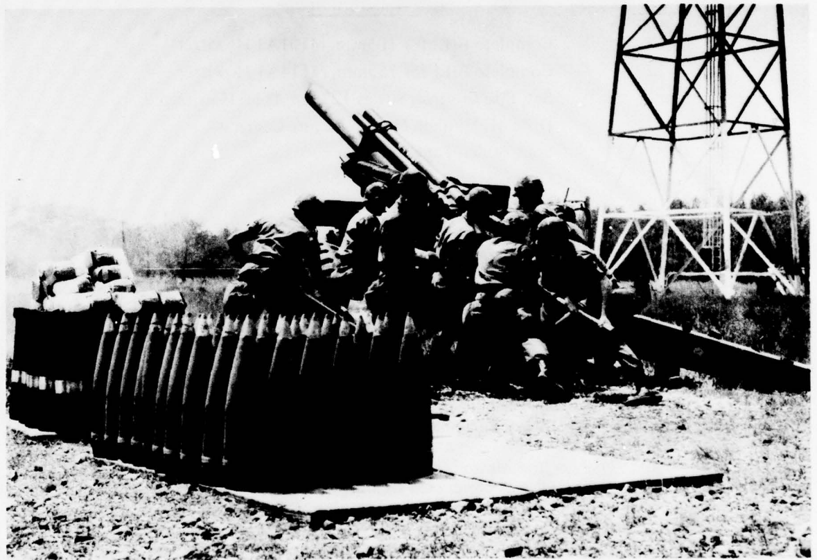
Figure 1. Projectile and propelling charge placement for testing.
