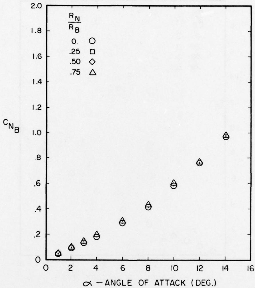
Figure A-32. Normal Force Coefficient Versus Angle of Attack for  $l_N/d = 2$ ,  $l_A/d = 10$ ,  $M = 0.8$
