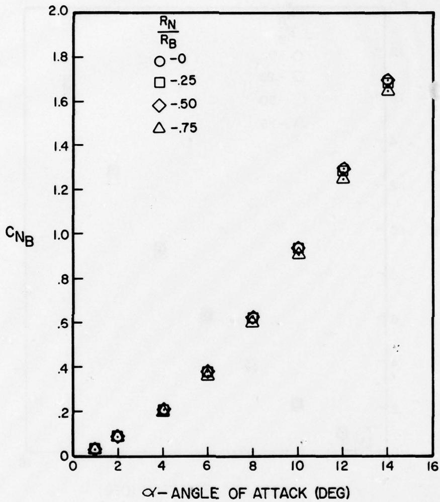
Figure A-60. Normal Force Coefficient Versus Angle of Attack for  $l_N/d = 3$ ,  $l_A/d = 8$ ,  $M = 2.0$
