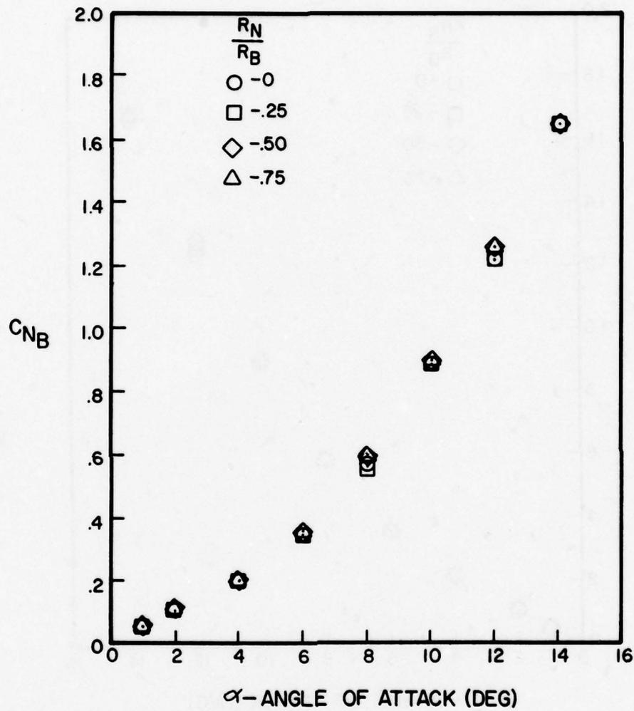
Figure A-53. Normal Force Coefficient Versus Angle of Attack for  $l_N/d = 2$ ,  $l_A/d = 10$ ,  $M = 1.5$
