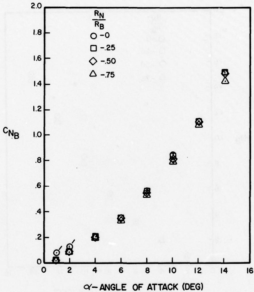
Figure A-57. Normal Force Coefficient Versus Angle of Attack for  $l_N/d = 3$ ,  $l_A/d = 6$ ,  $M = 2.0$
