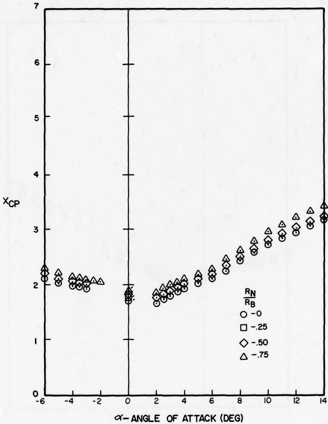
Figure A-113. Center of Pressure Versus Angle of Attack for  $l_N/d = 2$ ,  $l_A/d = 6$ ,  $M = 2.0$
