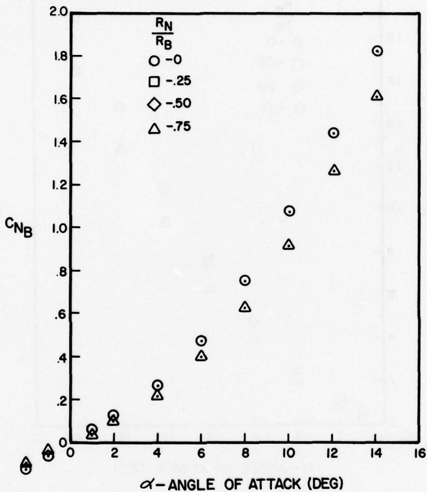
Figure A-69. Normal Force Coefficient Versus Angle of Attack for  $l_N/d = 3$ ,  $l_A/d = 8$ ,  $M = 3.0$
