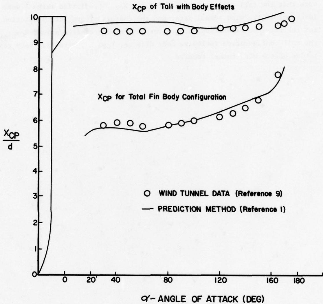
Figure 18. Center of Pressure Versus Angle of Attack for 10-Caliber Finned Body
