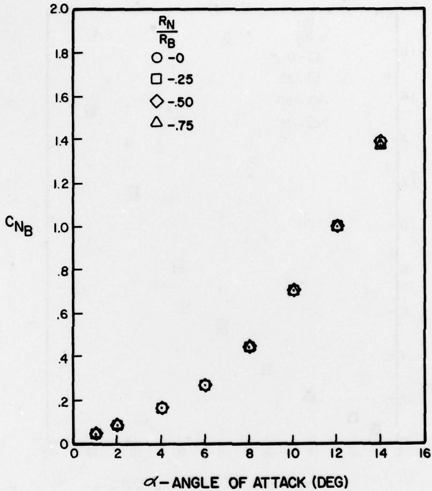
Figure A-49. Normal Force Coefficient Versus Angle of Attack for  $l_N/d = 4$ ,  $l_A/d = 6$ ,  $M = 1.5$
