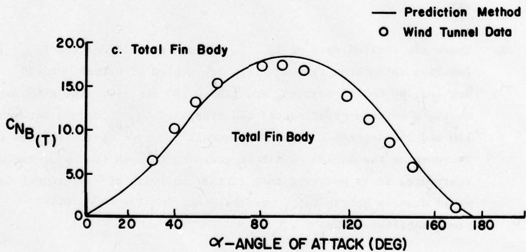
Figure 16. Normal Force Coefficient Versus Angle of Attack for the 10-Caliber Finned Body
