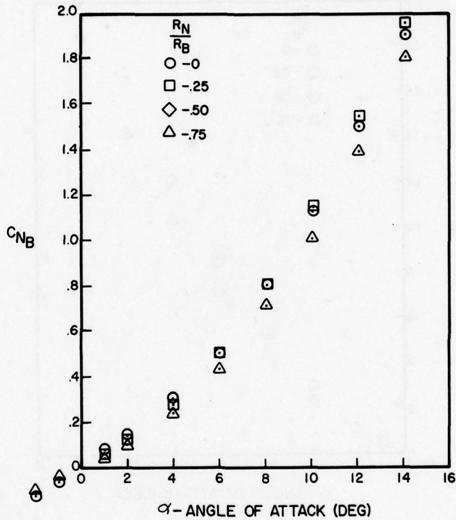
Figure A-71. Normal Force Coefficient Versus Angle of Attack for  $l_N/d = 2$ ,  $l_A/d = 10$ ,  $M = 3.0$
