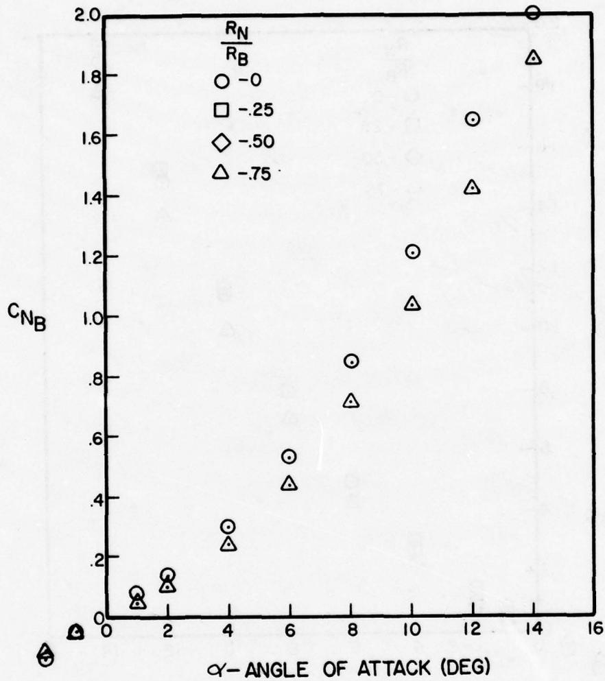
Figure A-72. Normal Force Coefficient Versus Angle of Attack for  $l_N/d = 3$ ,  $l_A/d = 10$ ,  $M = 3.0$
