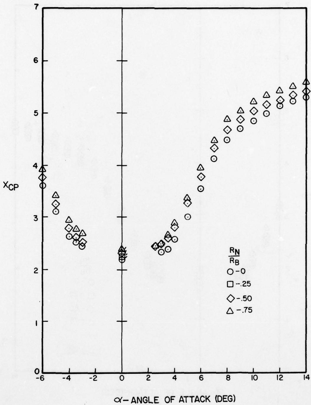
Figure A-120. Center of Pressure Versus Angle of Attack for  $l_N/d = 3$ ,  $l_A/d = 10$ ,  $M = 2.0$
