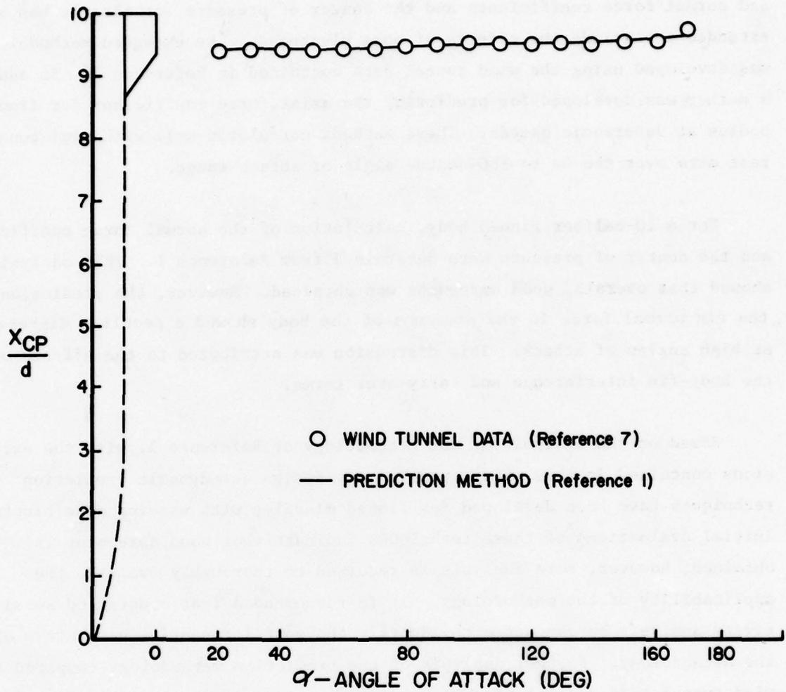
Figure 19. Tail Only Center of Pressure Versus Angle of Attack for 10-Caliber Finned Body
