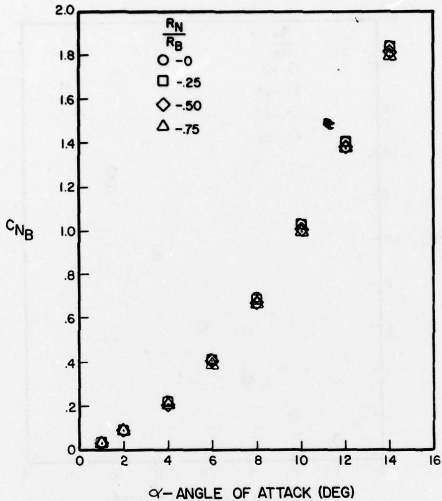
Figure A-62. Normal Force Coefficient Versus Angle of Attack for  $l_N/d = 2$ ,  $l_A/d = 10$ ,  $M = 2.0$
