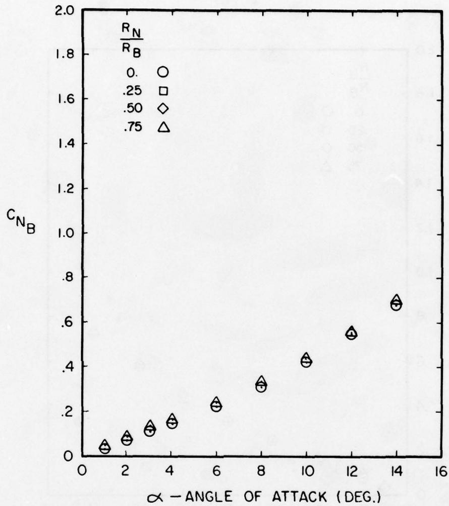
Figure A-23. Normal Force Coefficient Versus Angle of Attack for  $l_N/d = 2$ ,  $l_A/d = 6$ ,  $M = 0.6$
