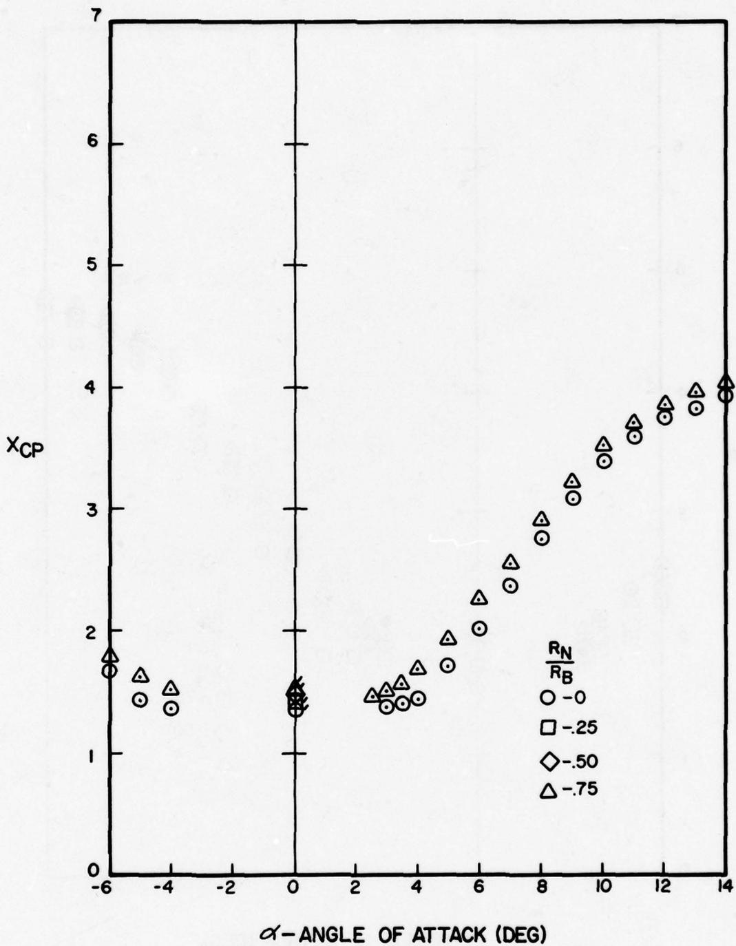
Figure A-105. Center of Pressure Versus Angle of Attack for  $l_N/d = 3$ ,  $l_A/d = 6$ ,  $M = 1.5$
