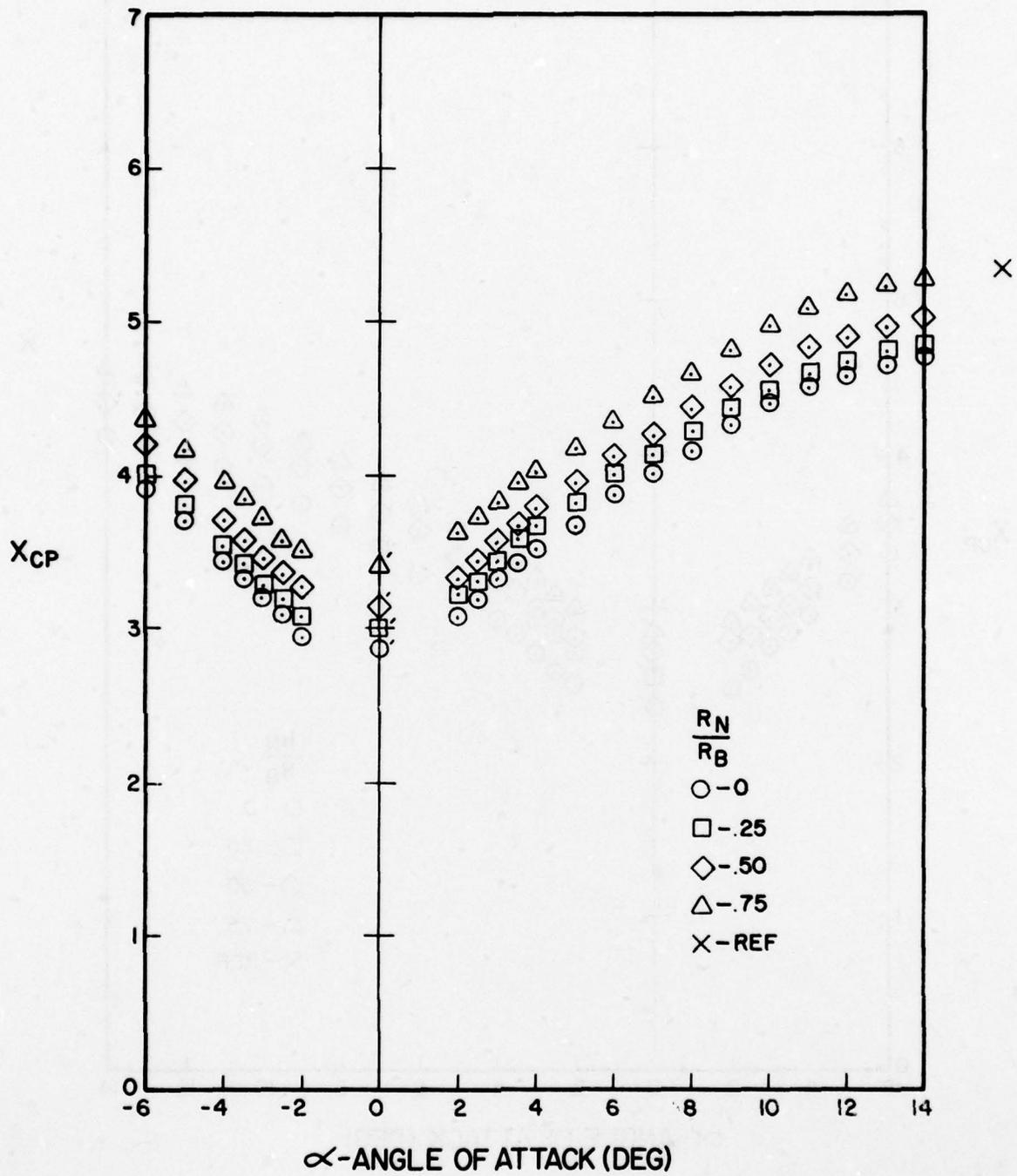
Figure A-124. Center of Pressure Versus Angle of Attack for  $l_N/d = 4$ ,  $l_A/d = 6$ ,  $M = 3.0$
