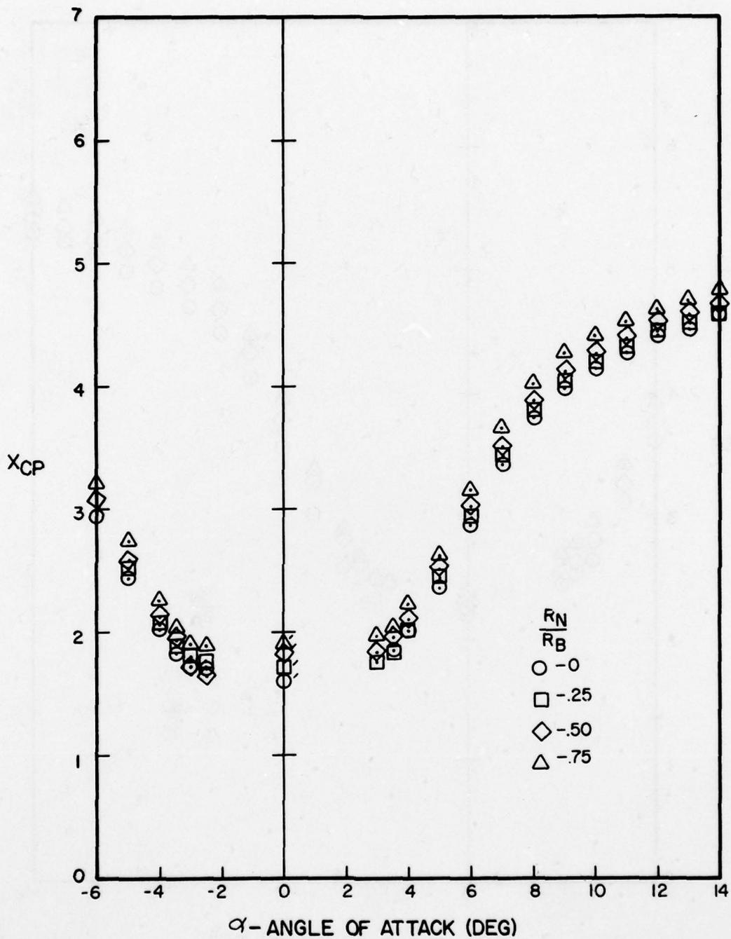
Figure A-119. Center of Pressure Versus Angle of Attack for  $\lambda_N/d = 2$ ,  $\lambda_A/d = 10$ ,  $M = 2.0$
