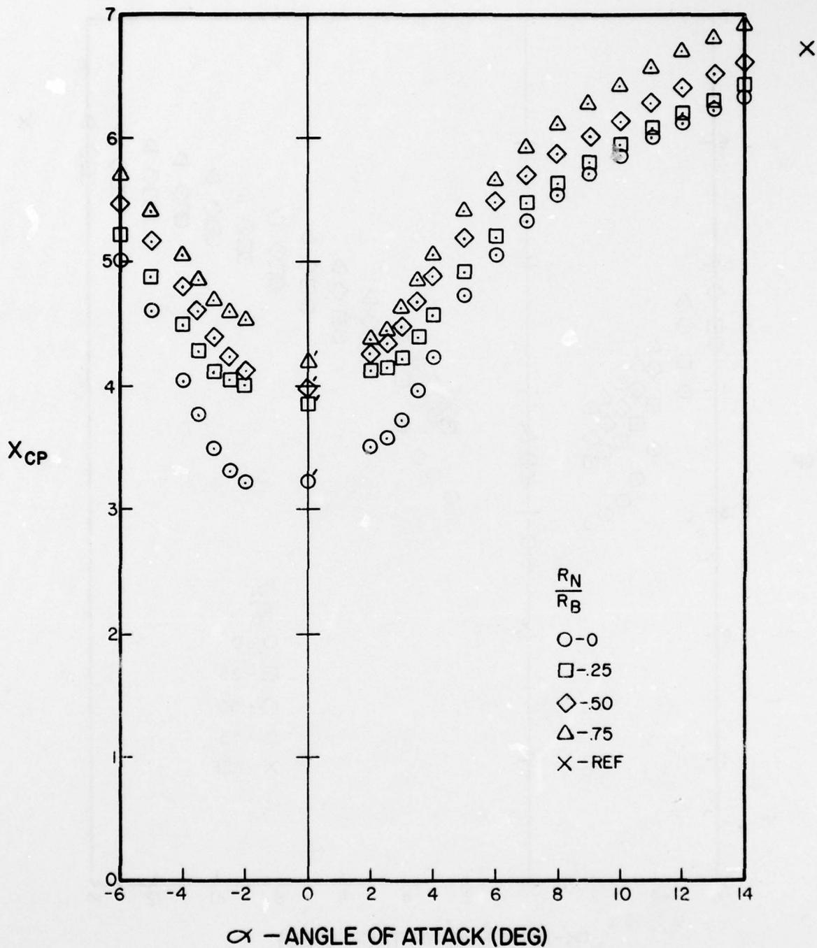
Figure A-130. Center of Pressure Versus Angle of Attack for  $l_N/d = 4$ ,  $l_A/d = 10$ ,  $M = 3.0$
