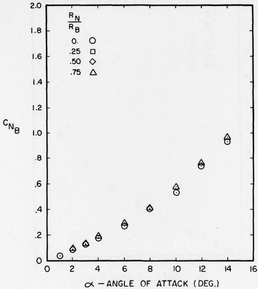
Figure A-42. Normal Force Coefficient Versus Angle of Attack for  $l_N/d = 3$ ,  $l_A/d = 6$ ,  $M = 1.2$
