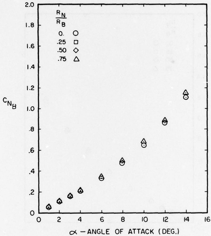
Figure A-39. Normal Force Coefficient Versus Angle of Attack for  $l_N/d = 3$ ,  $l_A/d = 10$ ,  $M = 1.0$
