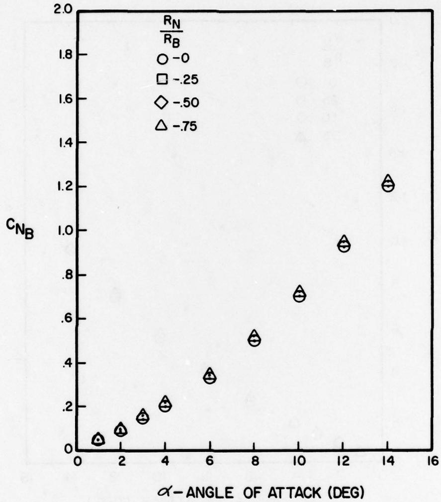
Figure A-44. Normal Force Coefficient Versus Angle of Attack for  $l_N/d = 2$ ,  $l_A/d = 10$ ,  $M = 1.2$
