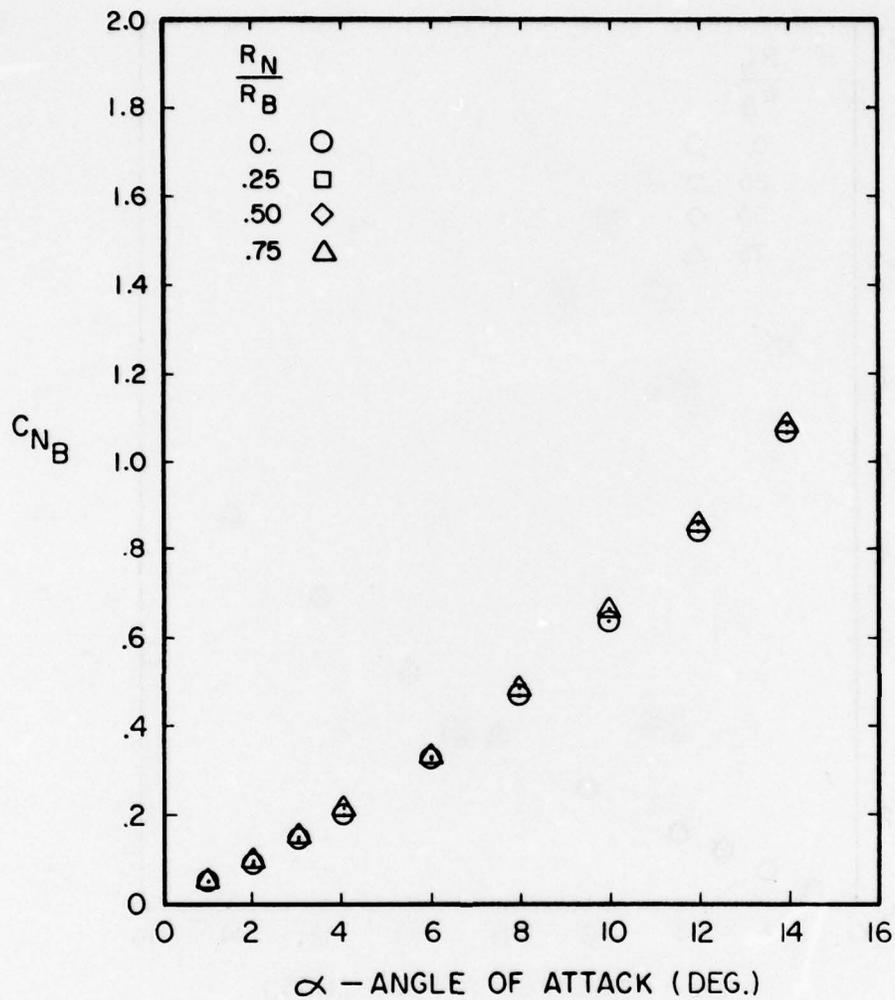
Figure A-38. Normal Force Coefficient Versus Angle of Attack for  $l_N/d = 2$ ,  $l_A/d = 10$ ,  $M = 1.0$
