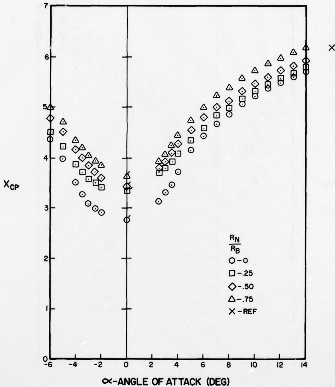
Figure A-129. Center of Pressure Versus Angle of Attack for  $l_N/d = 3$ ,  $l_A/d = 10$ ,  $M = 3.0$
