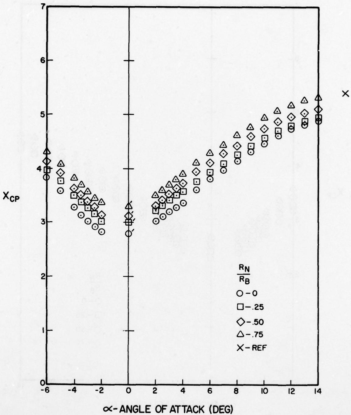
Figure A-126. Center of Pressure Versus Angle of Attack for  $l_N/d = 3$ ,  $l_A/d = 8$ ,  $M = 3.0$
