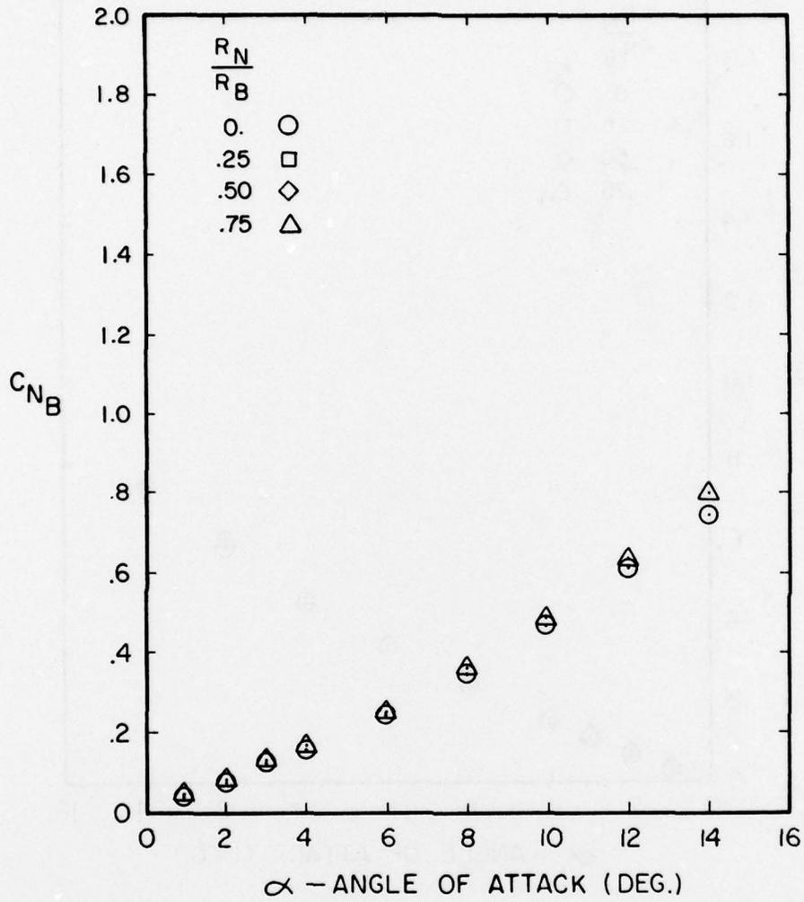
Figure 30. Normal Force Coefficient Versus Angle of Attack
