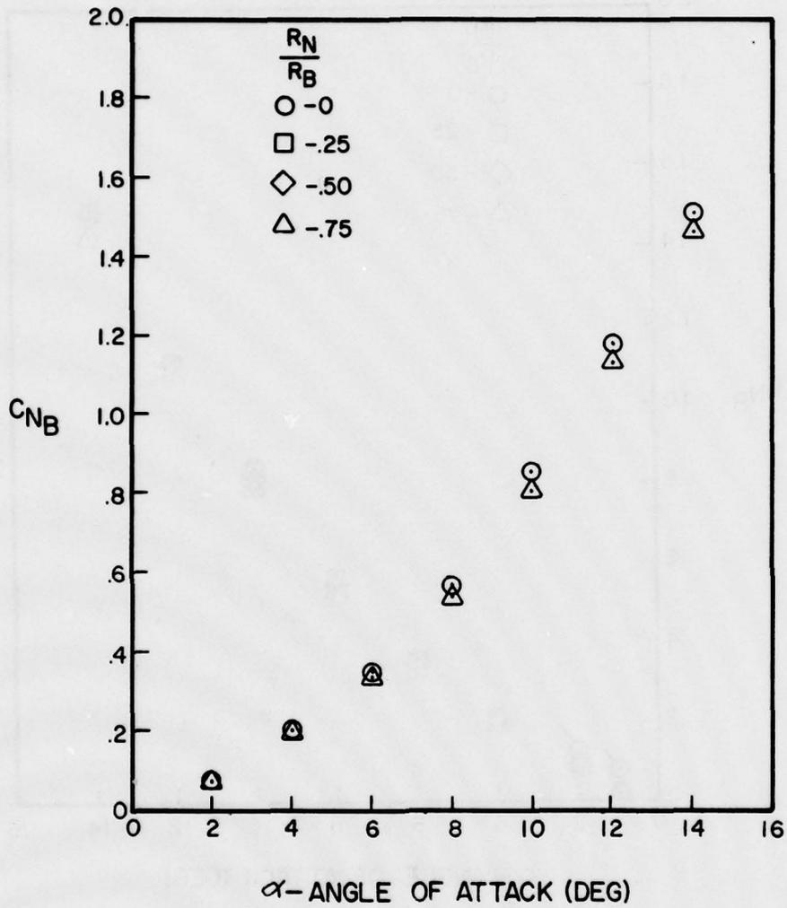
Figure A-58. Normal Force Coefficient Versus Angle of Attack for  $l_N/d = 4$ ,  $l_A/d = 6$ ,  $M = 2.0$
