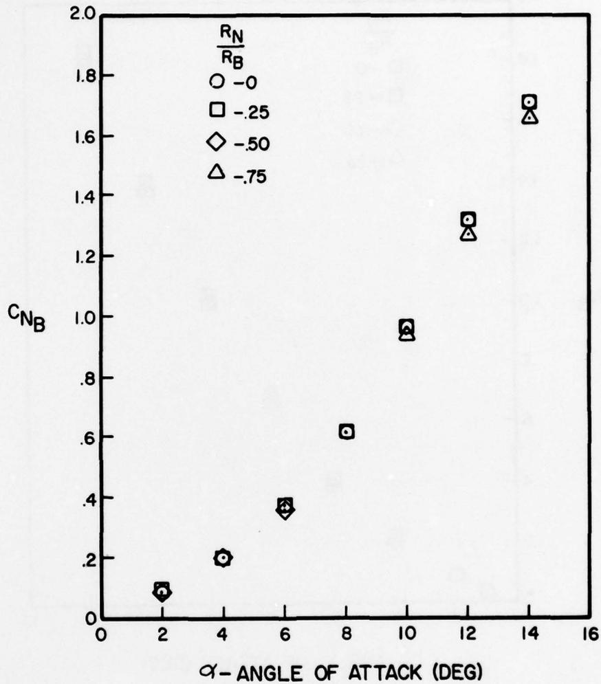
Figure A-61. Normal Force Coefficient Versus Angle of Attack for  $l_N/d = 4$ ,  $l_A/d = 8$ ,  $M = 2.0$
