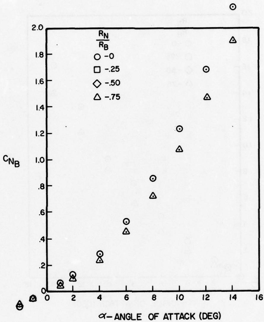
Figure A-73. Normal Force Coefficient Versus Angle of Attack for  $l_N/d = 4$ ,  $l_A/d = 10$ ,  $M = 3.0$
