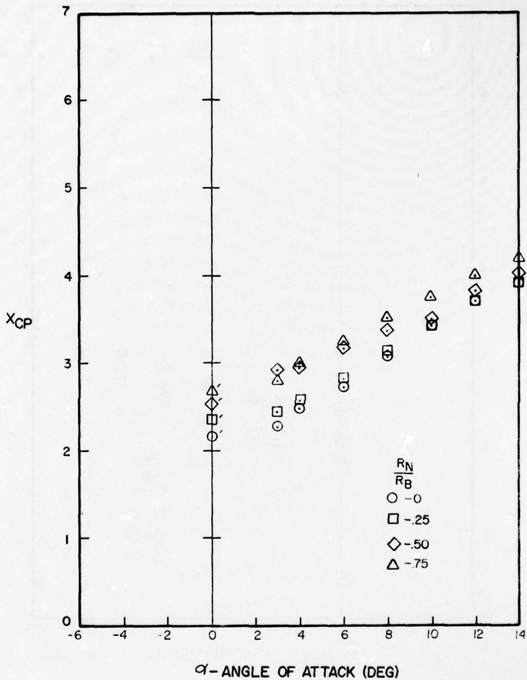
Figure A-88. Center of Pressure Versus Angle of Attack for  $l_N/d = 4$ ,  $l_A/d = 6$ ,  $M = 0.8$
