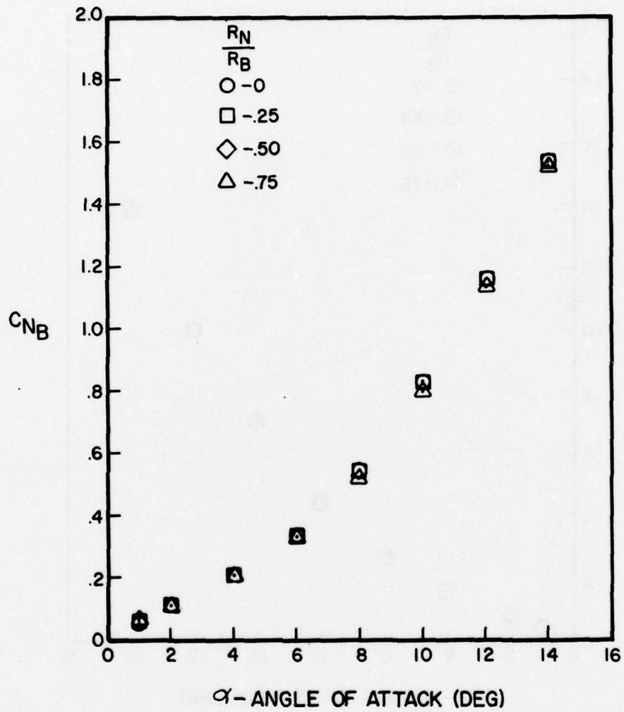
Figure A-50. Normal Force Coefficient Versus Angle of Attack for  $l_N/d = 3$ ,  $l_A/d = 8$ ,  $M = 1.5$
