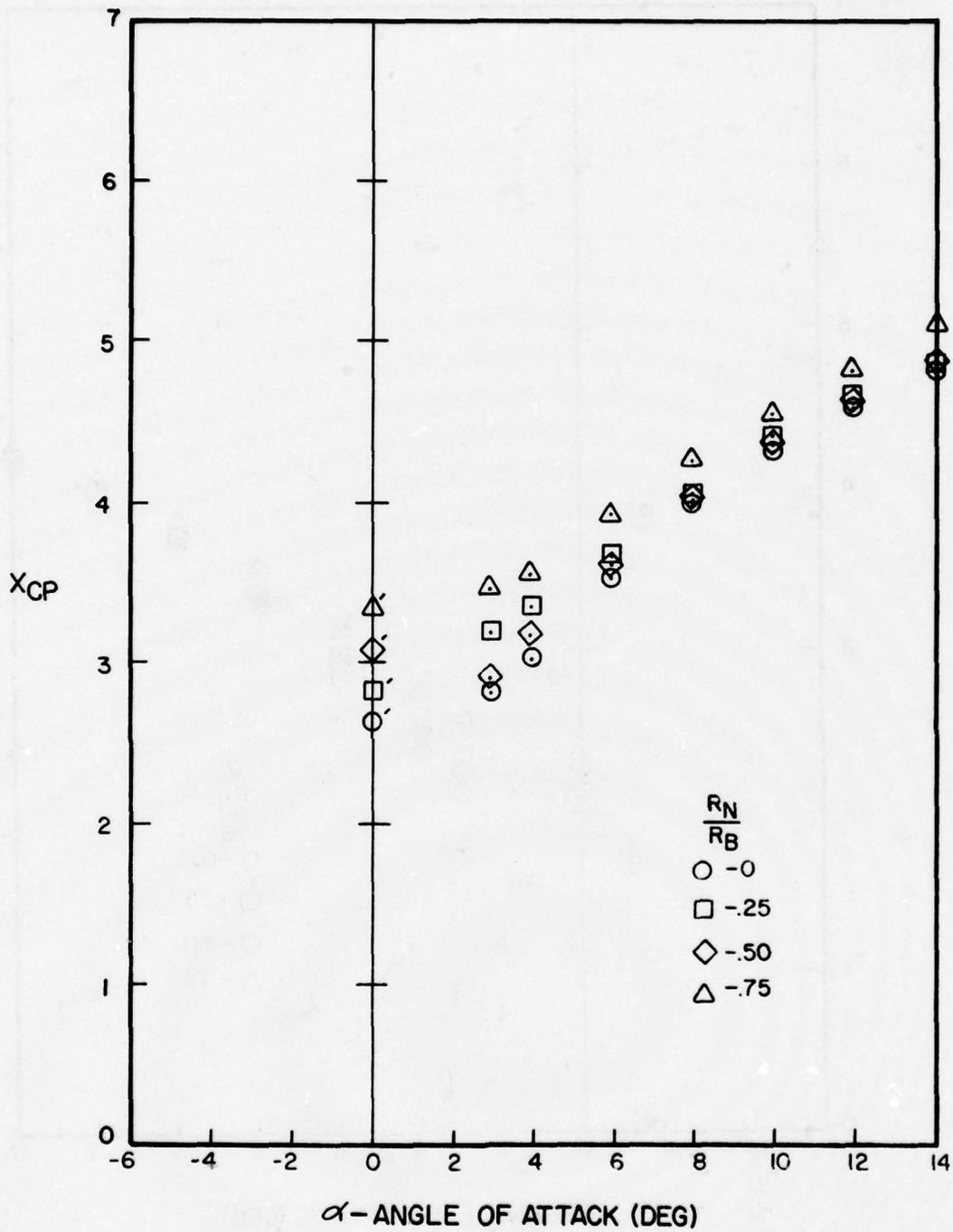
Figure A-90. Center of Pressure Versus Angle of Attack for  $l_N/d = 3$ ,  $l_A/d = 10$ ,  $M = 0.8$
