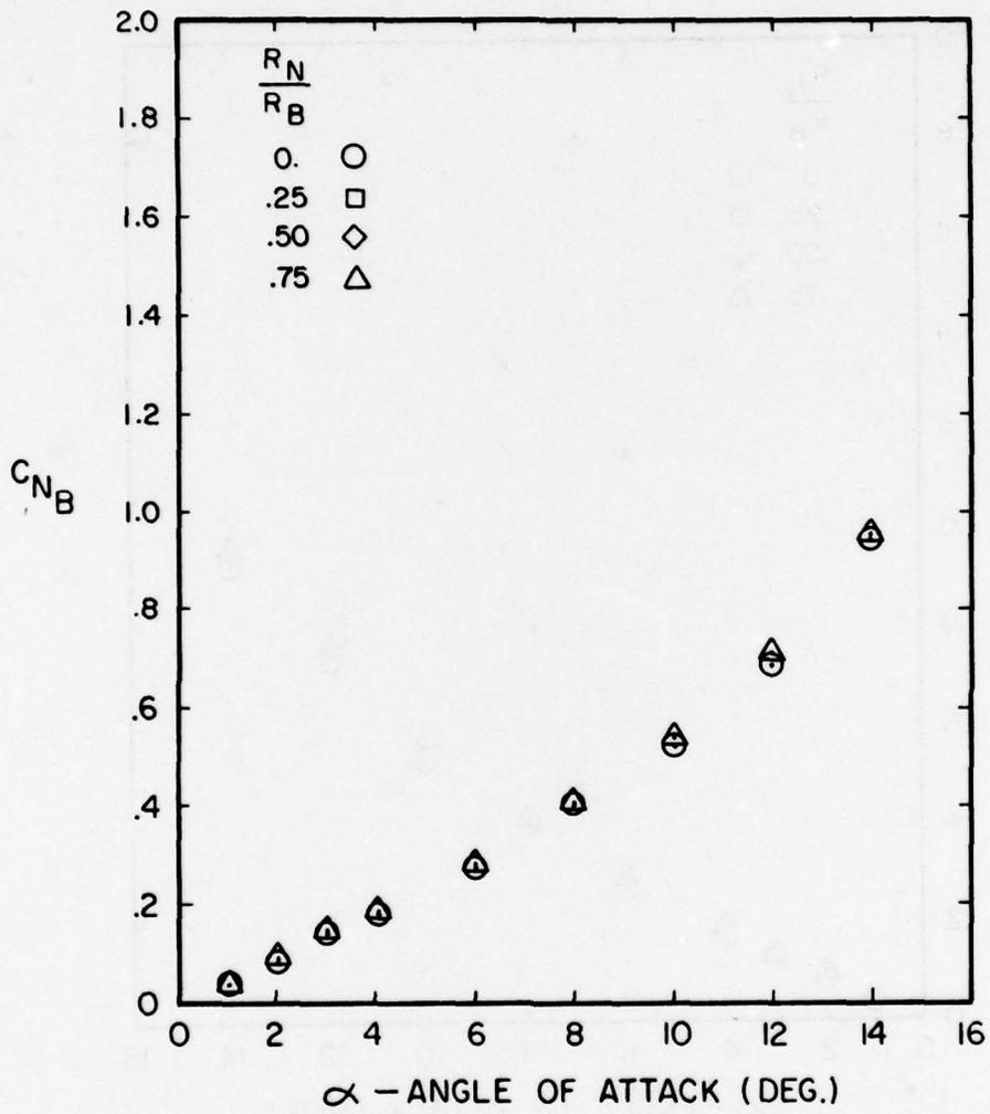
Figure A-41. Normal Force Coefficient Versus Angle of Attack for  $l_N/d = 2$ ,  $l_A/d = 6$ ,  $M = 1.2$
