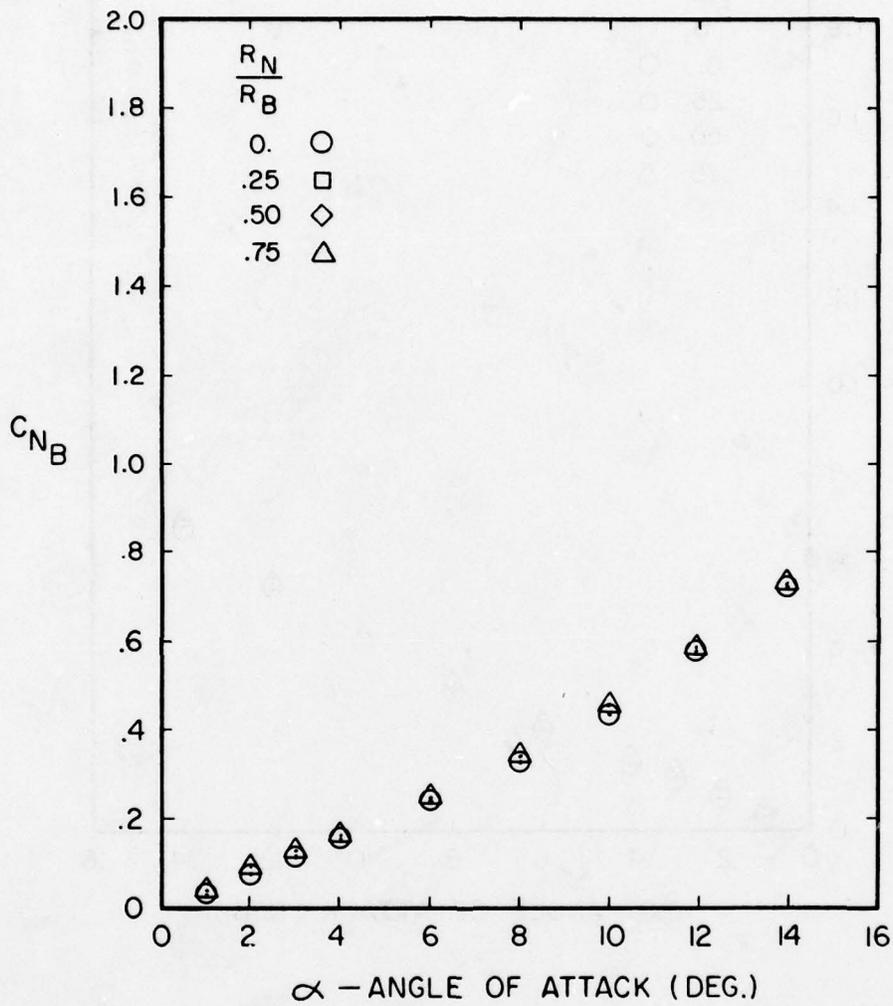
Figure A-24. Normal Force Coefficient Versus Angle of Attack for  $l_N/d = 3$ ,  $l_A = 6$ ,  $M = 0.6$
