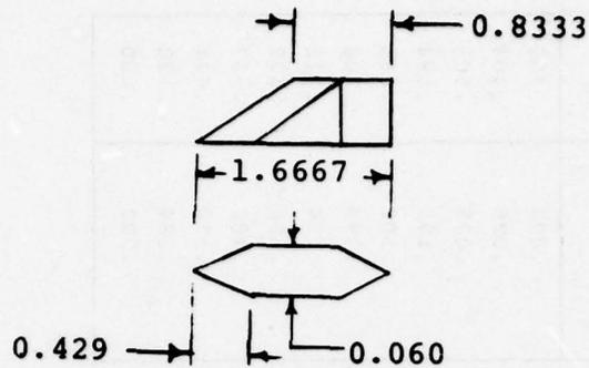
Figure 13. Fin Geometry for a Slender Body Model
