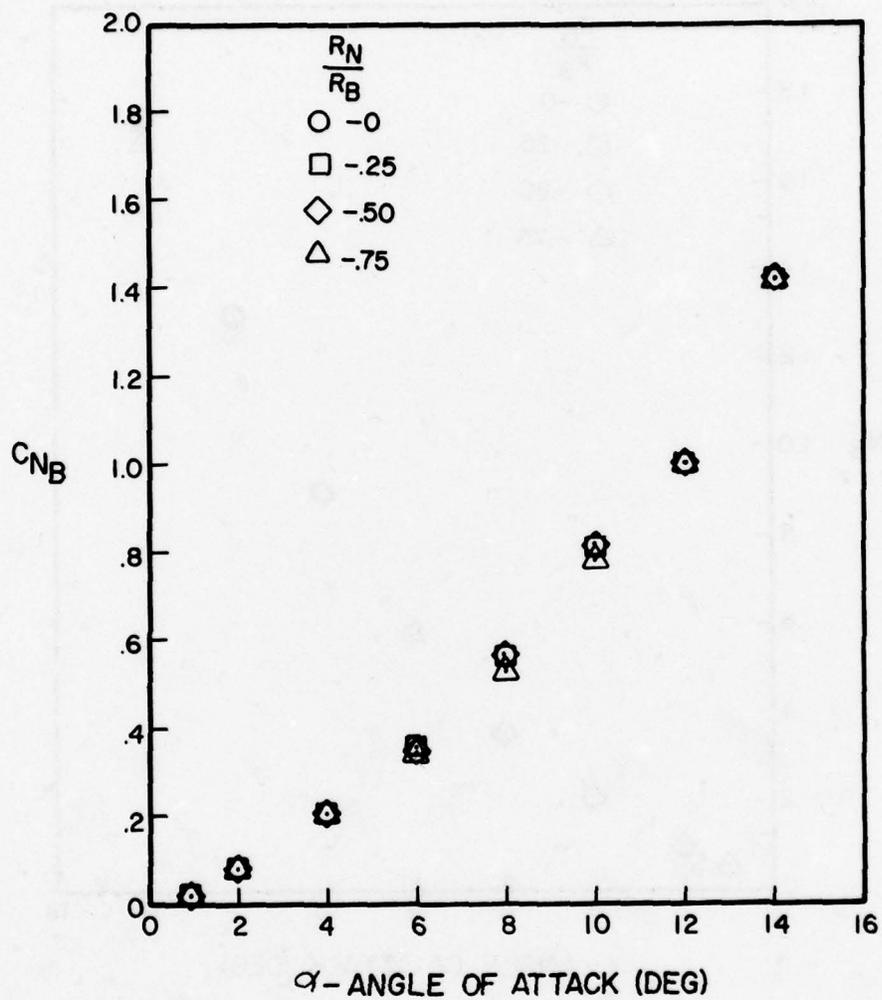
Figure A-56. Normal Force Coefficient Versus Angle of Attack for  $l_N/d = 2$ ,  $l_A/d = 6$ ,  $M = 2.0$
