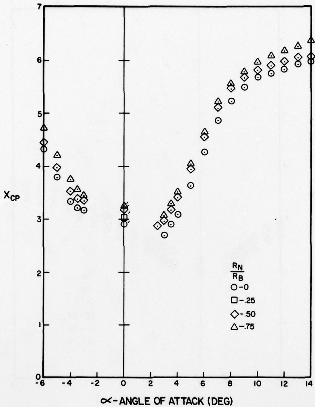
Figure A-121. Center of Pressure Versus Angle of Attack for  $l_N/d = 4$ ,  $l_A/d = 10$ ,  $M = 2.0$
