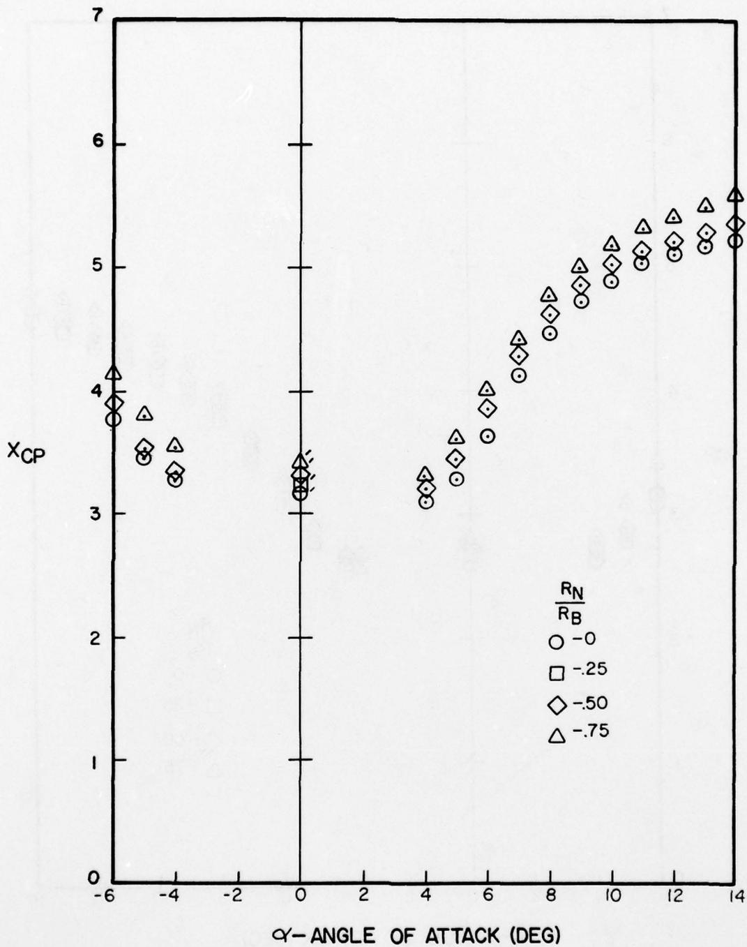
Figure A-118. Center of Pressure Versus Angle of Attack for  $l_N/d = 4$ ,  $l_A/d = 8$ ,  $M = 2.0$
