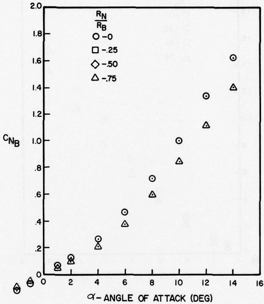
Figure A-66. Normal Force Coefficient Versus Angle of Attack for  $l_N/d = 3$ ,  $l_A/d = 6$ ,  $M = 3.0$
