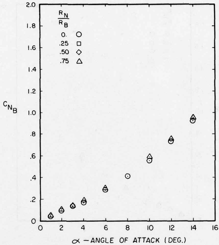
Figure A-27. Normal Force Coefficient Versus Angle of Attack for  $l_N/d = 3$ ,  $l_A/d = 10$ ,  $M = 0.6$
