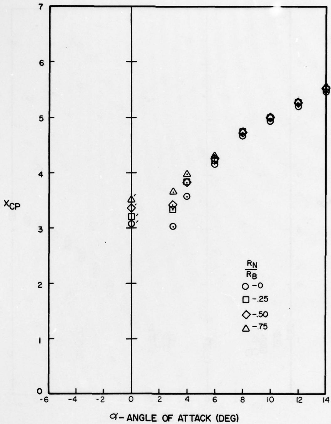
Figure A-103. Center of Pressure Versus Angle of Attack for  $l_N/d = 4$ ,  $l_A/d = 10$ ,  $M = 1.2$
