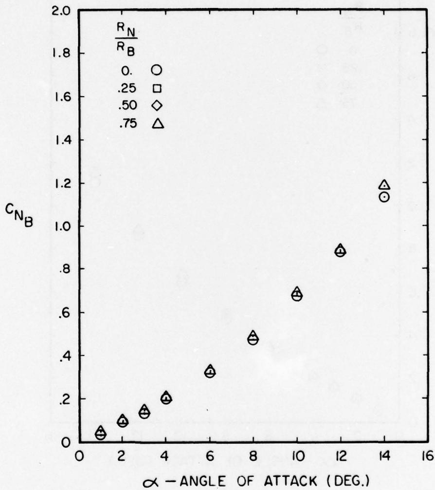
Figure A-40. Normal Force Coefficient Versus Angle of Attack for  $l_N/d = 4$ ,  $l_A/d = 10$ ,  $M = 1.0$
