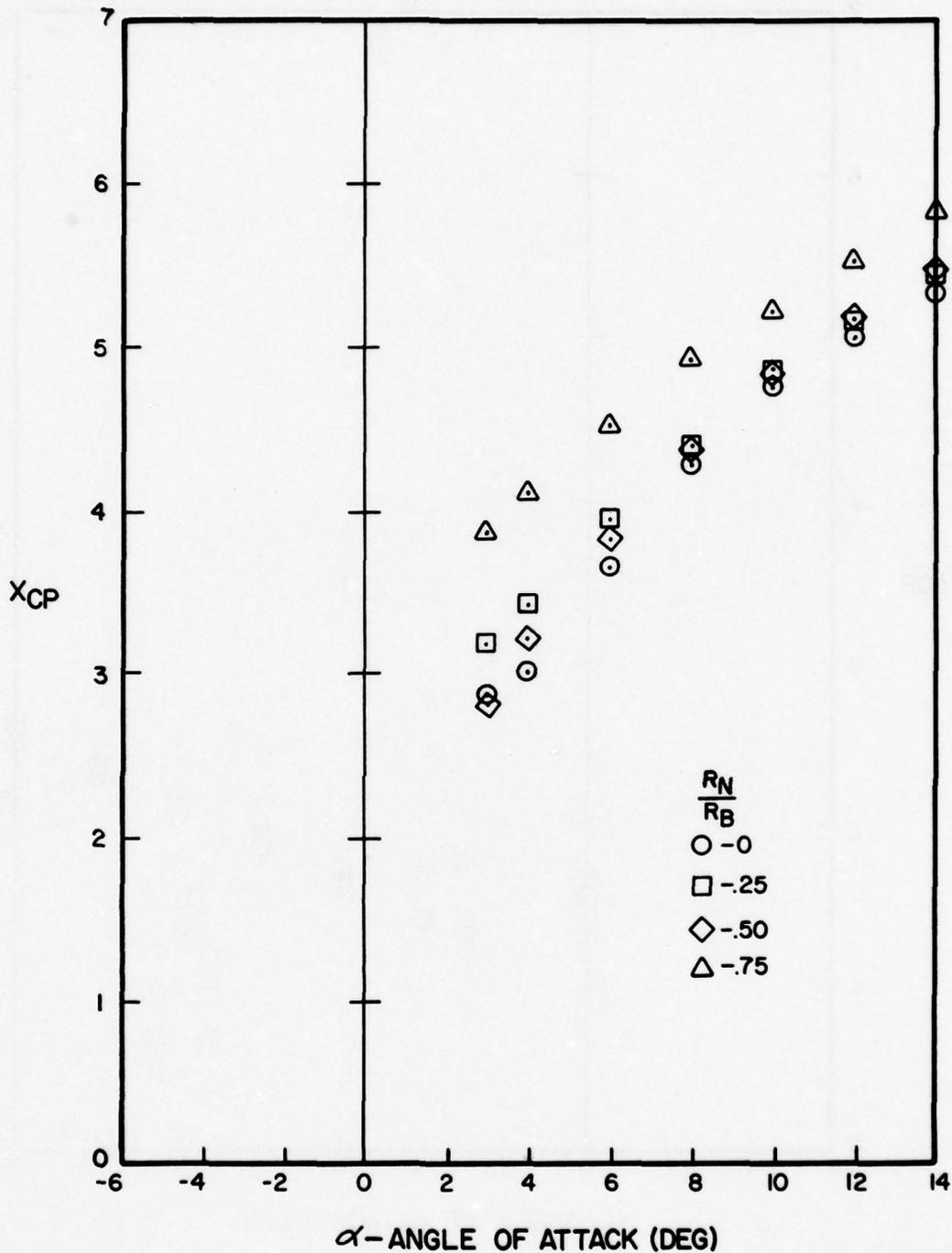
Figure A-85. Center of Pressure Versus Angle of Attack for  $l_N/d = 4$ ,  $l_A/d = 10$ ,  $M = 0.6$
