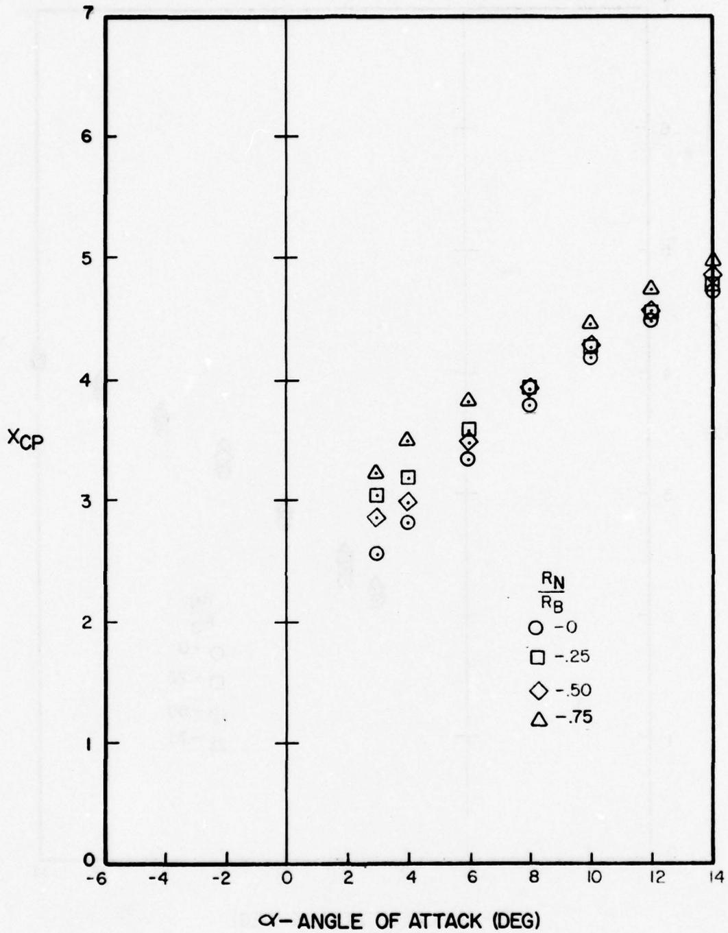
Figure A-84. Center of Pressure Versus Angle of Attack for  $l_N/d = 3$ ,  $l_A/d = 10$ ,  $M = 0.6$
