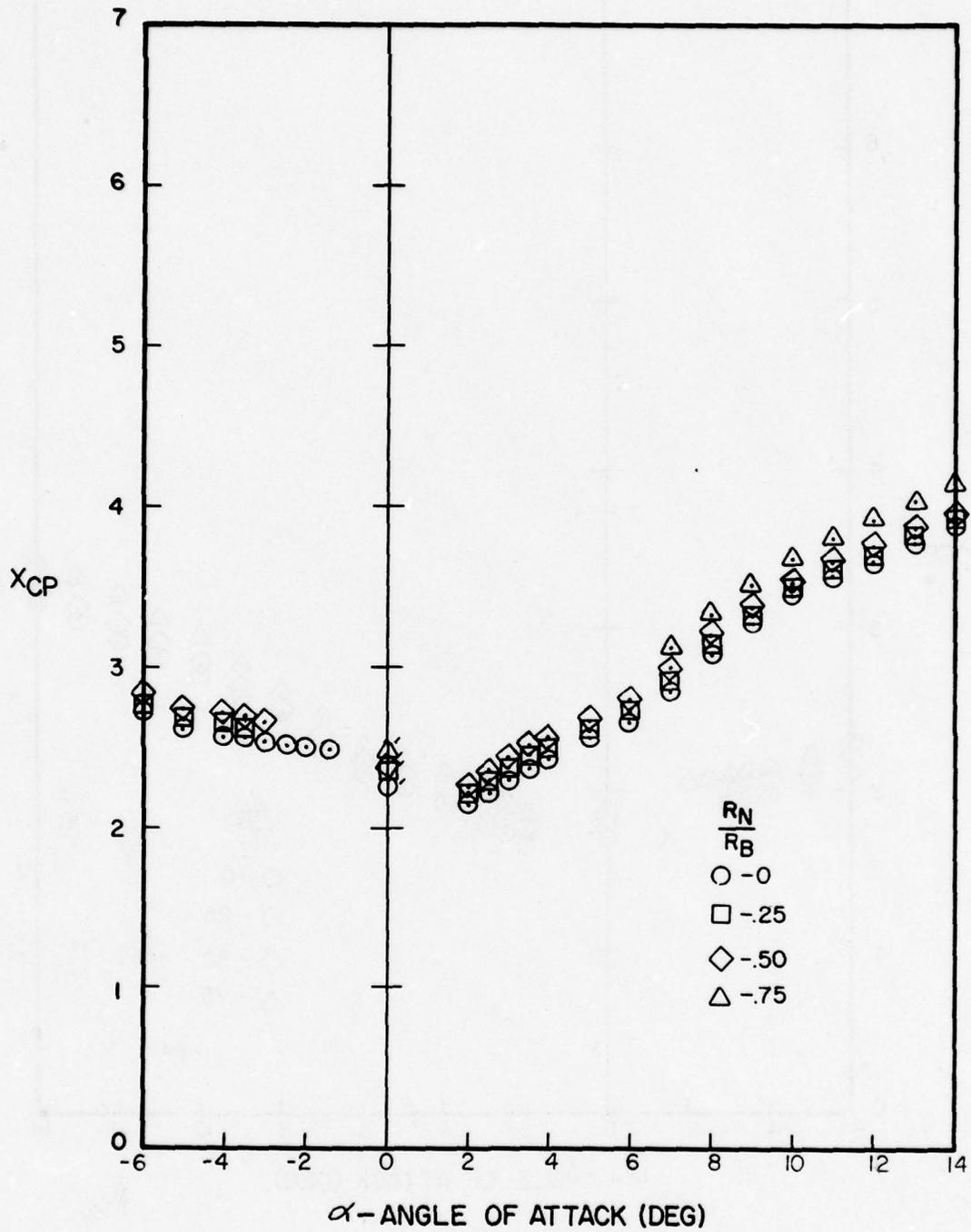
Figure A-114. Center of Pressure Versus Angle of Attack for  $l_N/d = 3$ ,  $l_A/d = 6$ ,  $M = 2.0$
