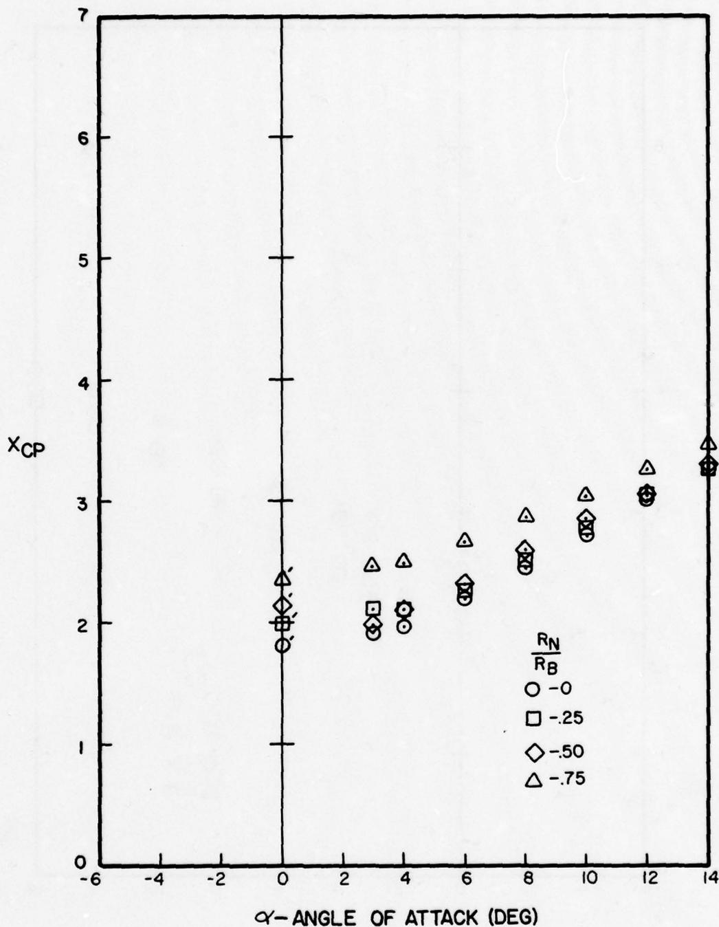
Figure A-87. Center of Pressure Versus Angle of Attack for  $l_N/d = 3$ ,  $l_A/d = 6$ ,  $M = 0.8$
