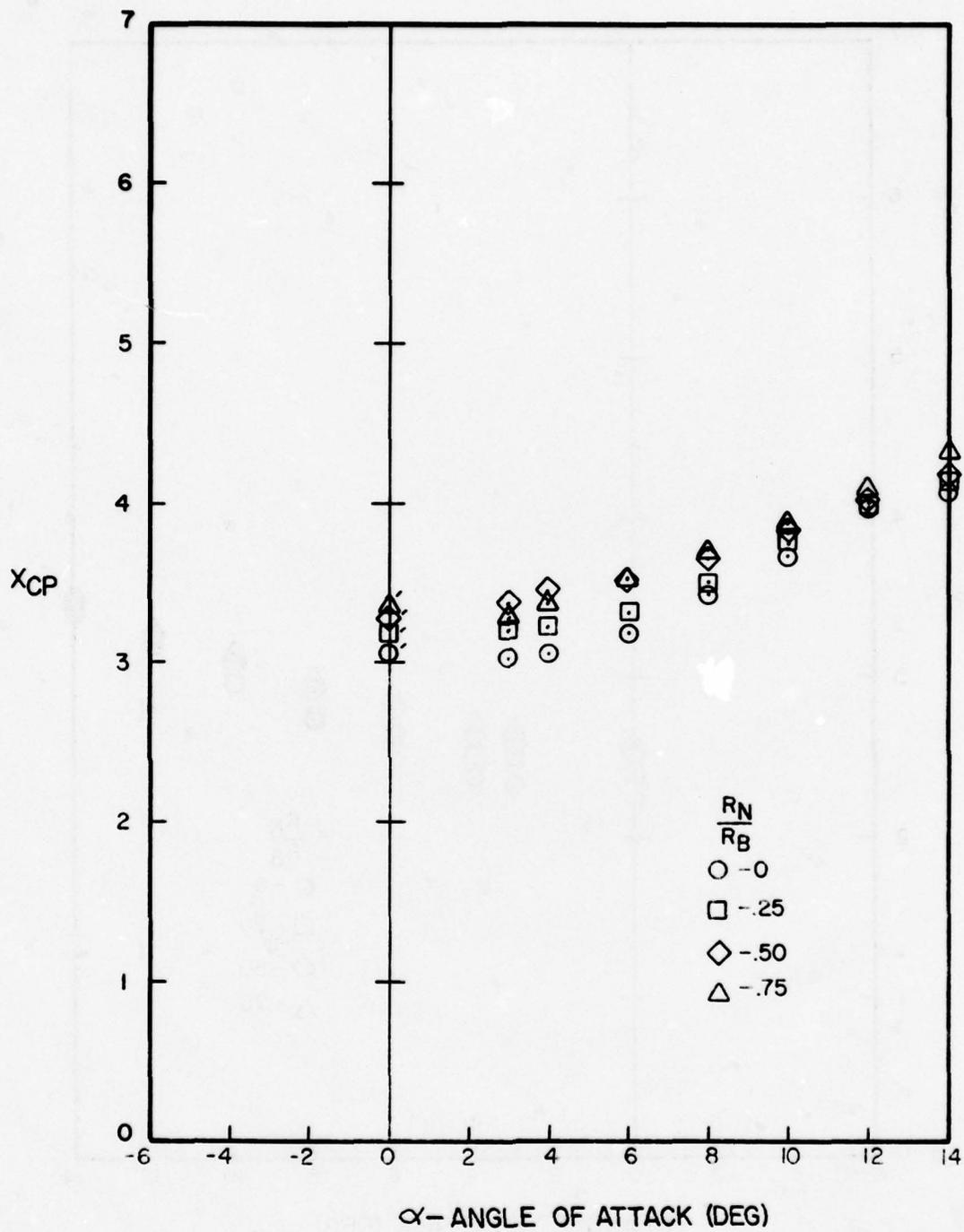
Figure A-94. Center of Pressure Versus Angle of Attack for  $l_N/d = 4$ ,  $l_A/d = 6$ ,  $M = 1.0$
