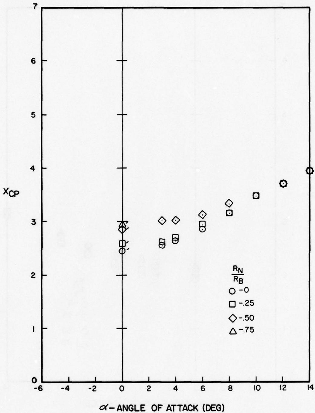
Figure A-100. Center of Pressure Versus Angle of Attack for  $l_N/d = 4$ ,  $l_A/d = 6$ ,  $M = 1.2$
