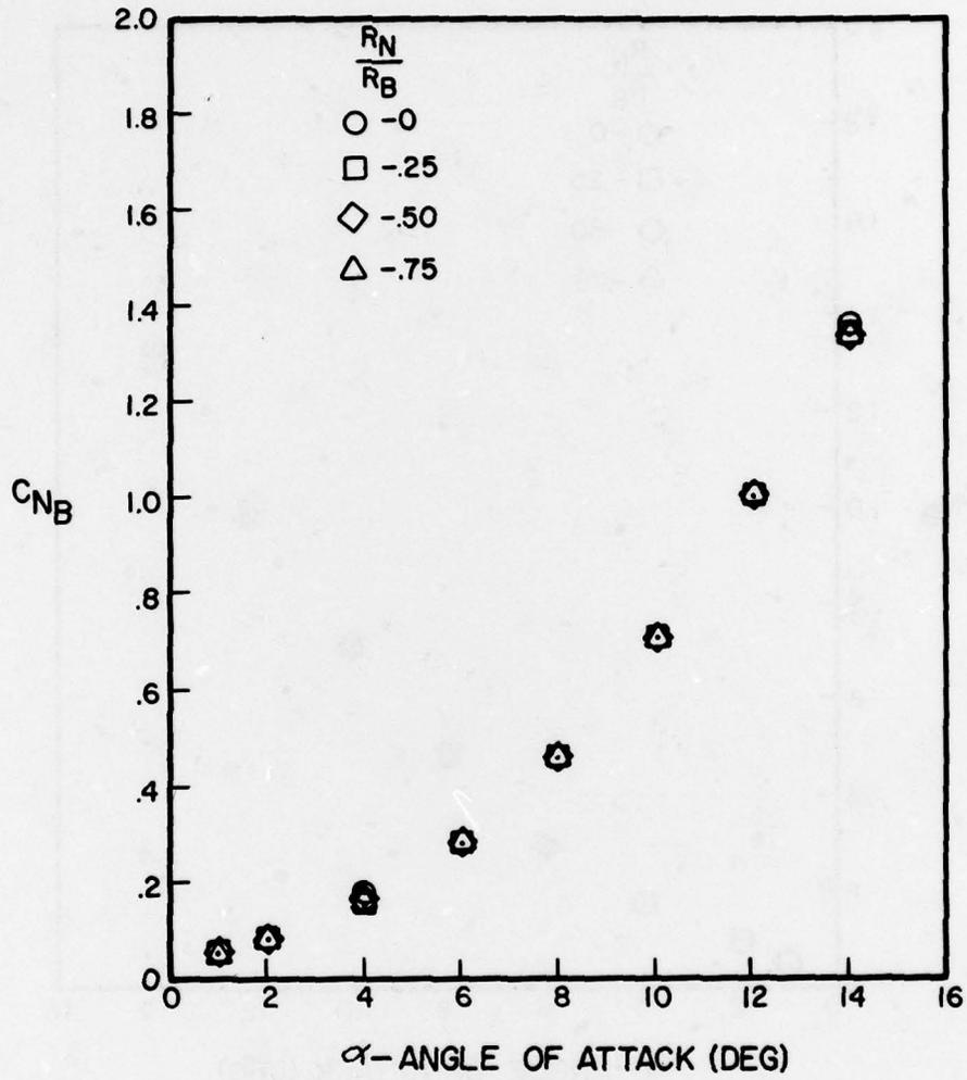
Figure A-48. Normal Force Coefficient Versus Angle of Attack for  $l_N/d = 3$ ,  $l_A/d = 6$ ,  $M = 1.5$
