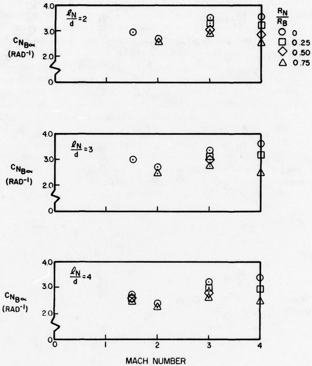
Figure 6. Variation of  $C_{N_{\alpha}}$  with Mach Number for  $\ell_A/d = 8$
