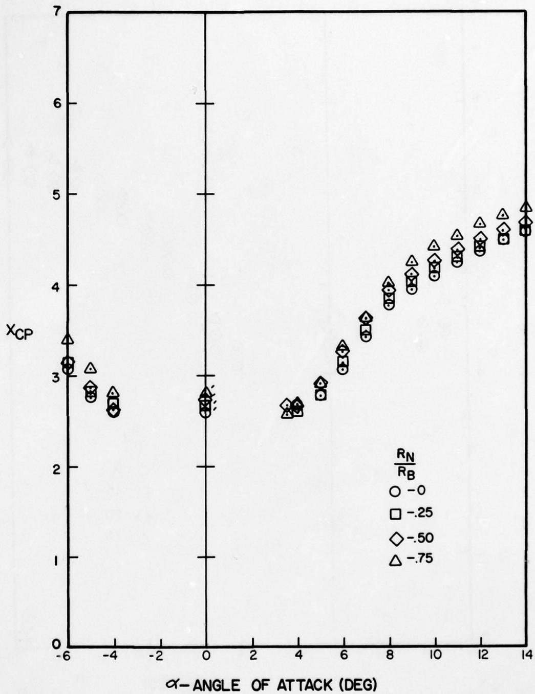
Figure A-117. Center of Pressure Versus Angle of Attack for  $l_N/d = 3$ ,  $l_A/d = 8$ ,  $M = 2.0$
