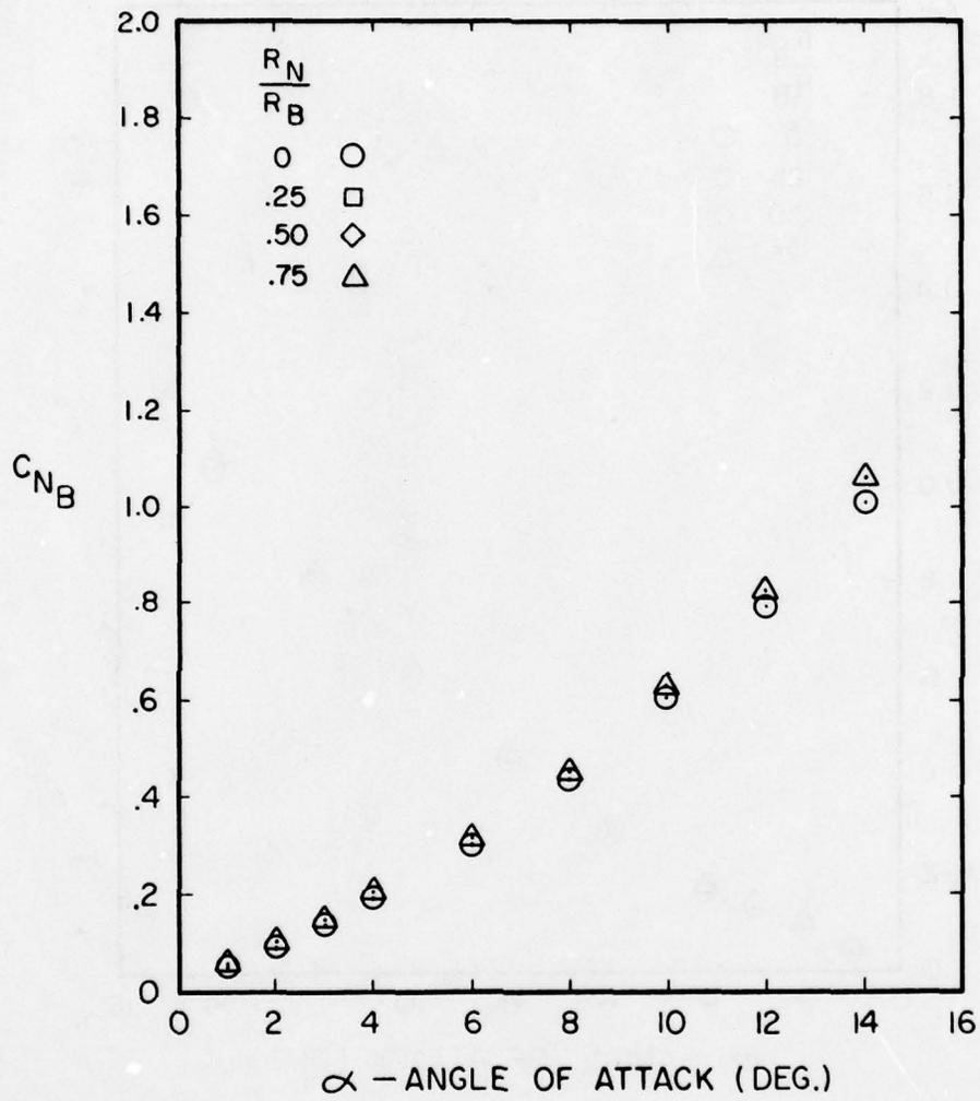
Figure A-33. Normal Force Coefficient Versus Angle of Attack for  $l_N/d = 3$ ,  $l_A/d = 10$ ,  $M = 0.8$
