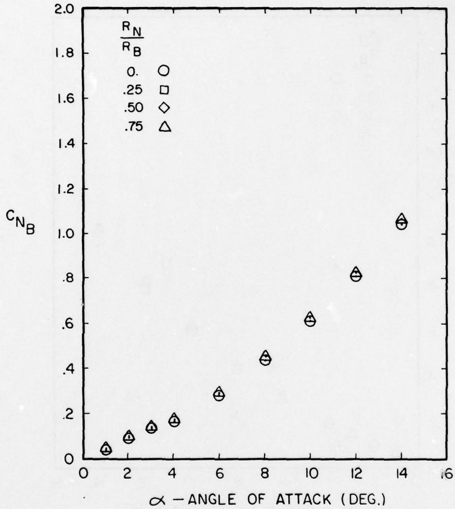
Figure A-34. Normal Force Coefficient Versus Angle of Attack for  $l_N/d = 4$ ,  $l_A/d = 10$ ,  $M = 0.8$
