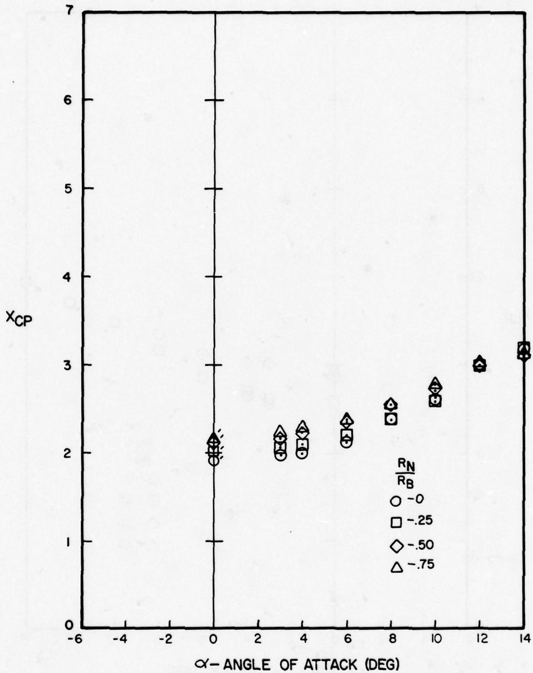
Figure A-99. Center of Pressure Versus Angle of Attack for  $l_N/d = 3$ ,  $l_A/d = 6$ ,  $M = 1.2$
