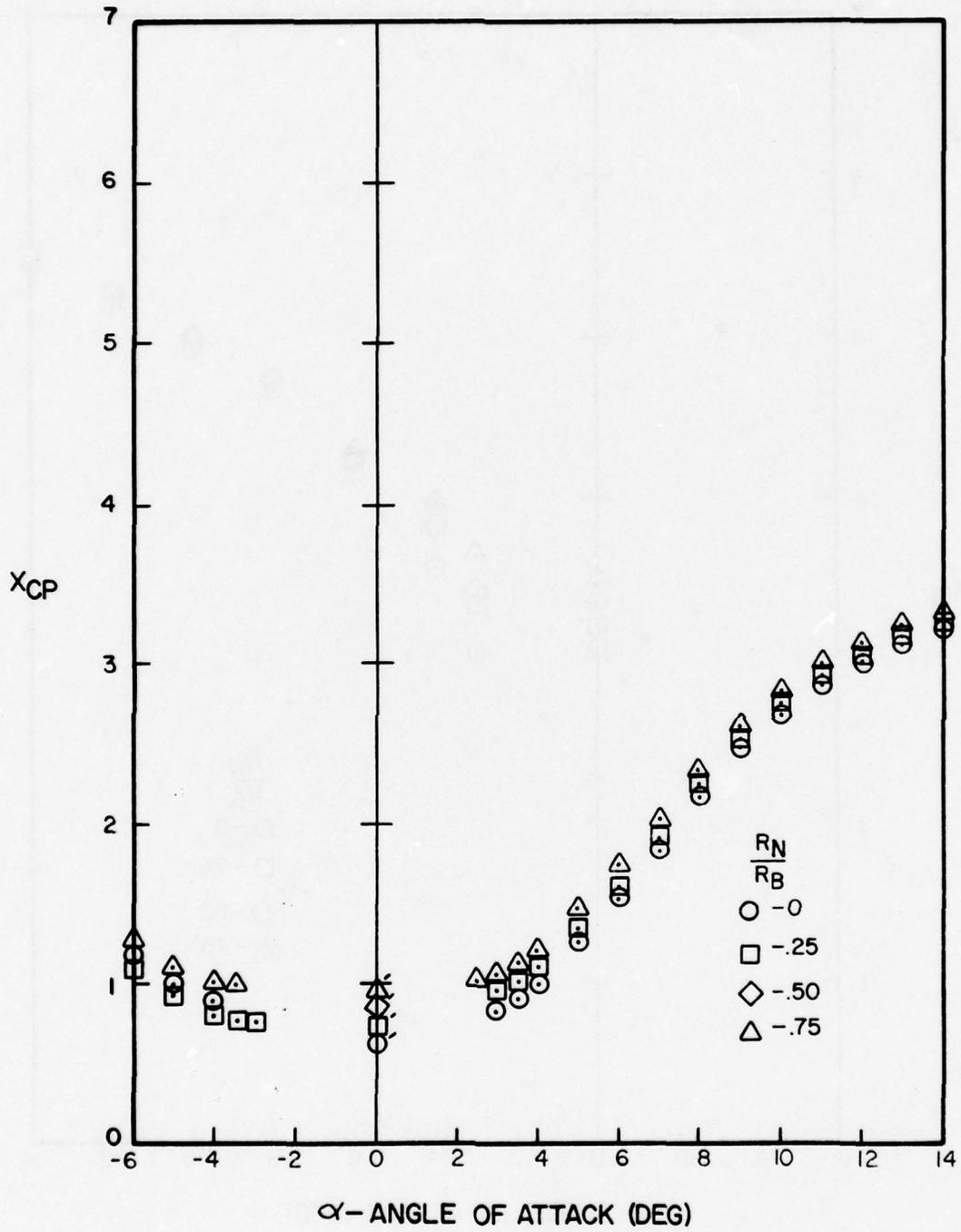
Figure A-104. Center of Pressure Versus Angle of Attack for  $l_N/d = 2$ ,  $l_A/d = 6$ ,  $M = 1.5$
