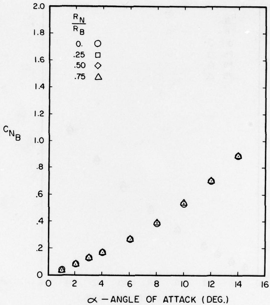
Figure A-37. Normal Force Coefficient Versus Angle of Attack for  $l_N/d = 4$ ,  $l_A/d = 6$ ,  $M = 1.0$
