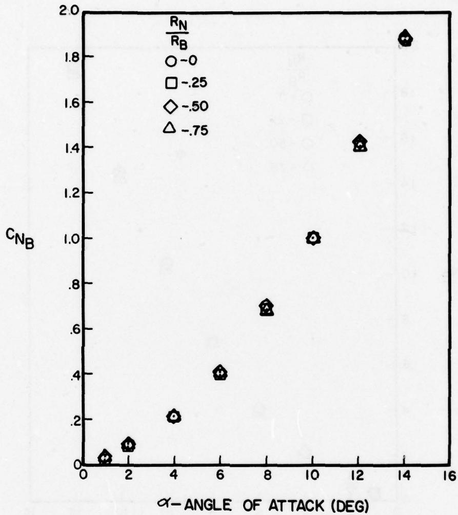
Figure A-63. Normal Force Coefficient Versus Angle of Attack for  $l_N/d = 3$ ,  $l_A/d = 10$ ,  $M = 2.0$
