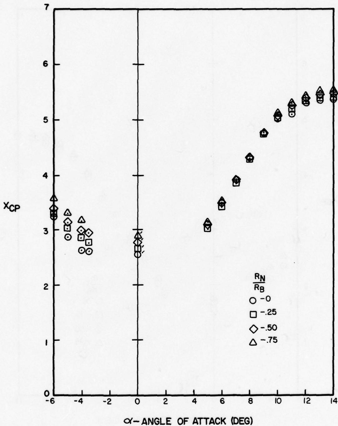
Figure A-109. Center of Pressure Versus Angle of Attack for  $l_N/d = 4$ ,  $l_A/d = 8$ ,  $M = 1.5$
