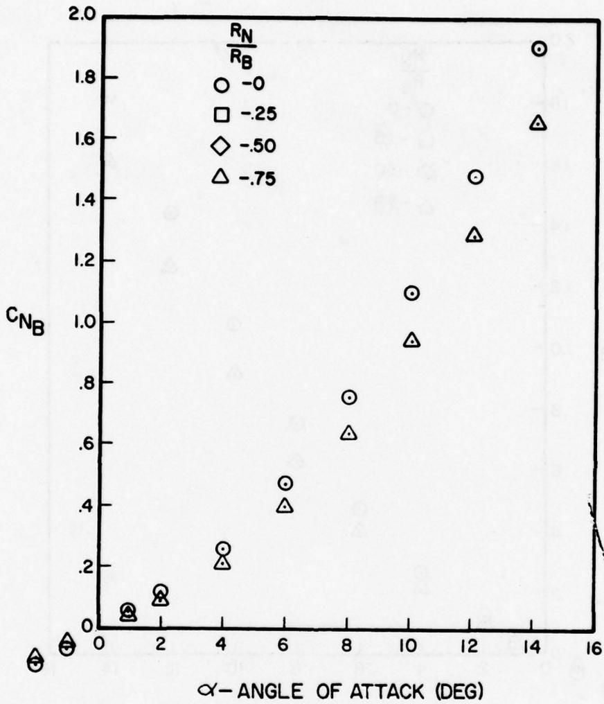
Figure A-70. Normal Force Coefficient Versus Angle of Attack for  $l_N/d = 4$ ,  $l_A/d = 8$ ,  $M = 3.0$
