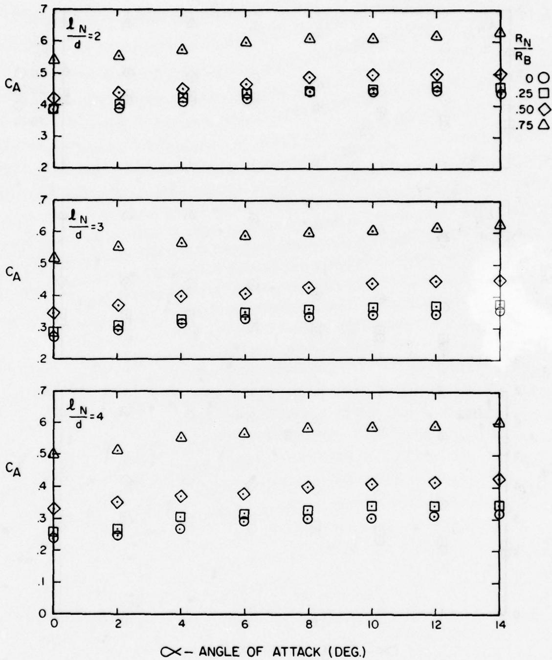
Figure A-11. Axial Force Coefficient Versus Angle of Attack for  $\frac{l_A}{d} = 10$ ,  $M = 1.5$
