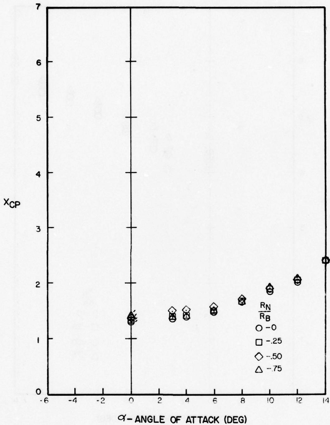
Figure A-98. Center of Pressure Versus Angle of Attack for  $l_N/d = 2$ ,  $l_A/d = 6$ ,  $M = 1.2$
