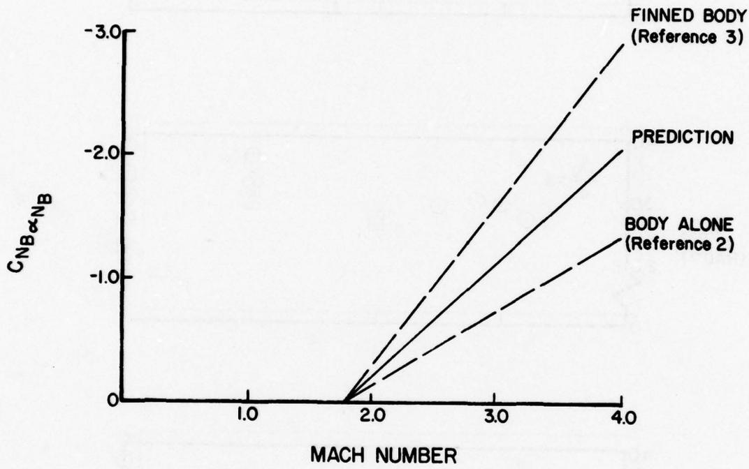
Figure 8. Change in Normal Force Slope Coefficient Due to Nose Bluntness
