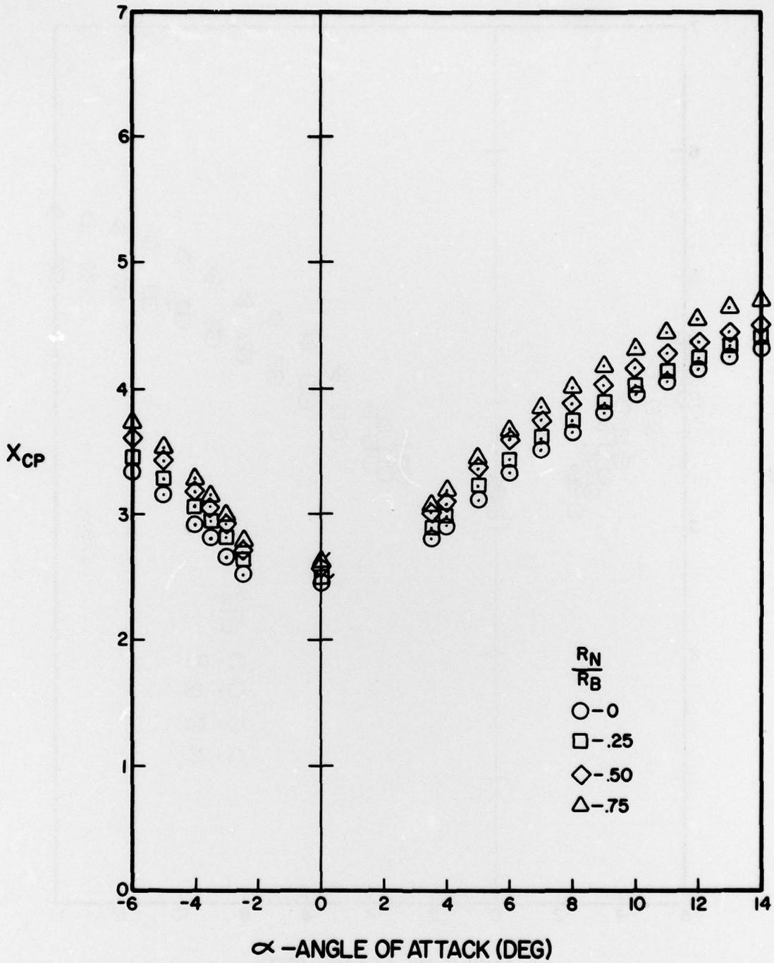
Figure A-131. Center of Pressure Versus Angle of Attack for  $l_N/d = 2$ ,  $l_A/d = 8$ ,  $M = 4.0$
