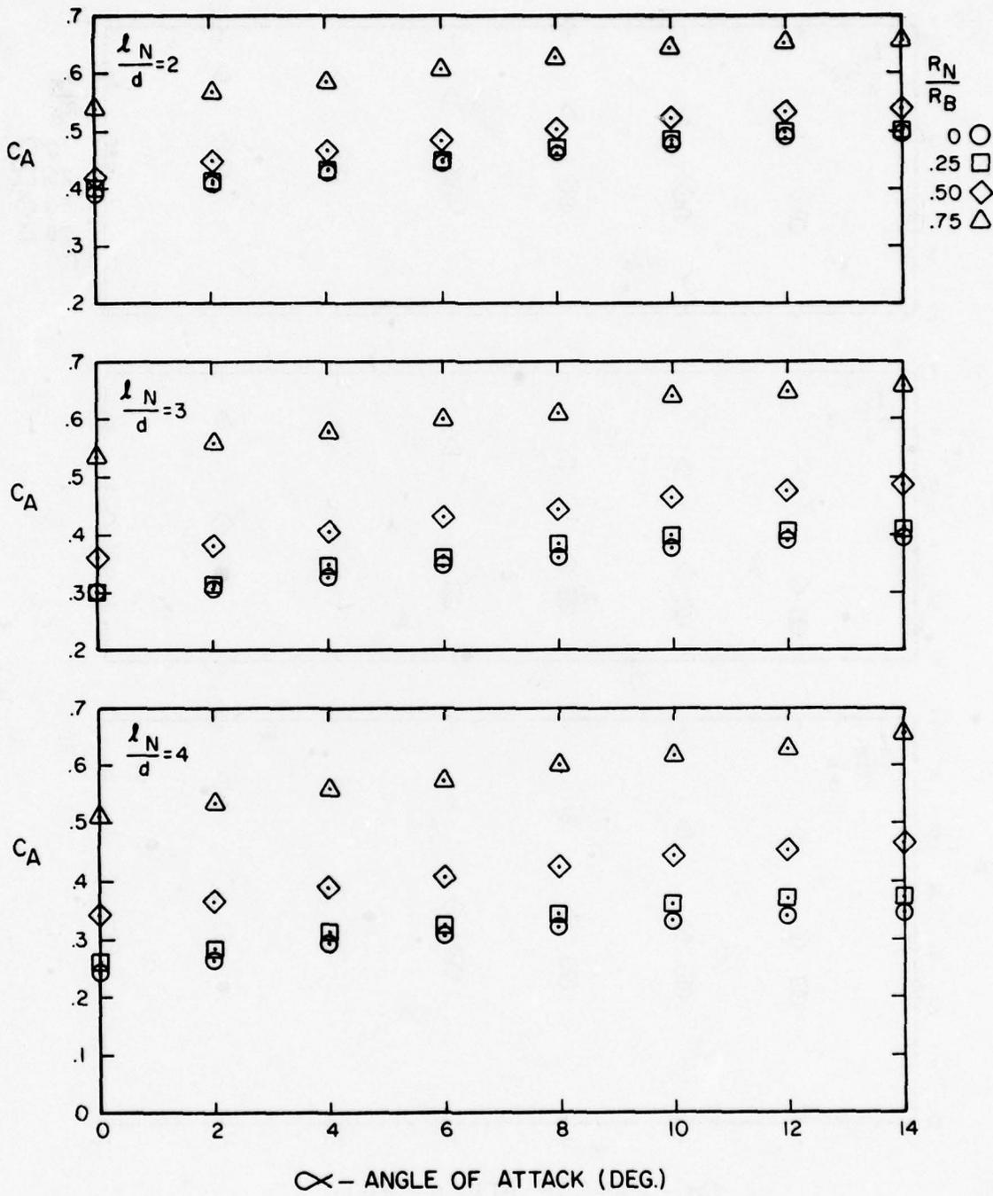
Figure A-10. Axial Force Coefficient Versus Angle of Attack for  $\frac{l_A}{d} = 6$ ,  $M = 1.5$
