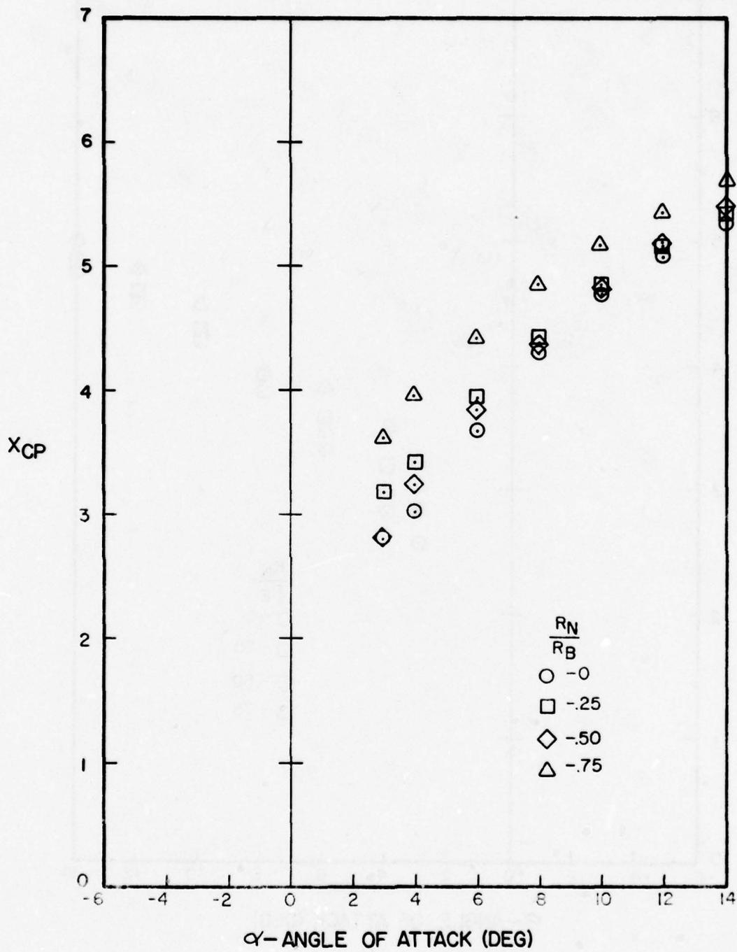
Figure A-82. Center of Pressure Versus Angle of Attack for  $l_N/d = 4$ ,  $l_A/d = 6$ ,  $M = 0.6$
