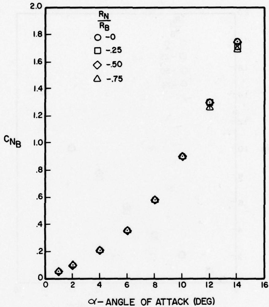
Figure A-55. Normal Force Coefficient Versus Angle of Attack for  $l_N/d = 4$ ,  $l_A/d = 10$ ,  $M = 1.5$
