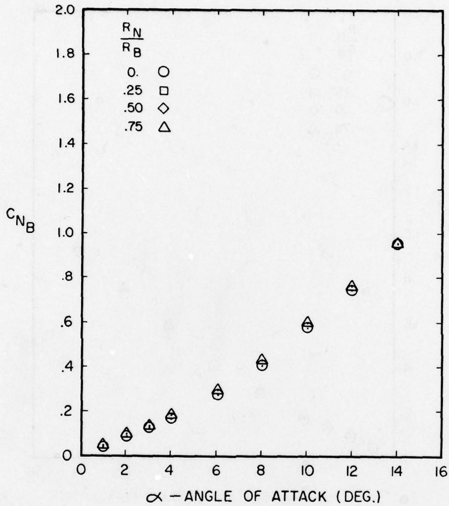
Figure A-28. Normal Force Coefficient Versus Angle of Attack for  $l_N/d = 4$ ,  $l_A/d = 10$ ,  $M = 0.6$
