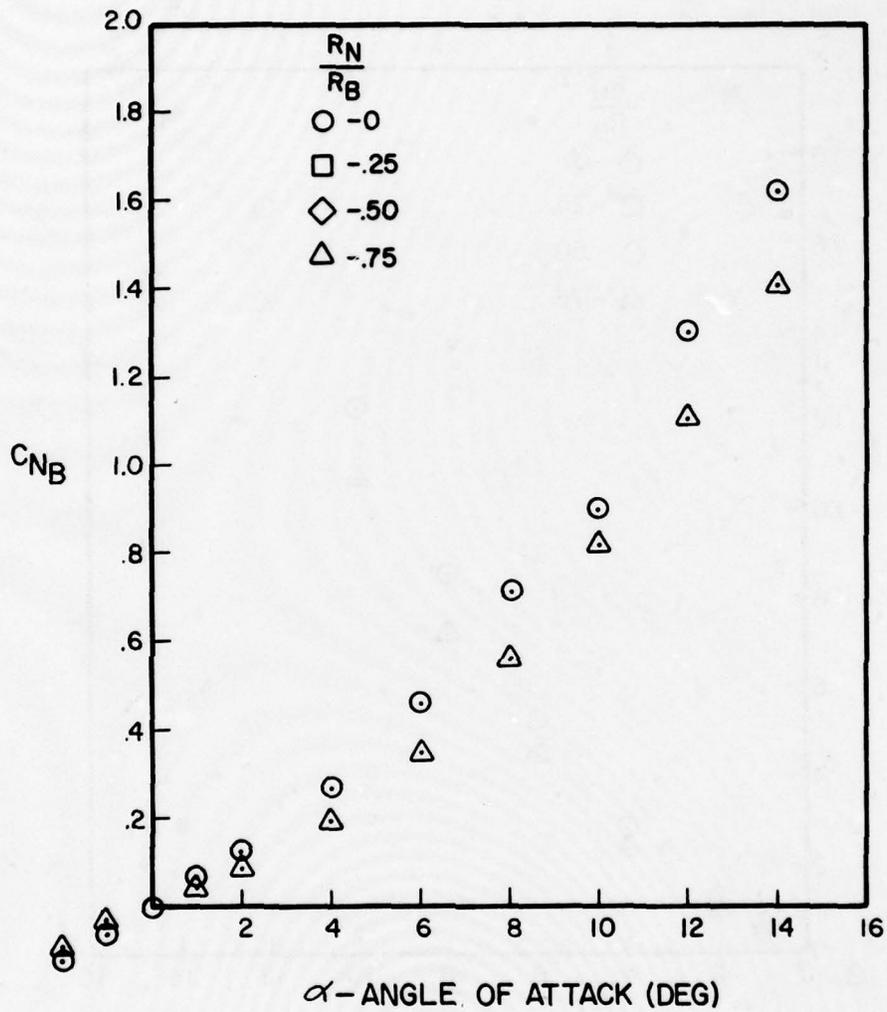
Figure A-74. Normal Force Coefficient Versus Angle of Attack for  $l_N/d = 2$ ,  $l_A/d = 8$ ,  $M = 4.0$
