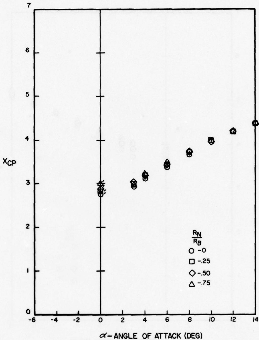
Figure A-95. Center of Pressure Versus Angle of Attack for  $l_N/d = 2$ ,  $l_A/d = 10$ ,  $M = 1.0$
