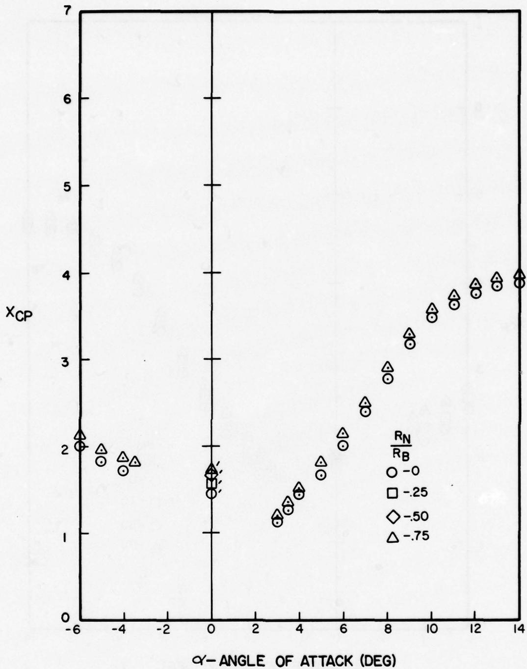
Figure A-107. Center of Pressure Versus Angle of Attack for  $l_N/d = 2$ ,  $l_A/d = 8$ ,  $M = 1.5$
