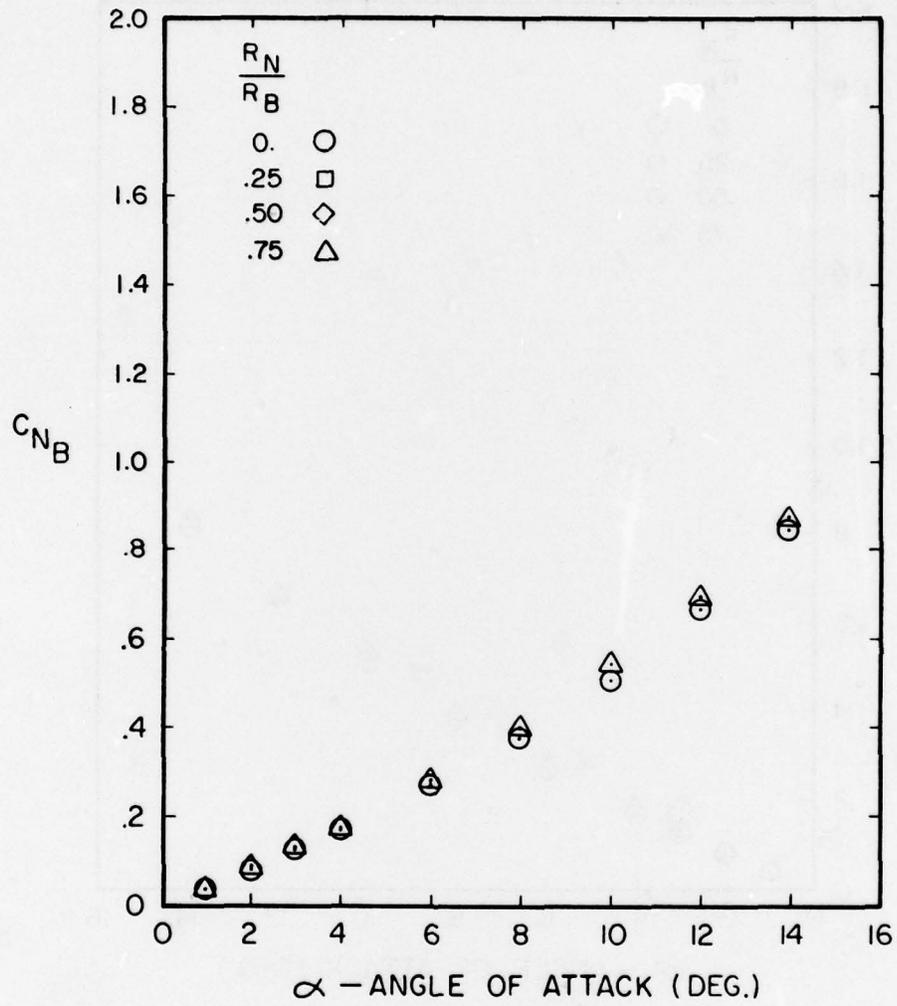
Figure A-36. Normal Force Coefficient Versus Angle of Attack for  $l_N/d = 3$ ,  $l_A/d = 6$ ,  $M = 1.0$
