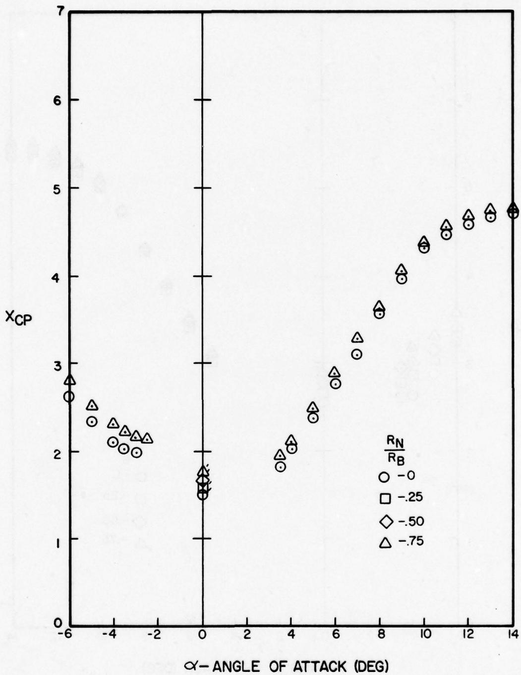
Figure A-110. Center of Pressure Versus Angle of Attack for  $l_N/d = 2$ ,  $l_A/d = 10$ ,  $M = 1.5$
