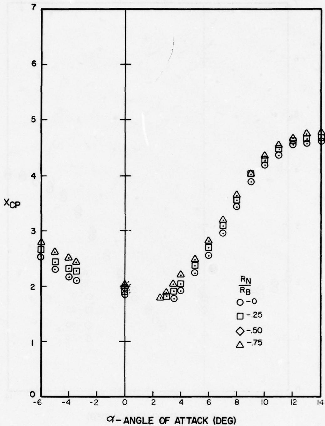
Figure A-108. Center of Pressure Versus Angle of Attack for  $l_N/d = 3$ ,  $l_A/d = 8$ ,  $M = 1.5$
