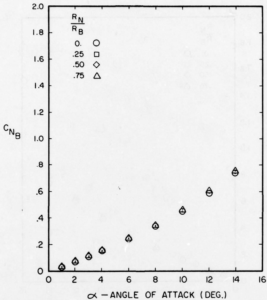
Figure A-29. Normal Force Coefficient Versus Angle of Attack for  $l_N/d = 2$ ,  $l_A/d = 6$ ,  $M = 0.8$
