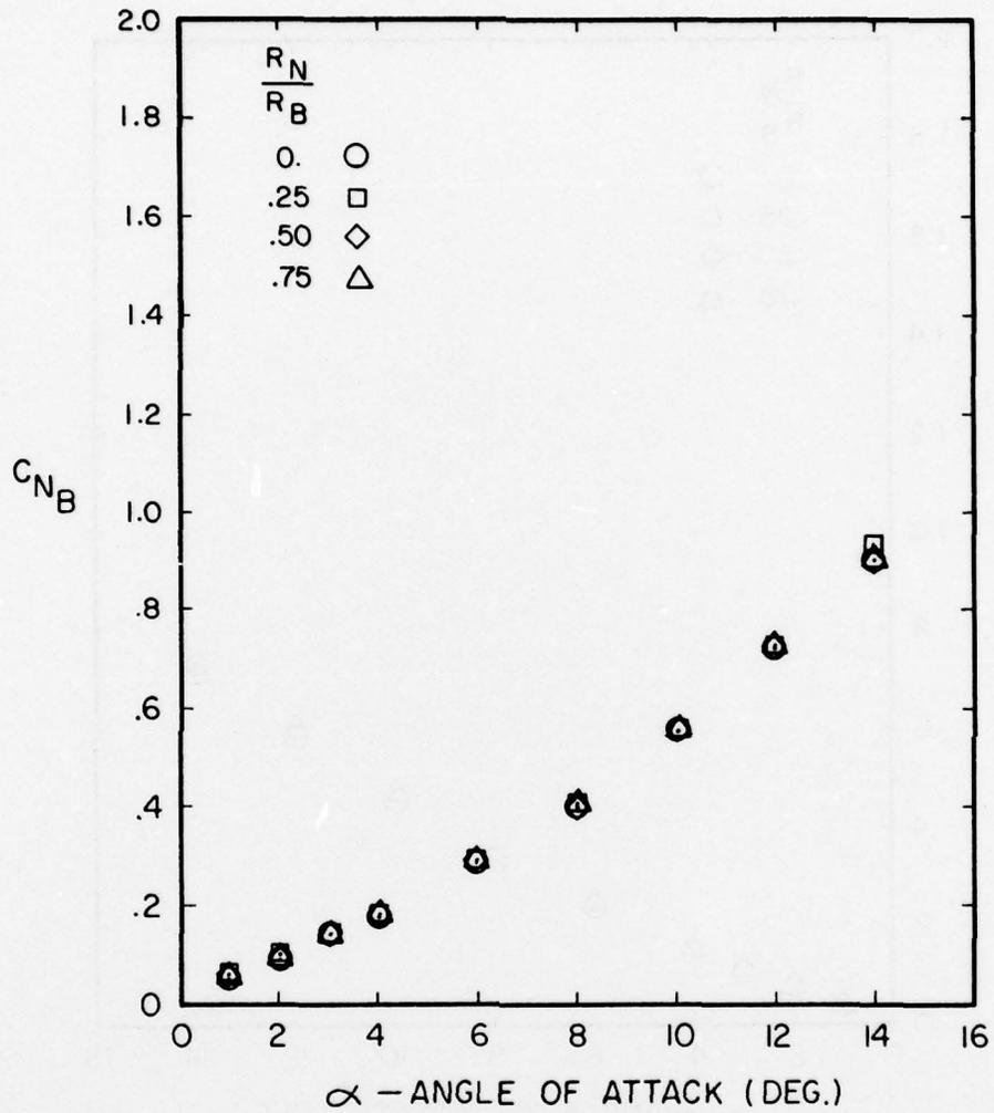
Figure A-26. Normal Force Coefficient Versus Angle of Attack for  $l_N/d = 2$ ,  $l_A/d = 10$ ,  $M = 0.6$
