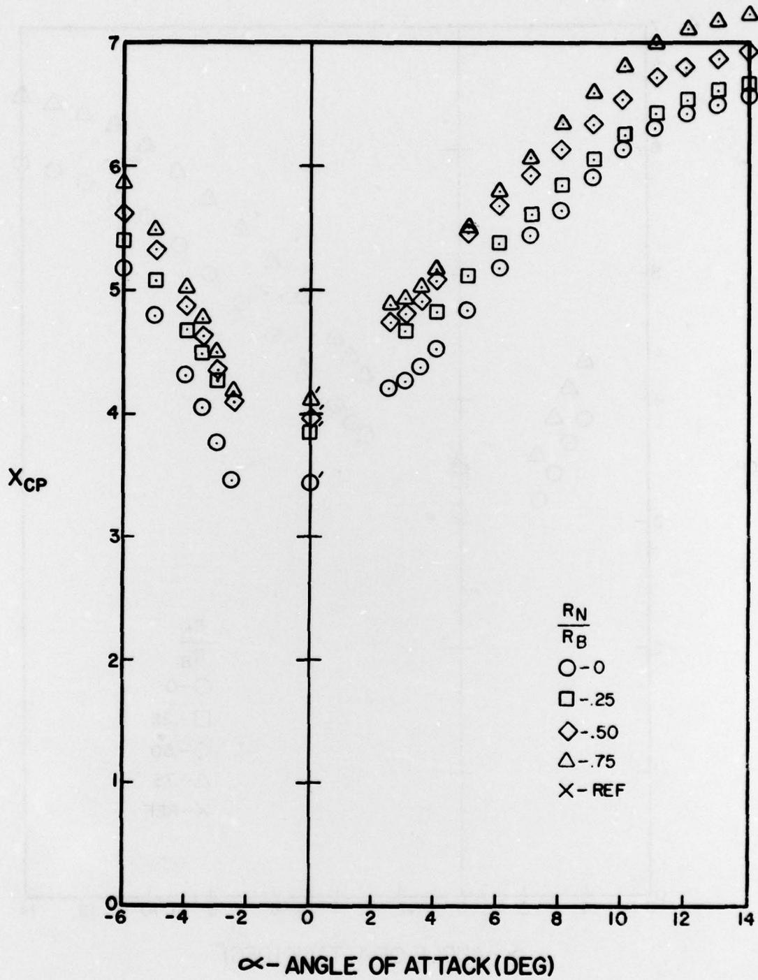
Figure A-136. Center of Pressure Versus Angle of Attack for  $l_N/d = 4$ ,  $l_A/d = 10$ ,  $M = 4.0$
