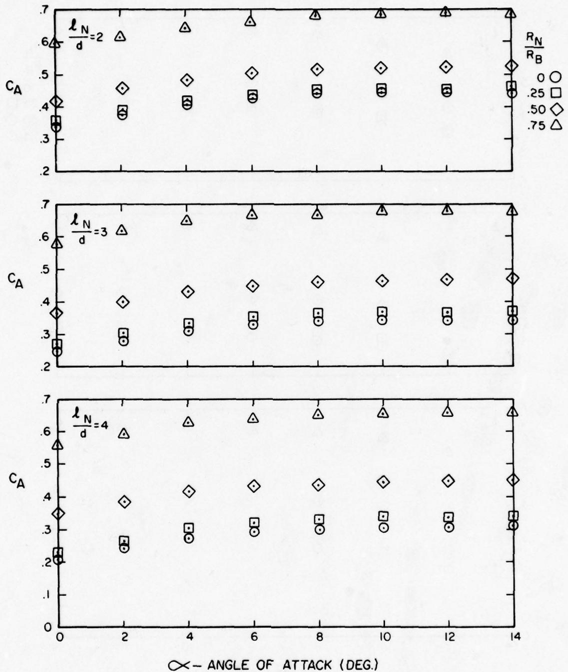
Figure A-14. Axial Force Coefficient Versus Angle of Attack for  $l_A/d = 10$ ,  $M = 2.0$
