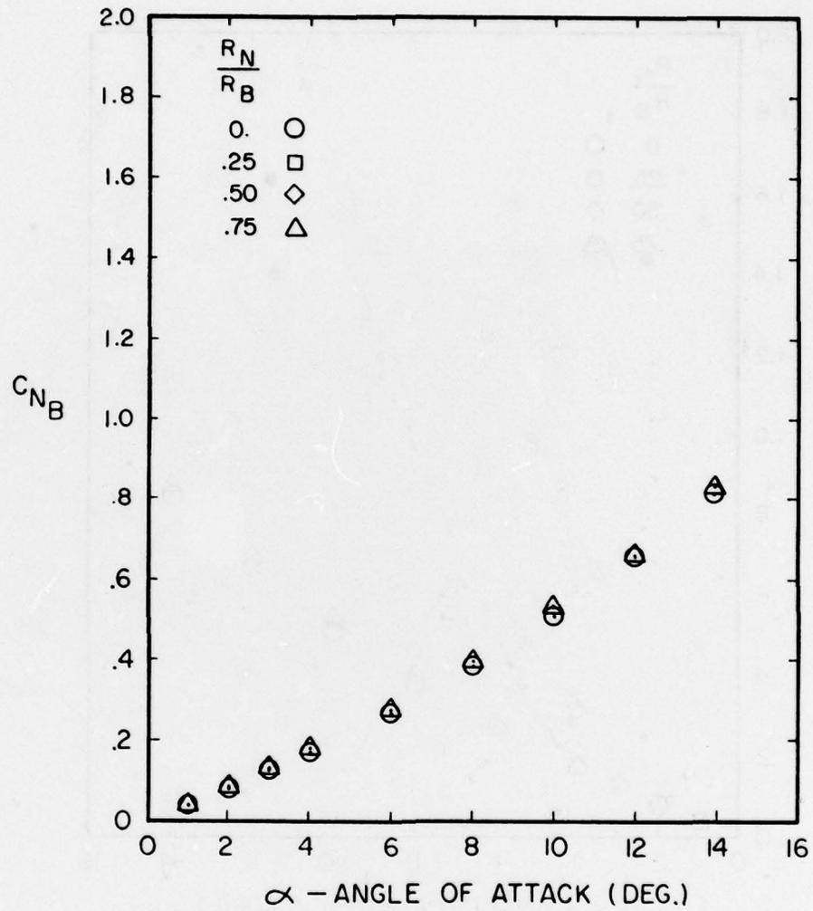
Figure A-35. Normal Force Coefficient Versus Angle of Attack for  $l_N/d = 2$ ,  $l_A/d = 6$ ,  $M = 1.0$
