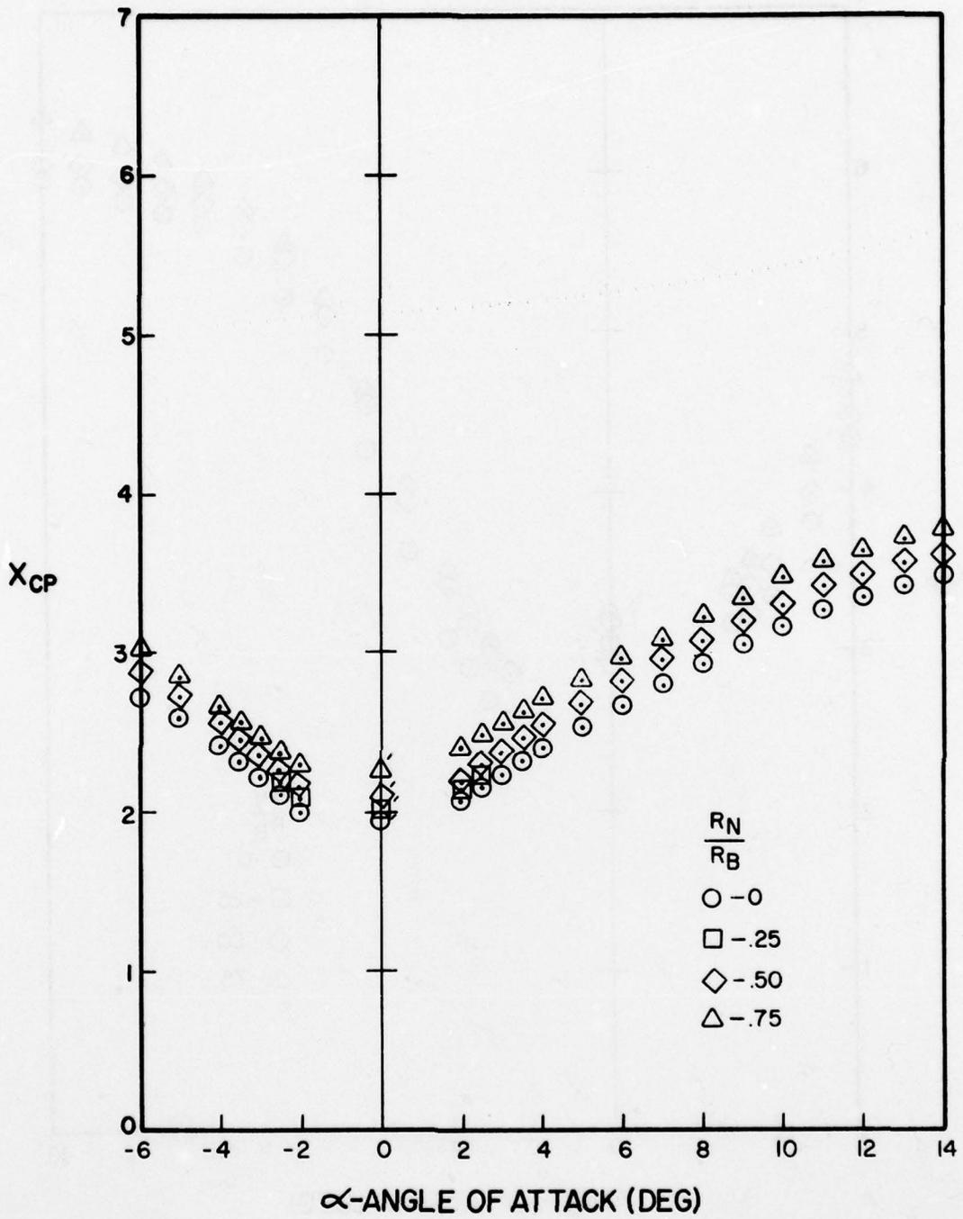
Figure A-122. Center of Pressure Versus Angle of Attack for  $l_N/d = 2$ ,  $l_A/d = 6$ ,  $M = 3.0$
