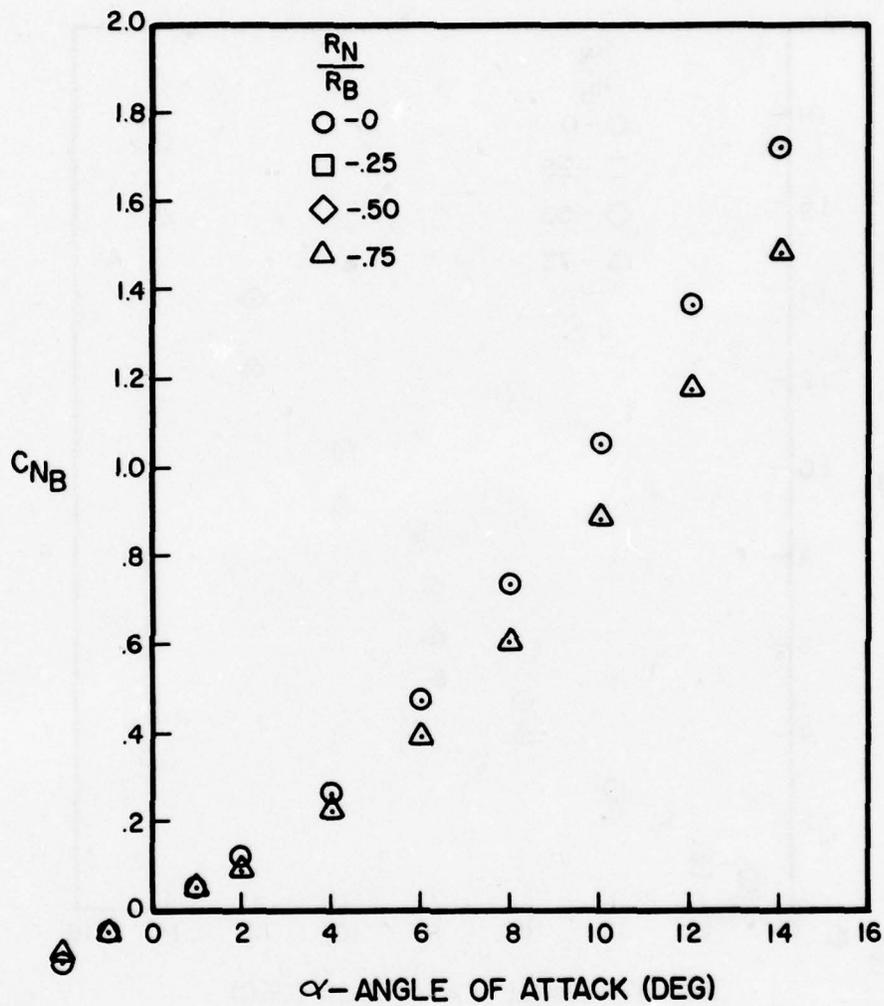
Figure A-67. Normal Force Coefficient Versus Angle of Attack for  $l_N/d = 4$ ,  $l_A/d = 6$ ,  $M = 3.0$
