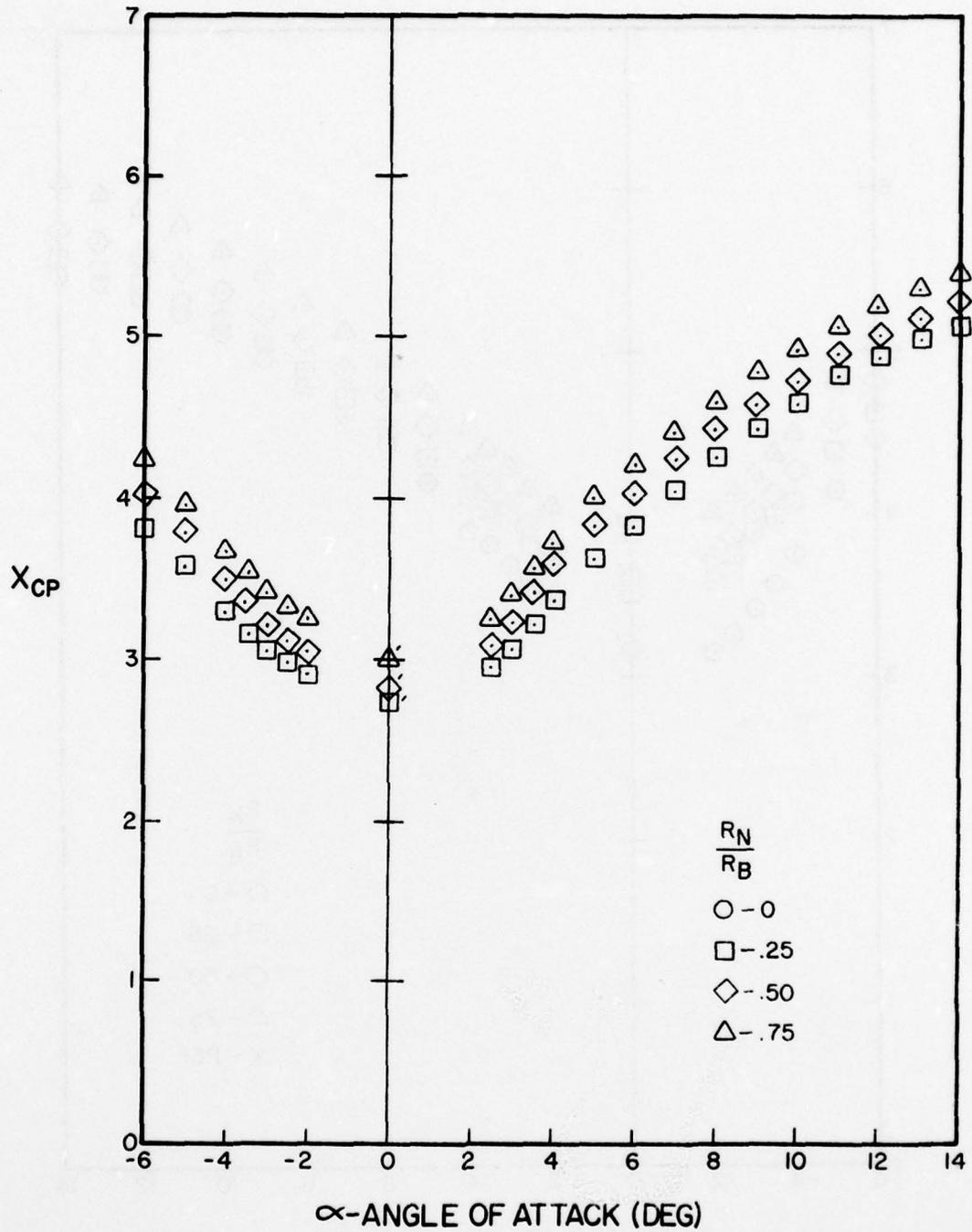
Figure A-128. Center of Pressure Versus Angle of Attack for  $l_N/d = 2$ ,  $l_A/d = 10$ ,  $M = 3.0$
