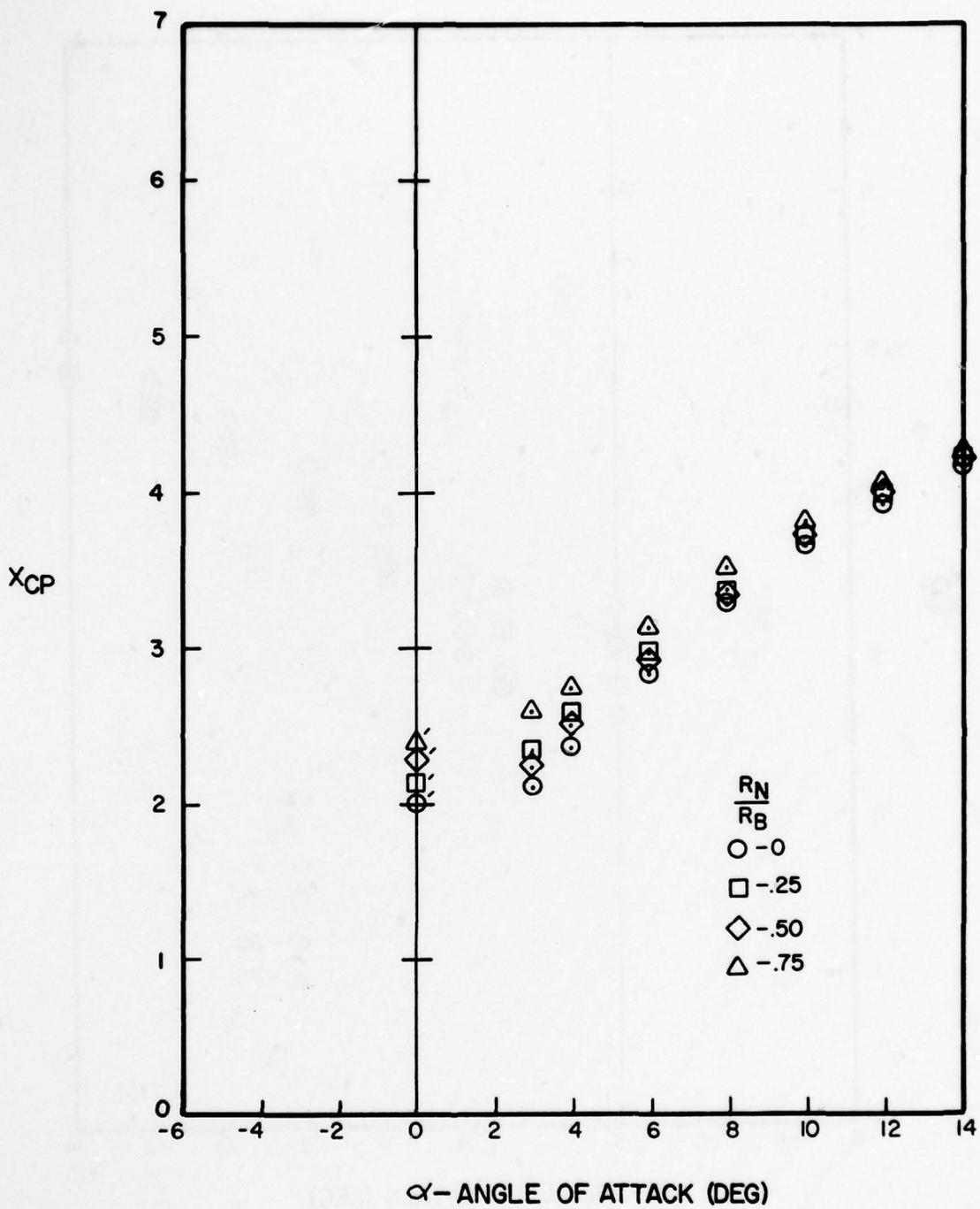
Figure A-89. Center of Pressure Versus Angle of Attack for  $l_N/d = 2$ ,  $l_A/d = 10$ ,  $M = 0.8$
