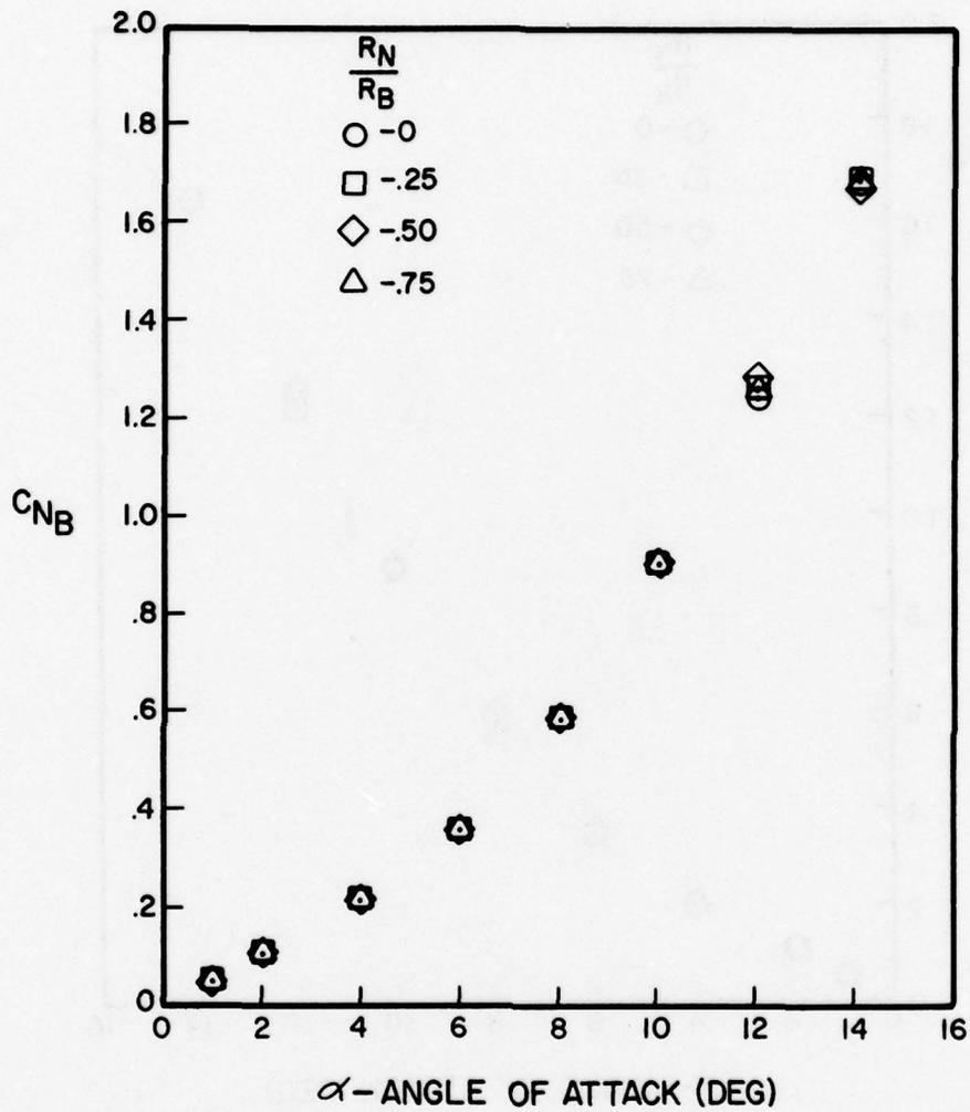
Figure A-54. Normal Force Coefficient Versus Angle of Attack for  $l_N/d = 3$ ,  $l_A/d = 10$ ,  $M = 1.5$
