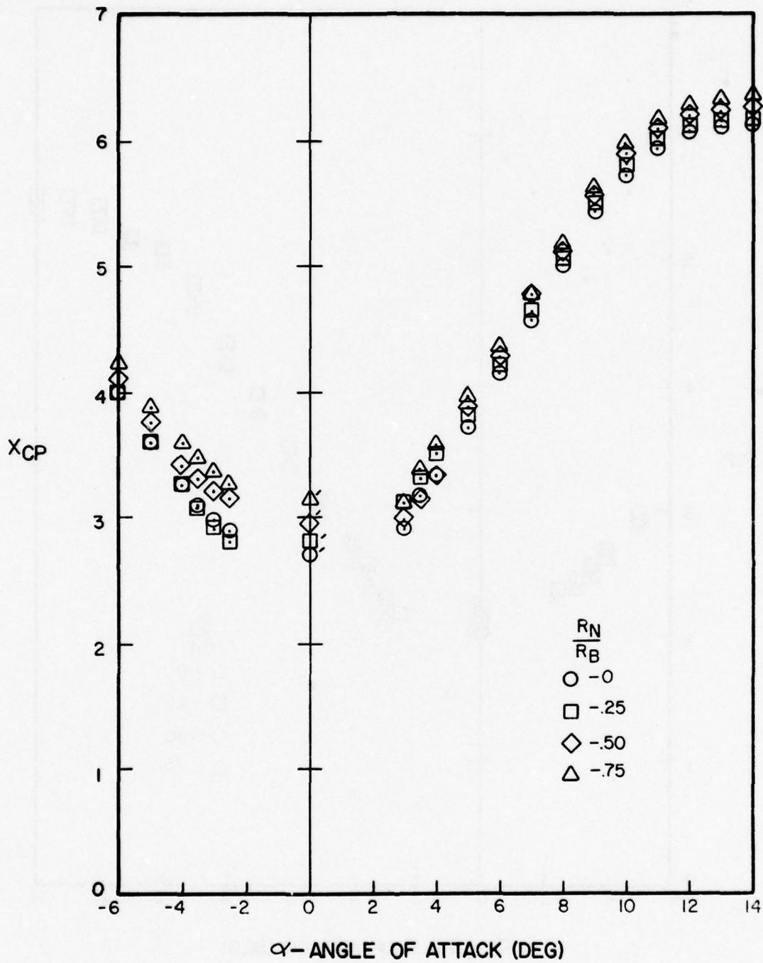
Figure A-112. Center of Pressure Versus Angle of Attack for  $l_N/d = 4$ ,  $l_A/d = 10$ ,  $M = 1.5$
