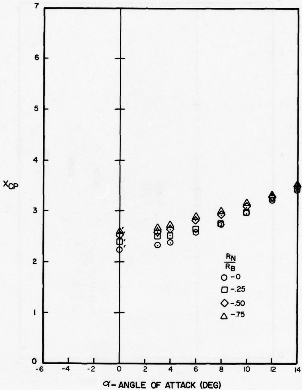
Figure A-93. Center of Pressure Versus Angle of Attack for  $l_N/d = 3$ ,  $l_A/d = 6$ ,  $M = 1.0$
