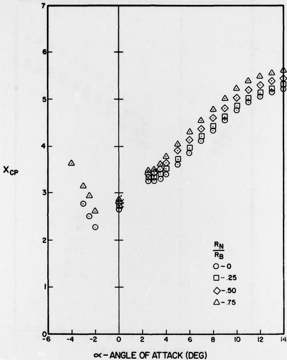
Figure A-134. Center of Pressure Versus Angle of Attack for  $l_N/d = 2$ ,  $l_A/d = 10$ ,  $M = 4.0$
