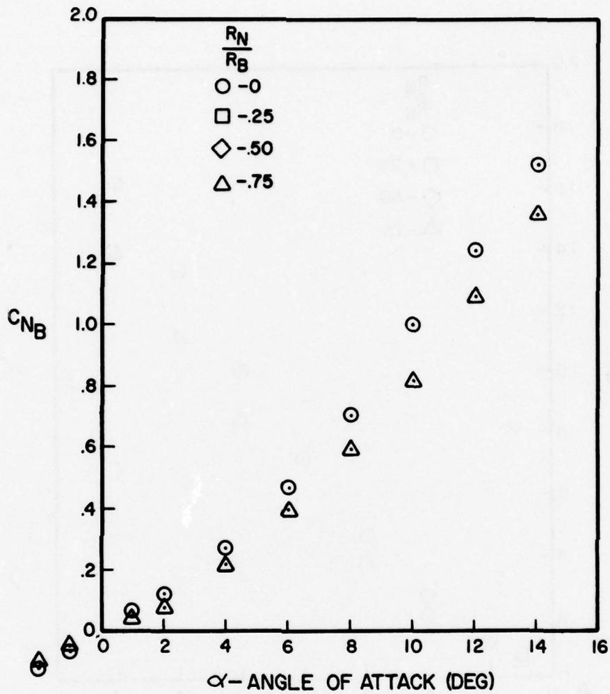
Figure A-65. Normal Force Coefficient Versus Angle of Attack for  $l_N/d = 2$ ,  $l_A/d = 6$ ,  $M = 3.0$
