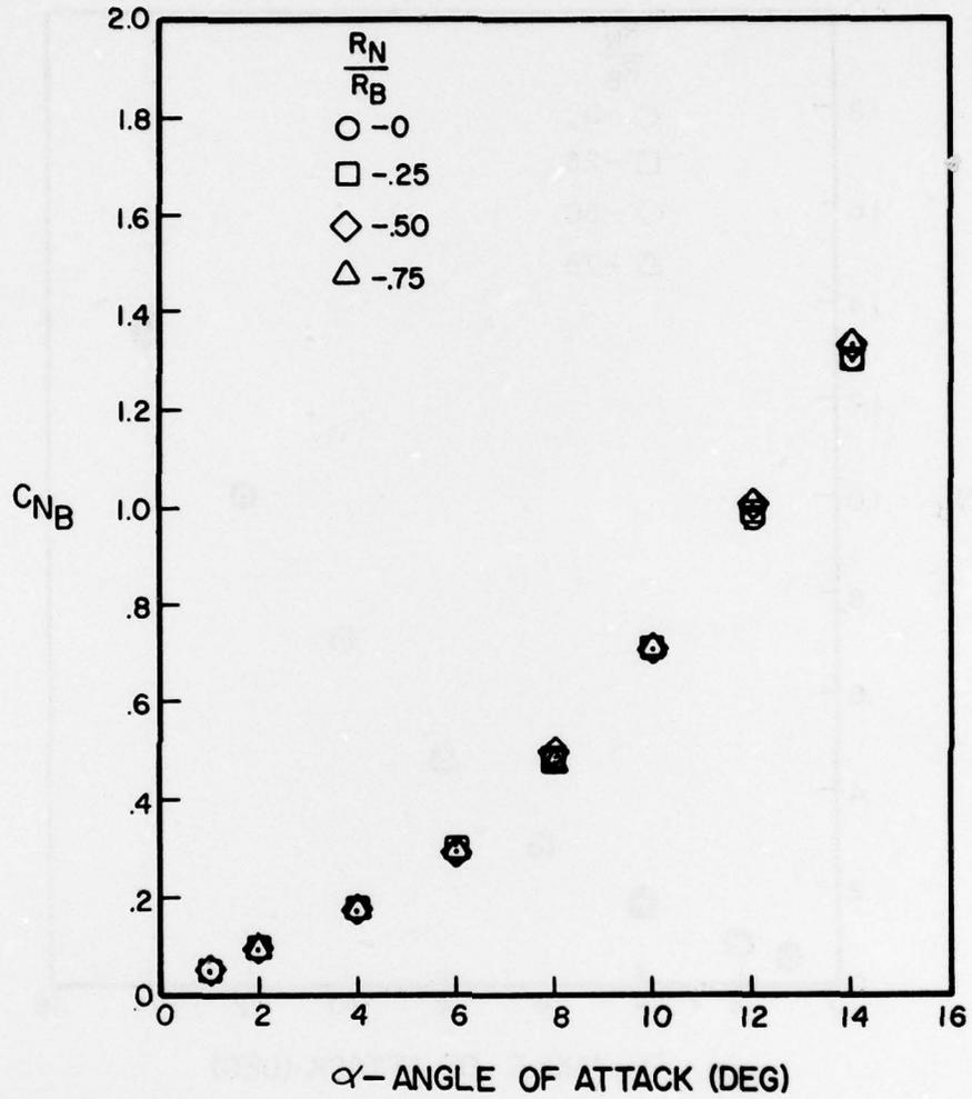
Figure A-47. Normal Force Coefficient Versus Angle of Attack for  $l_N/d = 2$ ,  $l_A/d = 6$ ,  $M = 1.5$
