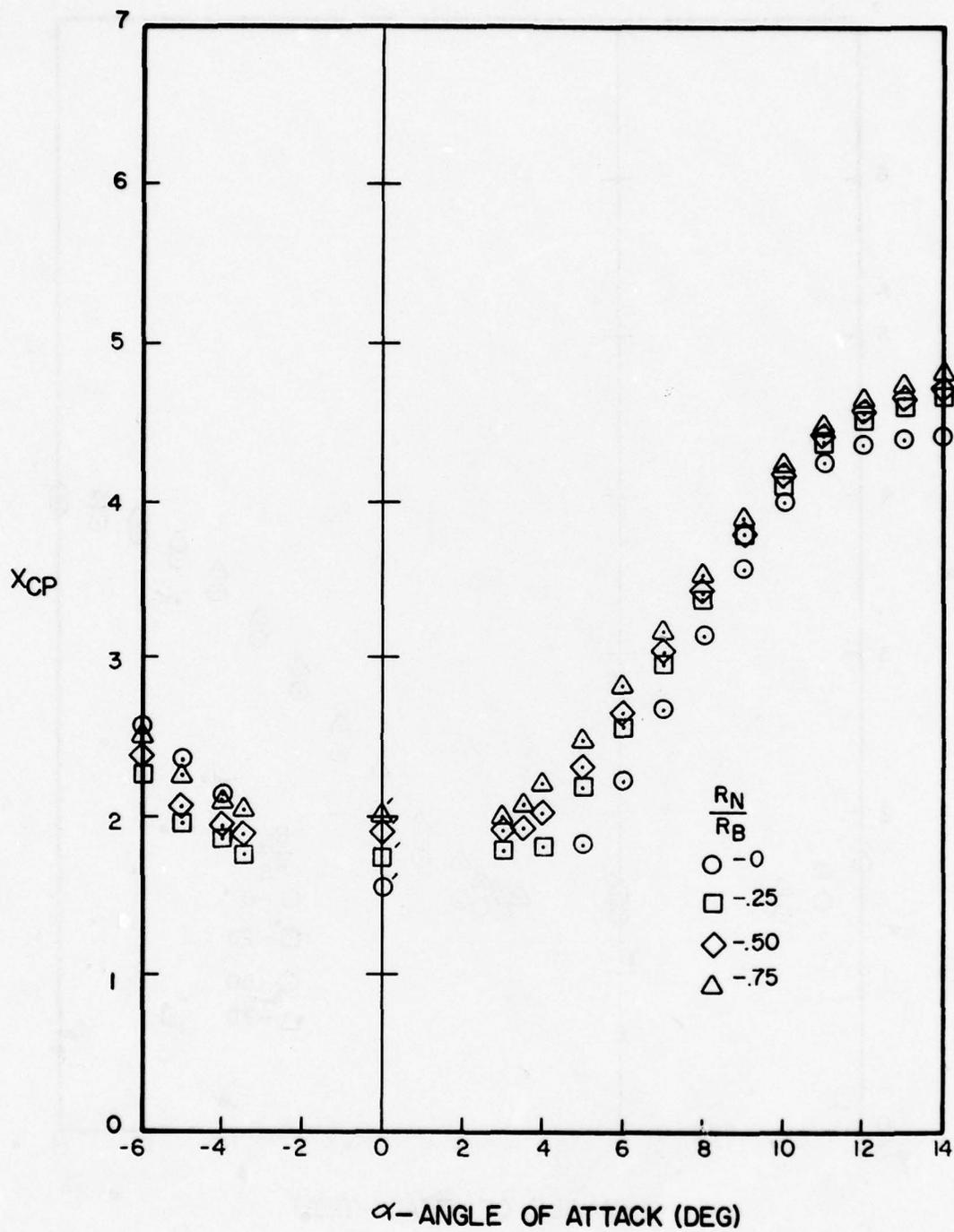
Figure A-106. Center of Pressure Versus Angle of Attack for  $l_N/d = 4$ ,  $l_A/d = 6$ ,  $M = 1.5$
