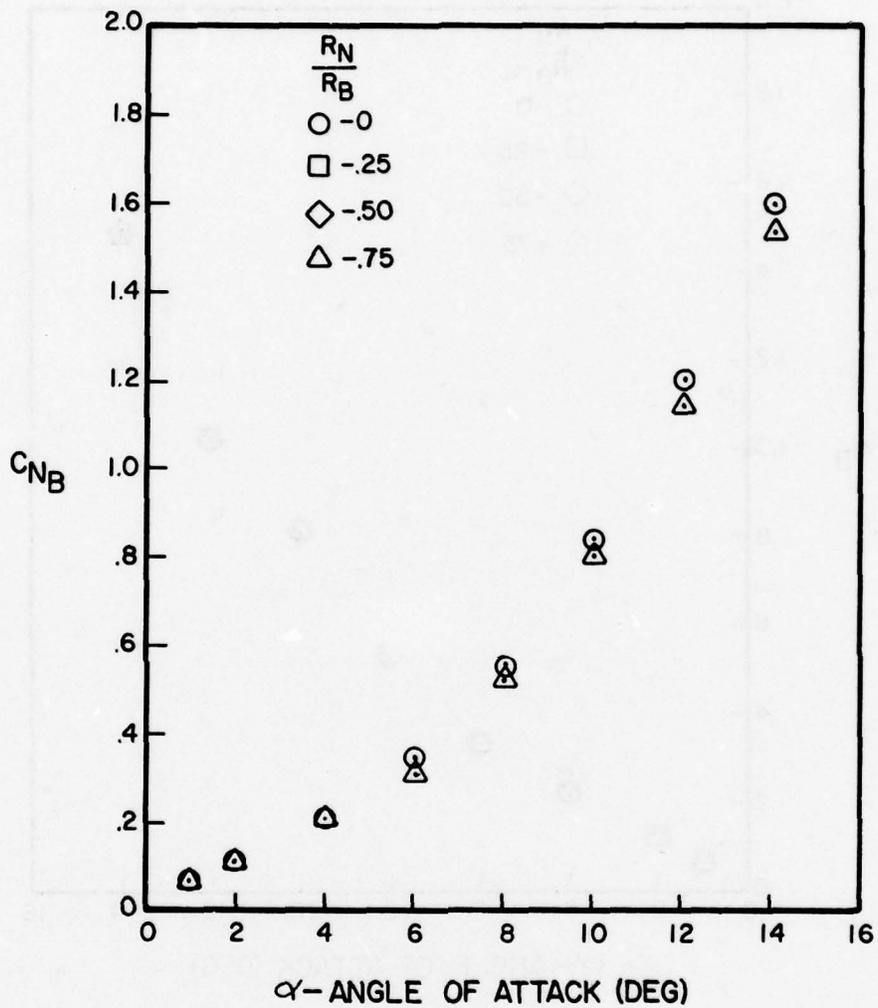
Figure A-52. Normal Force Coefficient Versus Angle of Attack for  $l_N/d = 4$ ,  $l_A/d = 8$ ,  $M = 1.5$
