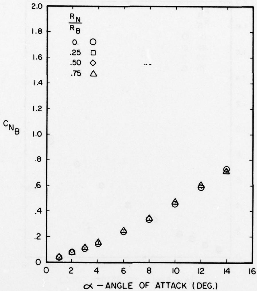
Figure A-25. Normal Force Coefficient Versus Angle of Attack for  $l_N/d = 4$ ,  $l_A/d = 6$ ,  $M = 0.6$
