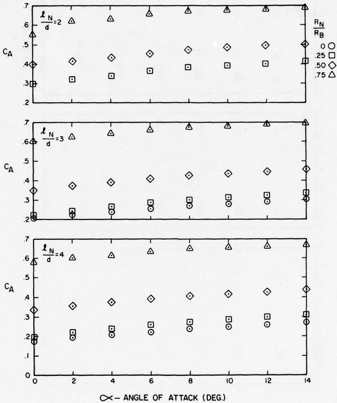
Figure A-17. Axial Force Coefficient Versus Angle of Attack for  $\frac{l_A}{d} = 10$ ,  $M = 3.0$
