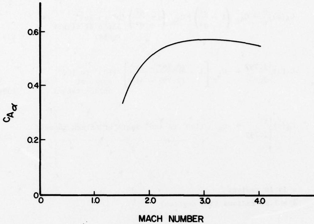
Figure 4A.  $C_{A\alpha}$  as Function of Mach Number
