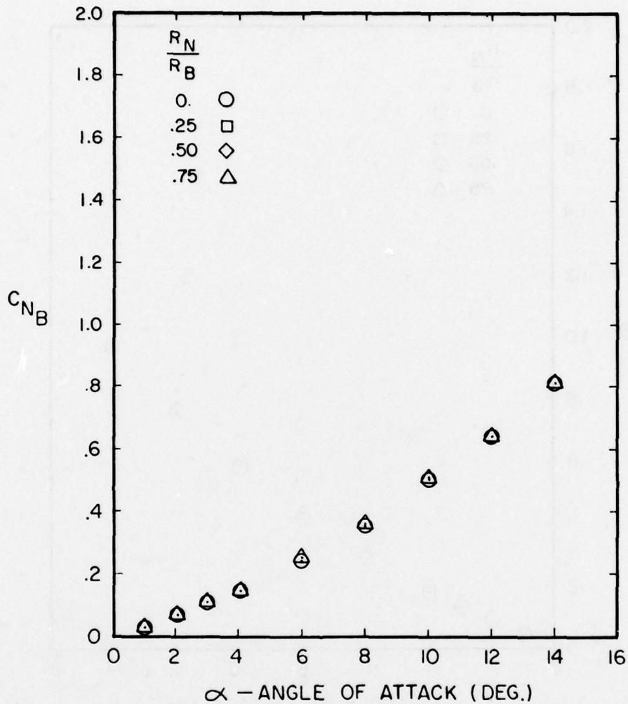
Figure A-31. Normal Force Coefficient Versus Angle of Attack for  $l_N/d = 4$ ,  $l_A/d = 6$ ,  $M = 0.8$
