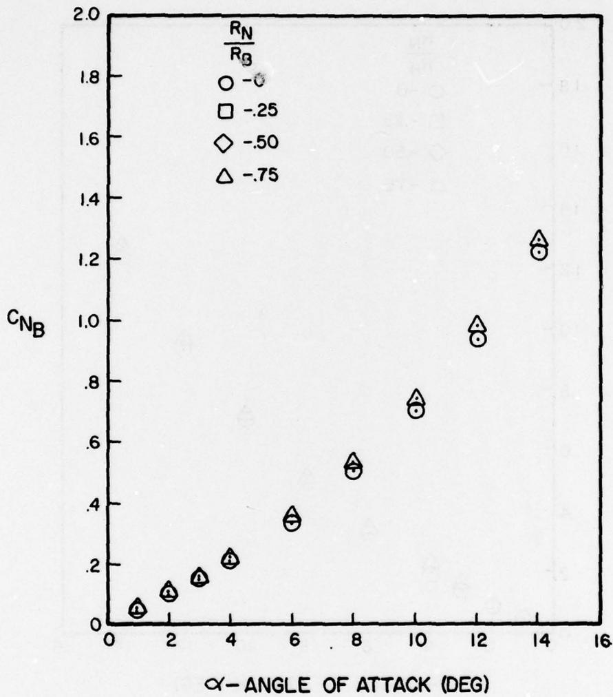
Figure A-45. Normal Force Coefficient Versus Angle of Attack for  $l_N/d = 3$ ,  $l_A/d = 10$ ,  $M = 1.2$
