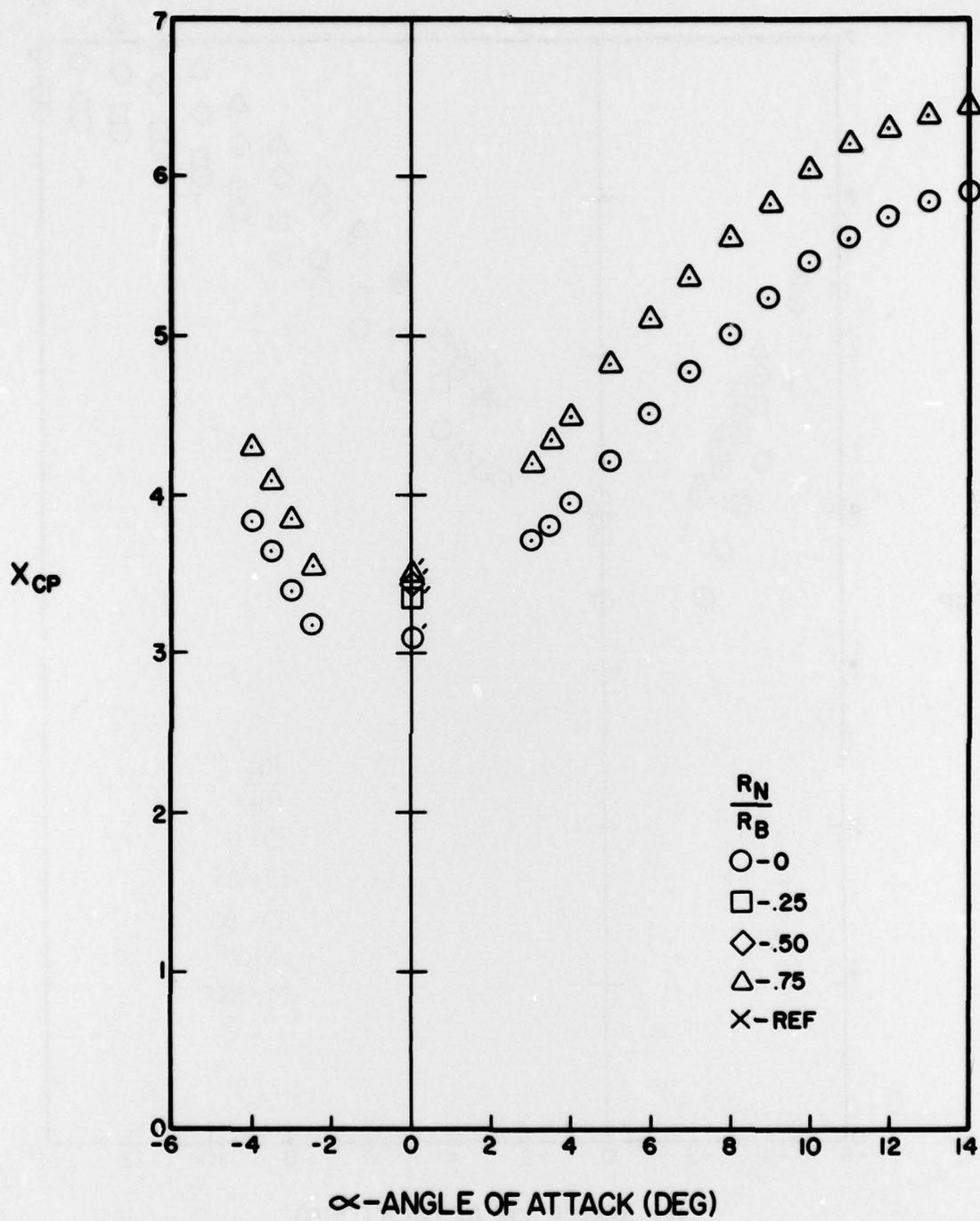
Figure A-135. Center of Pressure Versus Angle of Attack for  $l_N/d = 3$ ,  $l_A/d = 10$ ,  $M = 4.0$
