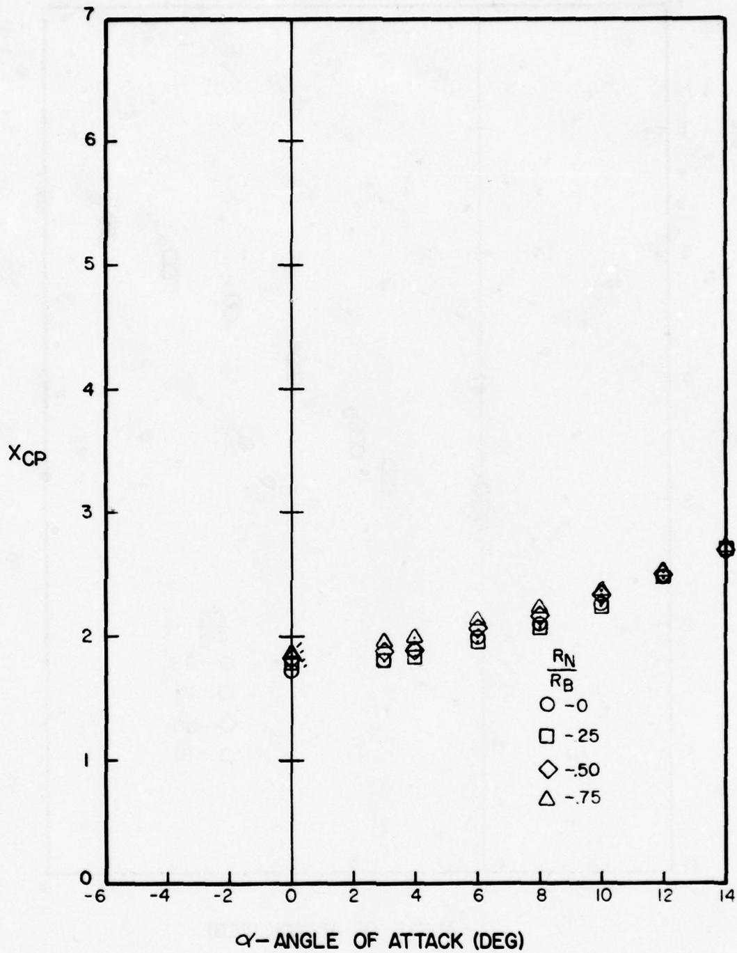
Figure A-92. Center of Pressure Versus Angle of Attack for  $l_N/d = 2$ ,  $l_A/d = 6$ ,  $M = 1.0$
