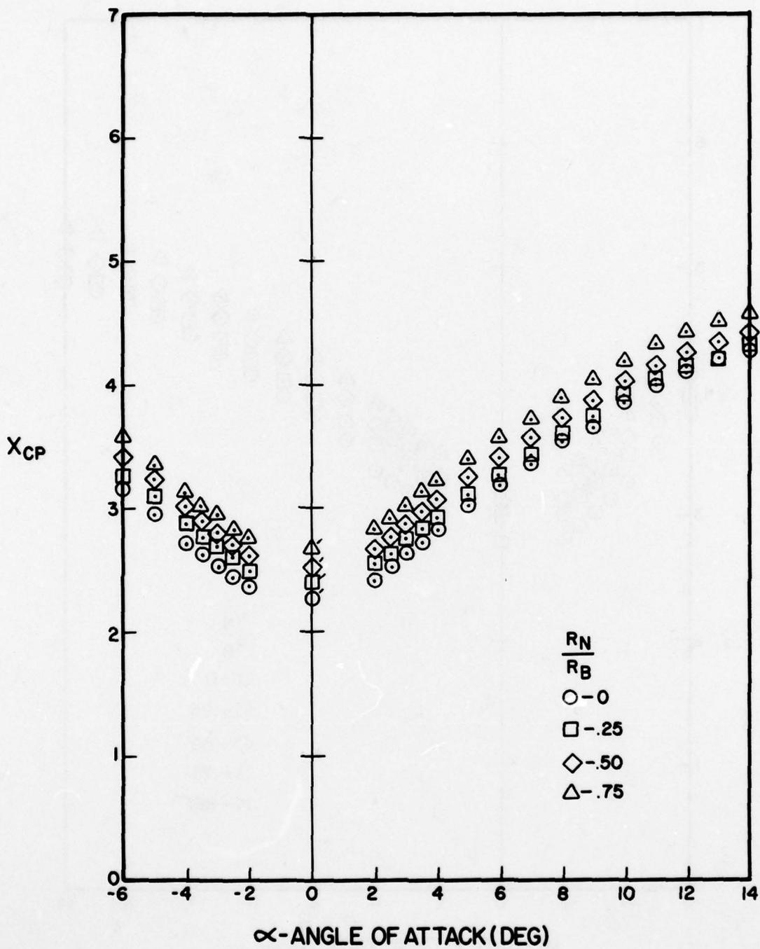
Figure A-125. Center of Pressure Versus Angle of Attack for  $l_N/d = 2$ ,  $l_A/d = 8$ ,  $M = 3.0$
