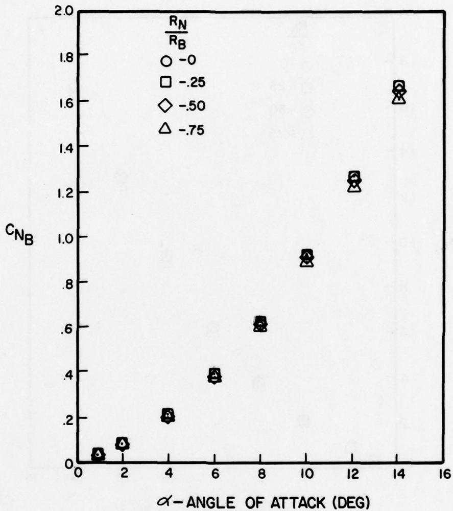
Figure A-59. Normal Force Coefficient Versus Angle of Attack for  $l_N/d = 2$ ,  $l_A/d = 8$ ,  $M = 2.0$
