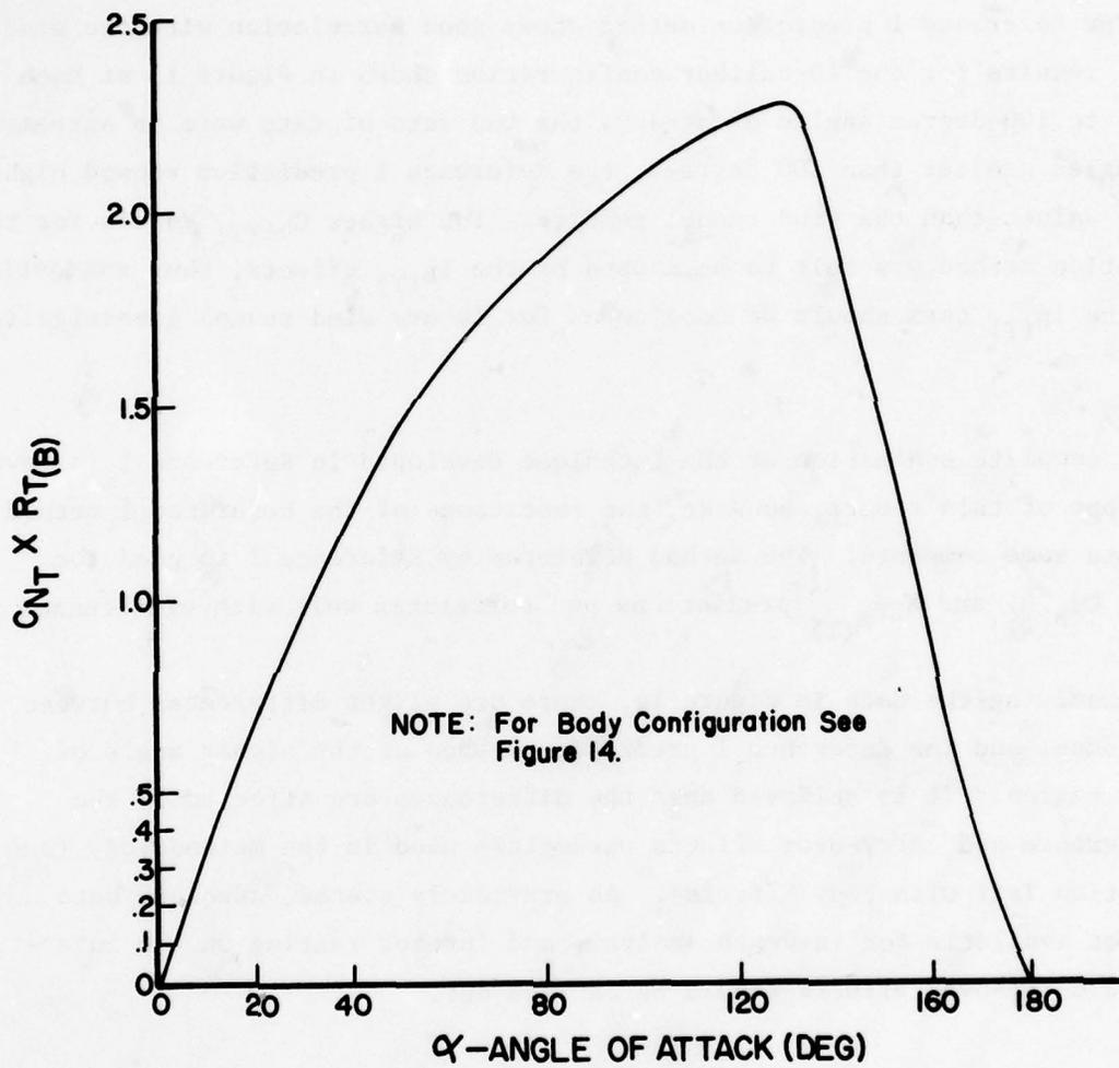
Figure 17.  $C_{NT} \times R_{T(B)}$  Versus Angle of Attack for a 10-Caliber Finned Body Using Prediction Method (Reference 1)
