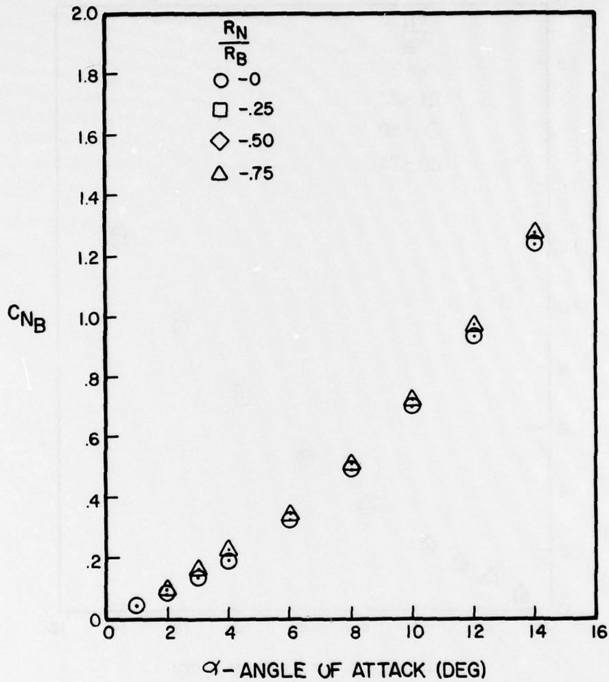
Figure A-46. Normal Force Coefficient Versus Angle of Attack for  $l_N/d = 4$ ,  $l_A/d = 10$ ,  $M = 1.2$
