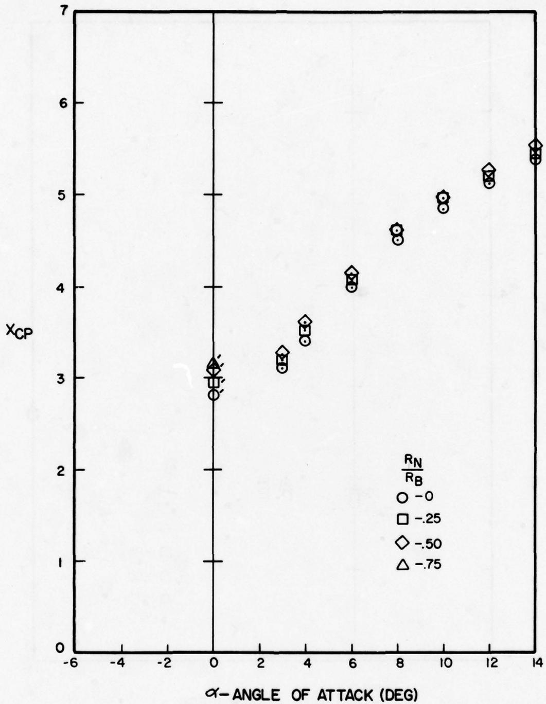
Figure A-91. Center of Pressure Versus Angle of Attack for  $l_N/d = 4$ ,  $l_A/d = 10$ ,  $M = 0.8$
