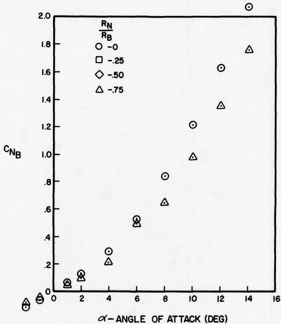
Figure A-79. Normal Force Coefficient Versus Angle of Attack for  $l_N/d = 4$ ,  $l_A/d = 10$ ,  $M = 4.0$
