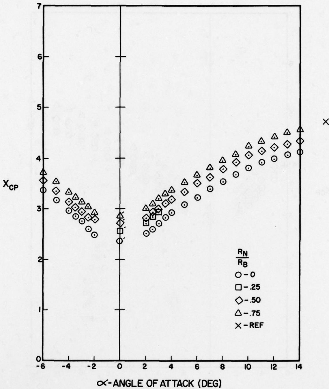
Figure A-123. Center of Pressure Versus Angle of Attack for  $l_N/d = 3$ ,  $l_A/d = 6$ ,  $M = 3.0$
