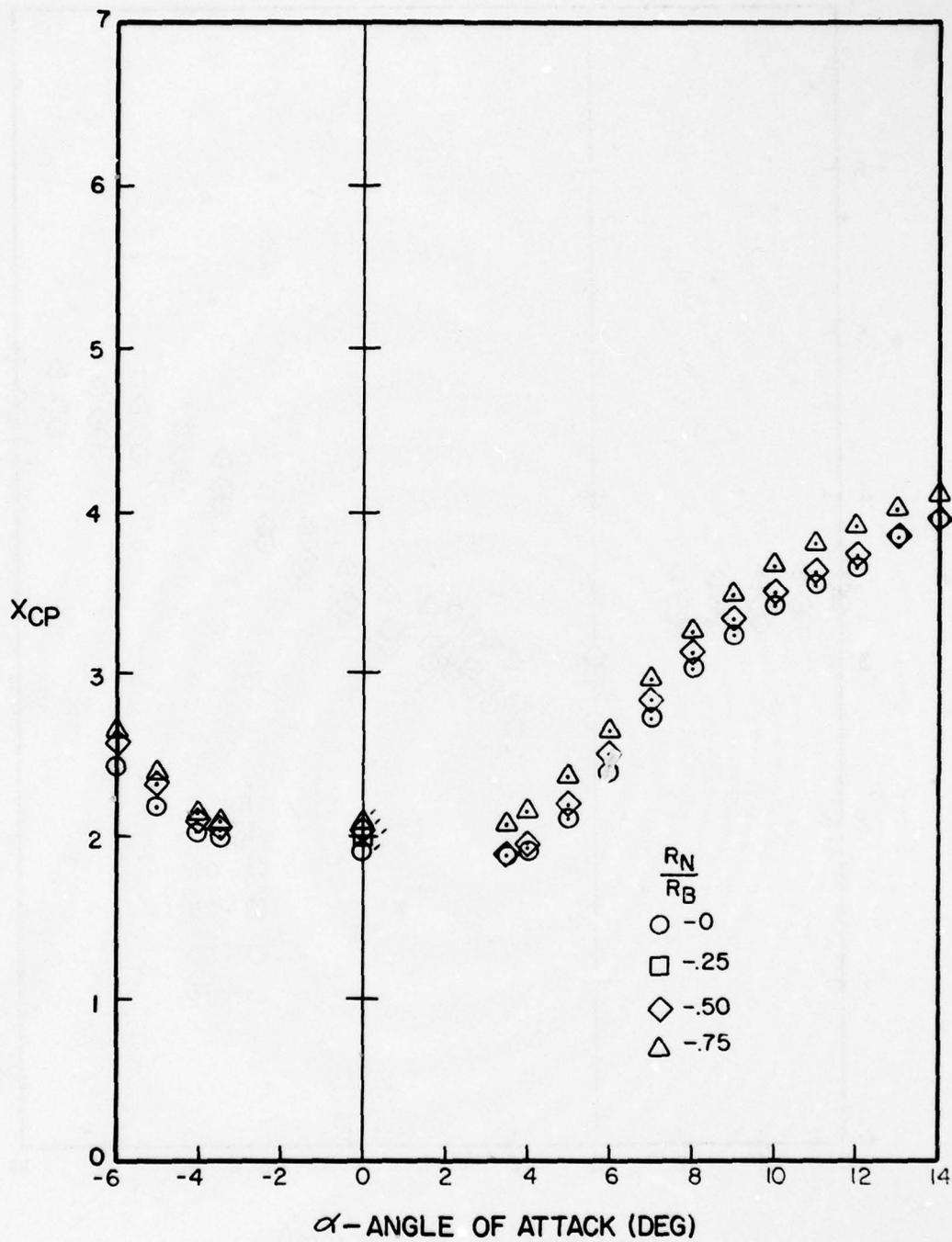
Figure A-116. Center of Pressure Versus Angle of Attack for  $l_N/d = 2$ ,  $l_A/d = 8$ ,  $M = 2.0$
