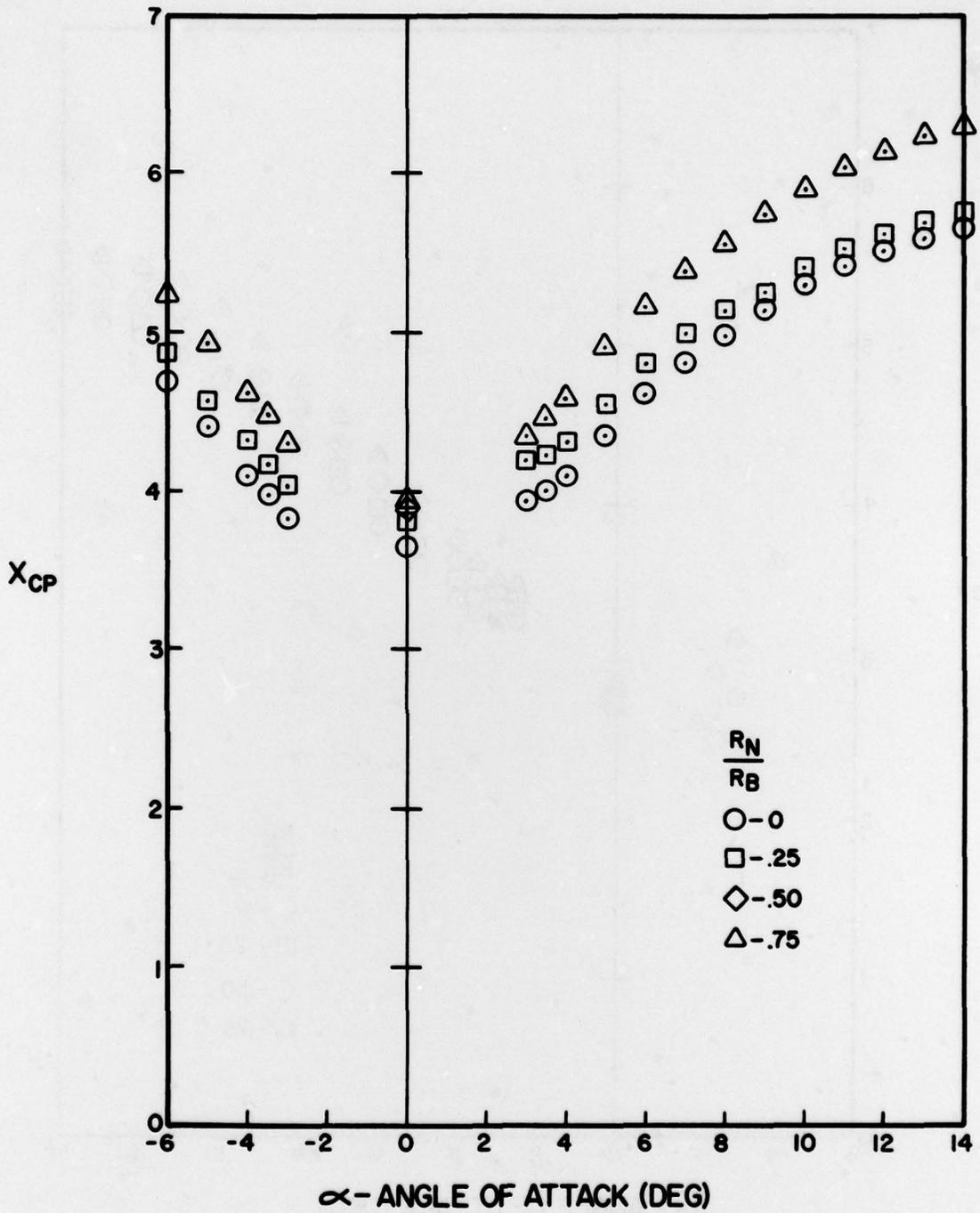
Figure A-133. Center of Pressure Versus Angle of Attack for  $l_N/d = 4$ ,  $l_A/d = 8$ ,  $M = 4.0$
