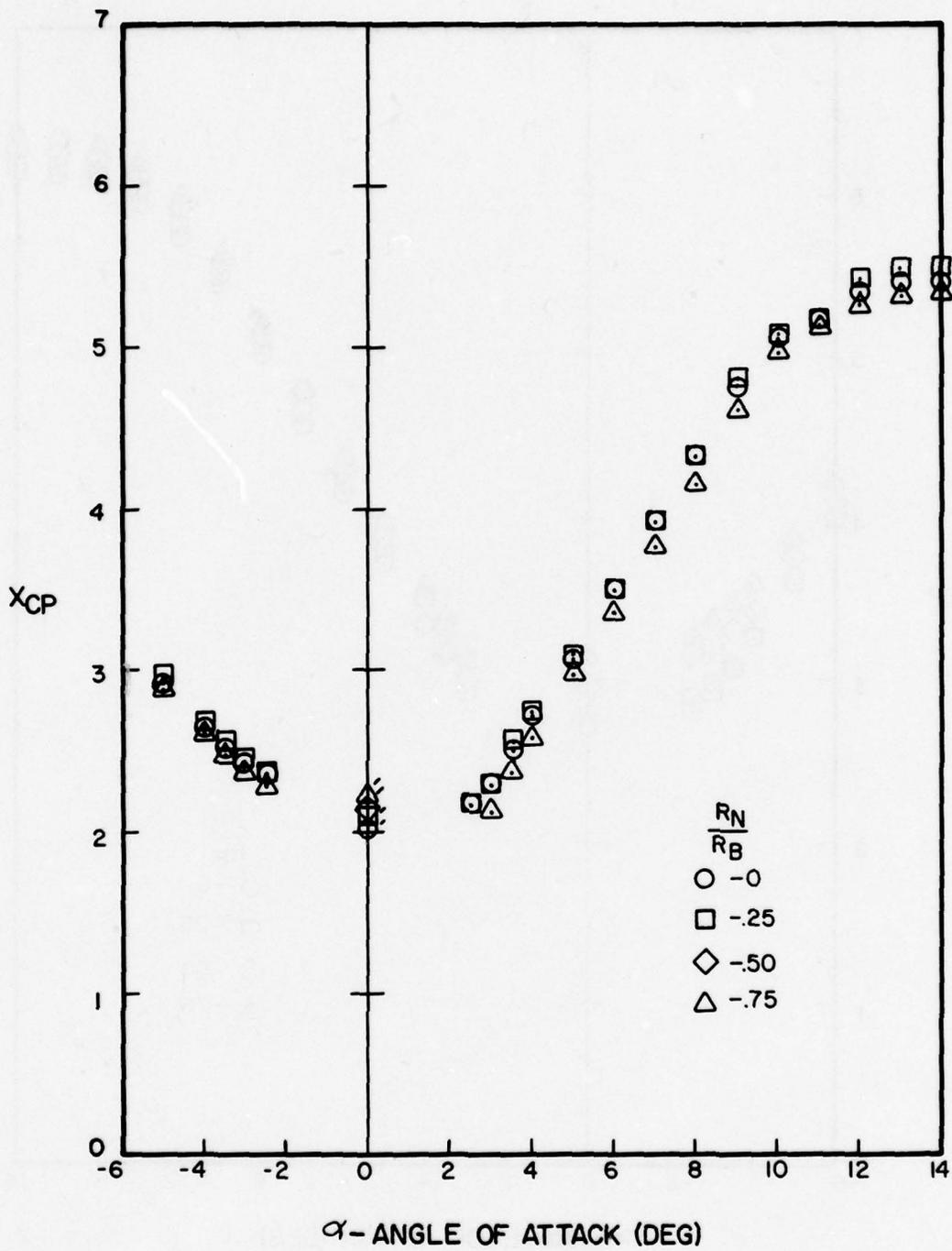
Figure A-111. Center of Pressure Versus Angle of Attack for  $l_N/d = 3$ ,  $l_A/d = 10$ ,  $M = 1.5$
