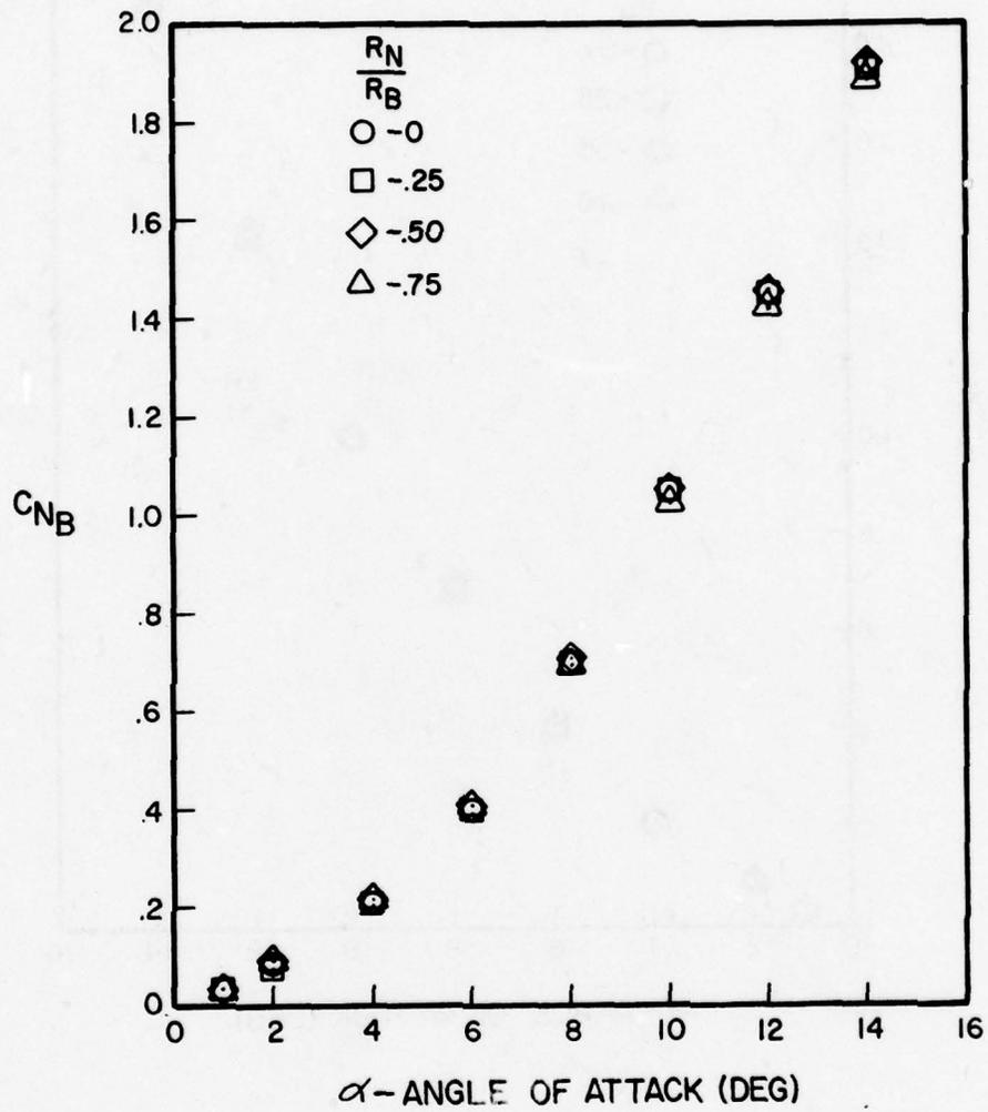
Figure A-64. Normal Force Coefficient Versus Angle of Attack for  $l_N/d = 4$ ,  $l_A/d = 10$ ,  $M = 2.0$
