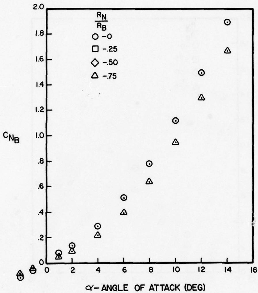
Figure A-77. Normal Force Coefficient Versus Angle of Attack for  $l_N/d = 2$ ,  $l_A/d = 10$ ,  $M = 4.0$
