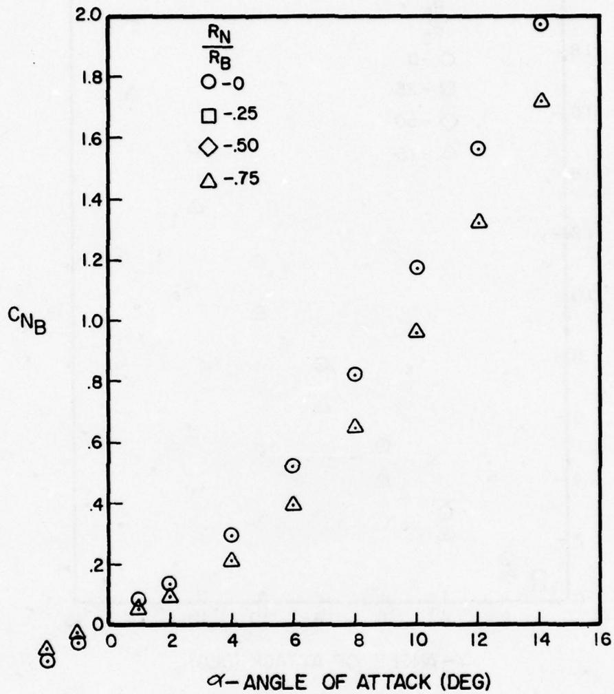
Figure A-78. Normal Force Coefficient Versus Angle of Attack for  $l_N/d = 3$ ,  $l_A/d = 10$ ,  $M = 4.0$
