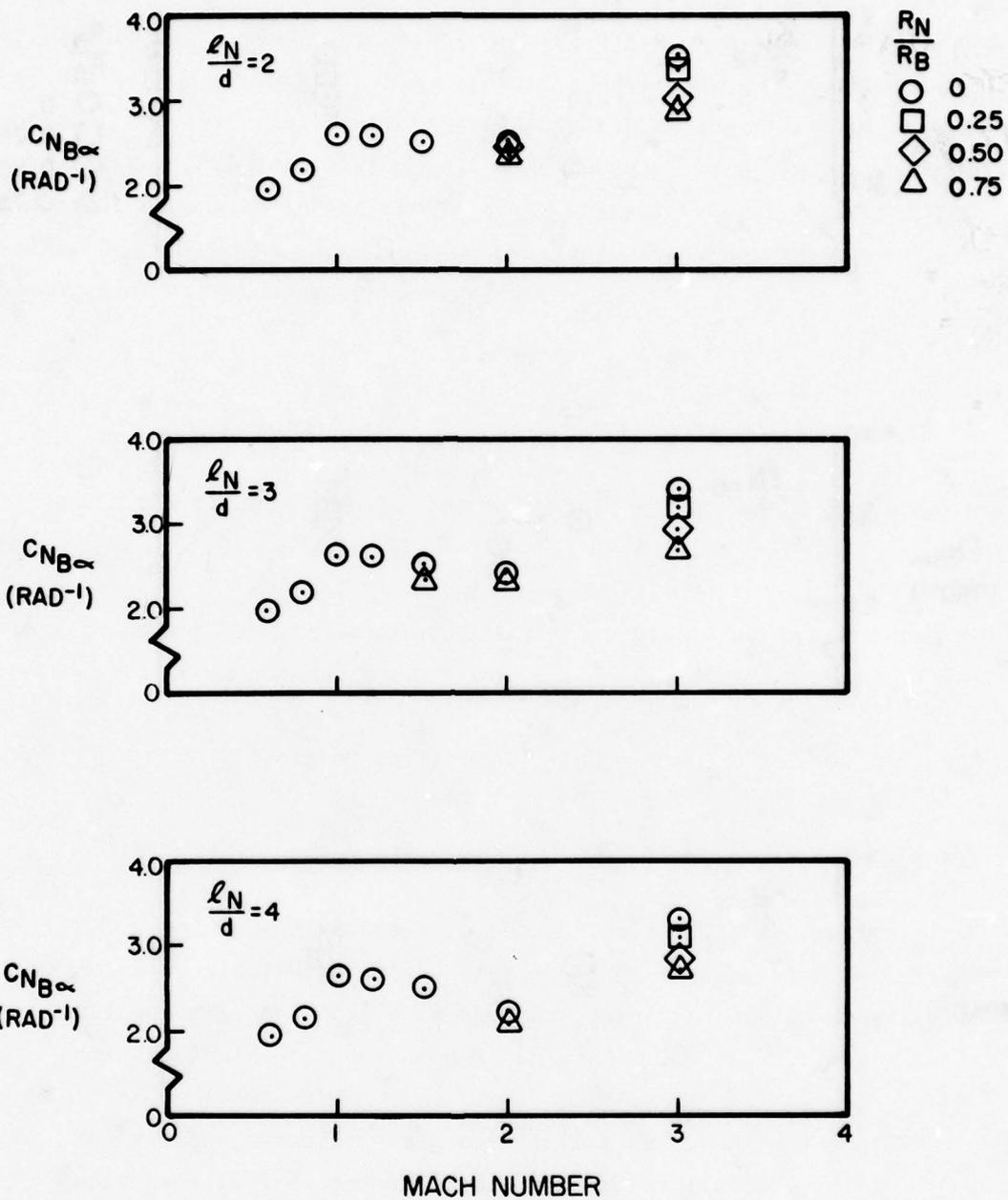
Figure 5. Variation of  $C_{N\alpha}$  with Mach Number for  $\ell_A/d = 6$
