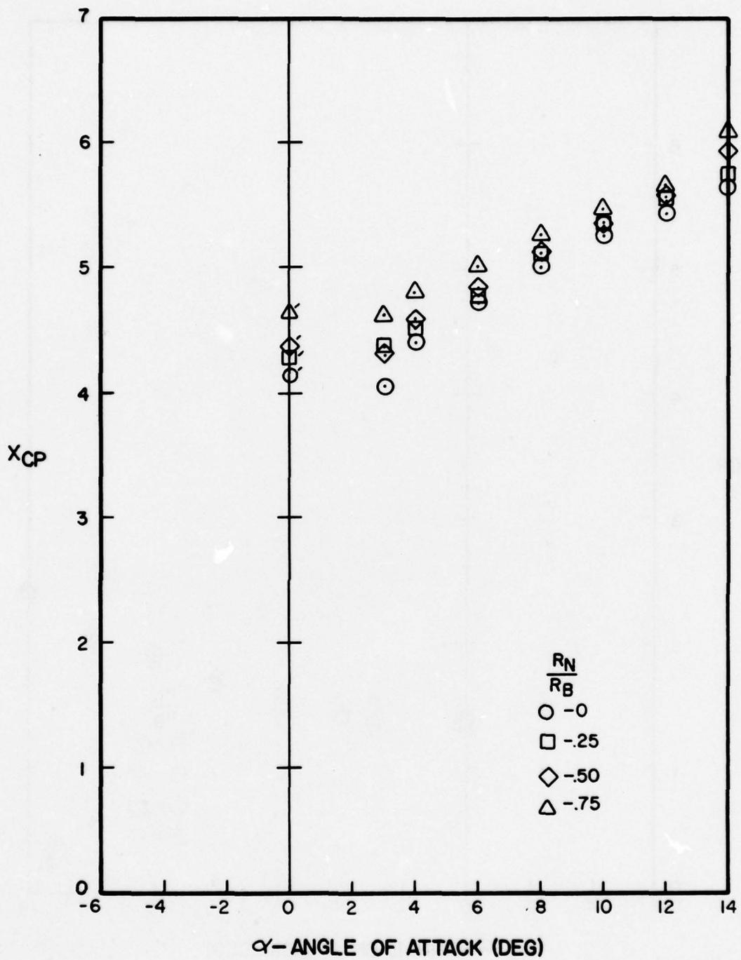
Figure A-97. Center of Pressure Versus Angle of Attack for  $l_N/d = 4$ ,  $l_A/d = 10$ ,  $M = 1.0$
