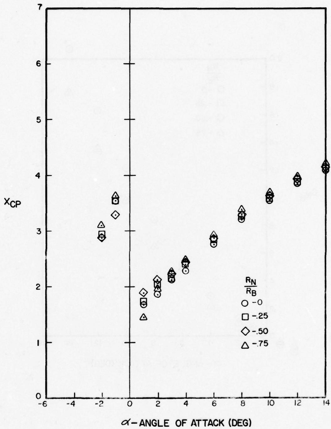
Figure A-80. Center of Pressure Versus Angle of Attack for  $l_N/d = 2$ ,  $l_A/d = 6$ ,  $M = 0.6$
