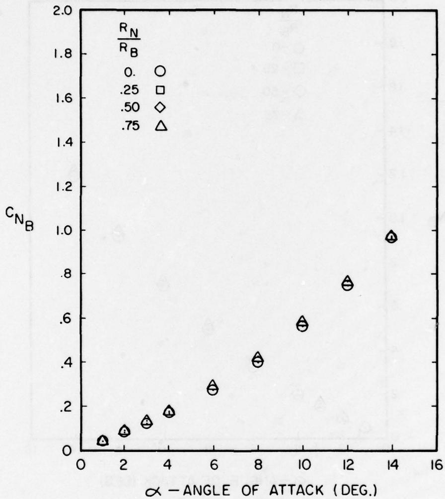
Figure A-43. Normal Force Coefficient Versus Angle of Attack for  $\lambda_N/d = 4$ ,  $\lambda_A/d = 6$ ,  $M = 1.2$
