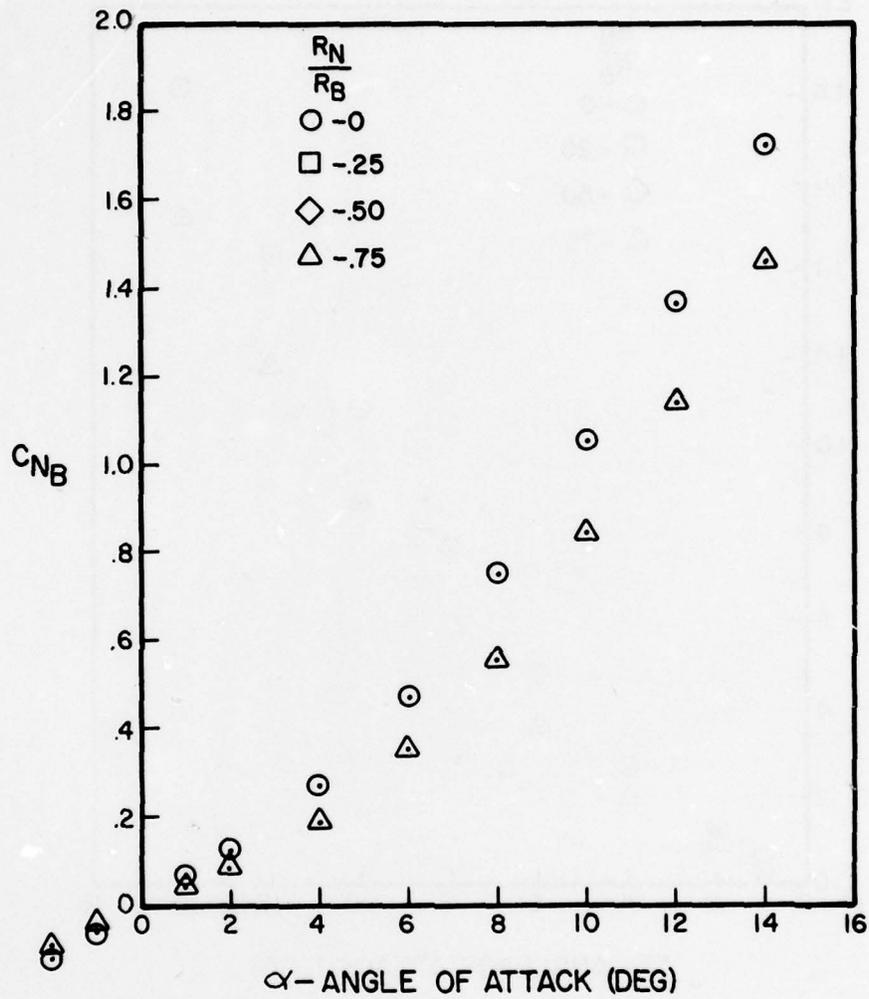
Figure A-75. Normal Force Coefficient Versus Angle of Attack for  $l_N/d = 3$ ,  $l_A/d = 8$ ,  $M = 4.0$
