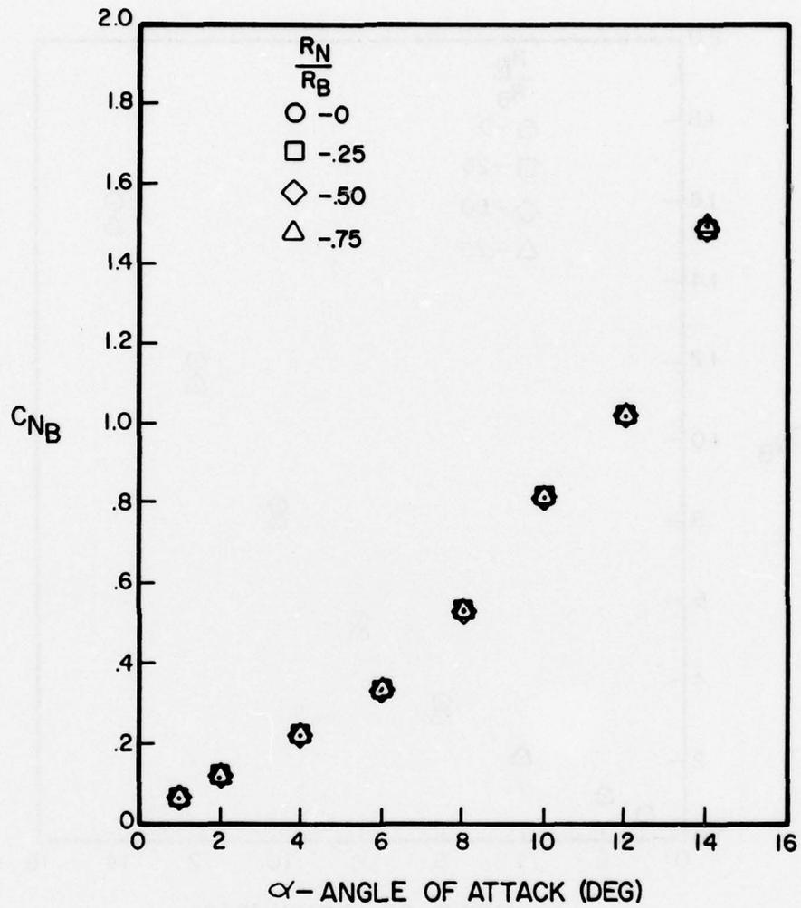
Figure A-51. Normal Force Coefficient Versus Angle of Attack for  $l_N/d = 2$ ,  $l_A/d = 8$ ,  $M = 1.5$
