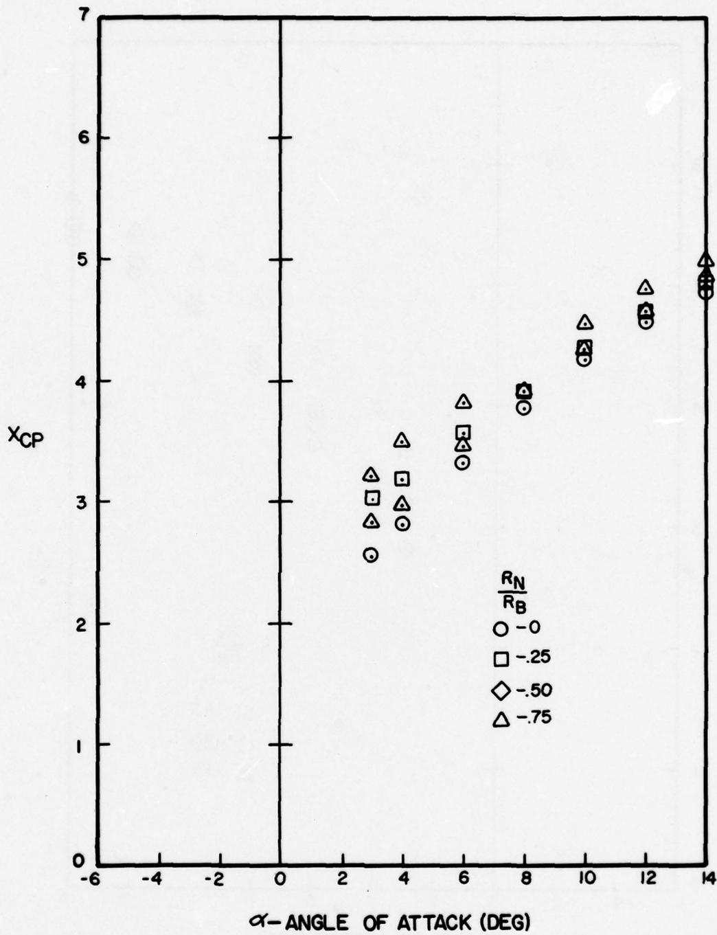
Figure A-81. Center of Pressure Versus Angle of Attack for  $l_N/d = 3$ ,  $l_A/d = 6$ ,  $M = 0.6$
