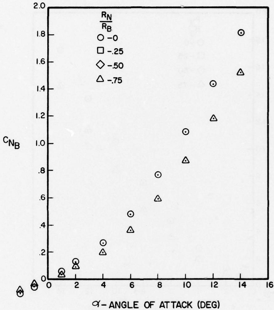
Figure A-76. Normal Force Coefficient Versus Angle of Attack for  $l_N/d = 4$ ,  $l_A/d = 8$ ,  $M = 4.0$
