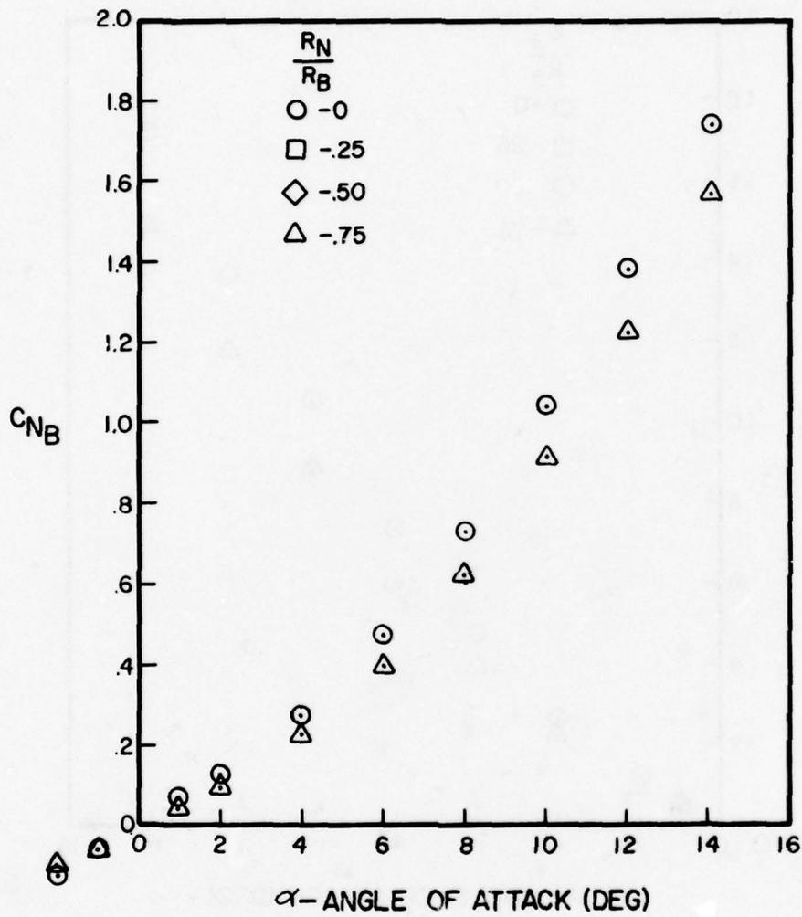
Figure A-68. Normal Force Coefficient Versus Angle of Attack for  $l_N/d = 2$ ,  $l_A/d = 8$ ,  $M = 3.0$
