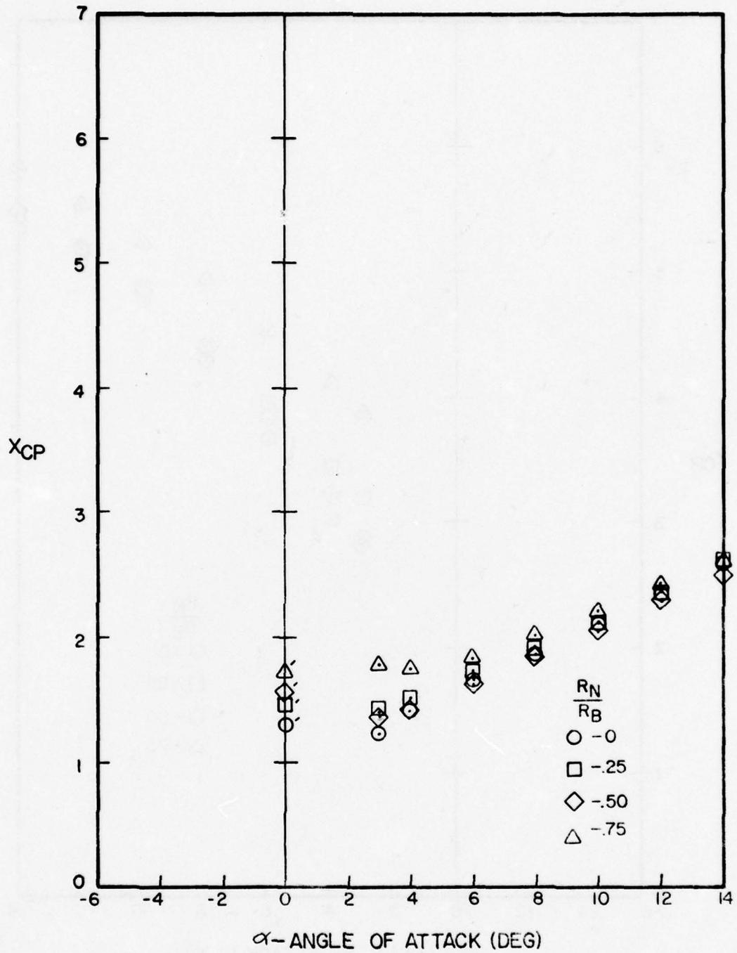
Figure A-86. Center of Pressure Versus Angle of Attack for  $l_N/d = 2$ ,  $l_A/d = 6$ ,  $M = 0.8$
