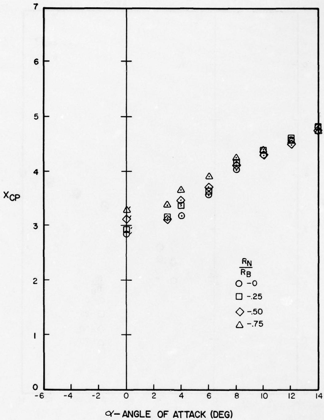
Figure A-102. Center of Pressure Versus Angle of Attack for  $l_N/d = 3$ ,  $l_A/d = 10$ ,  $M = 1.2$
