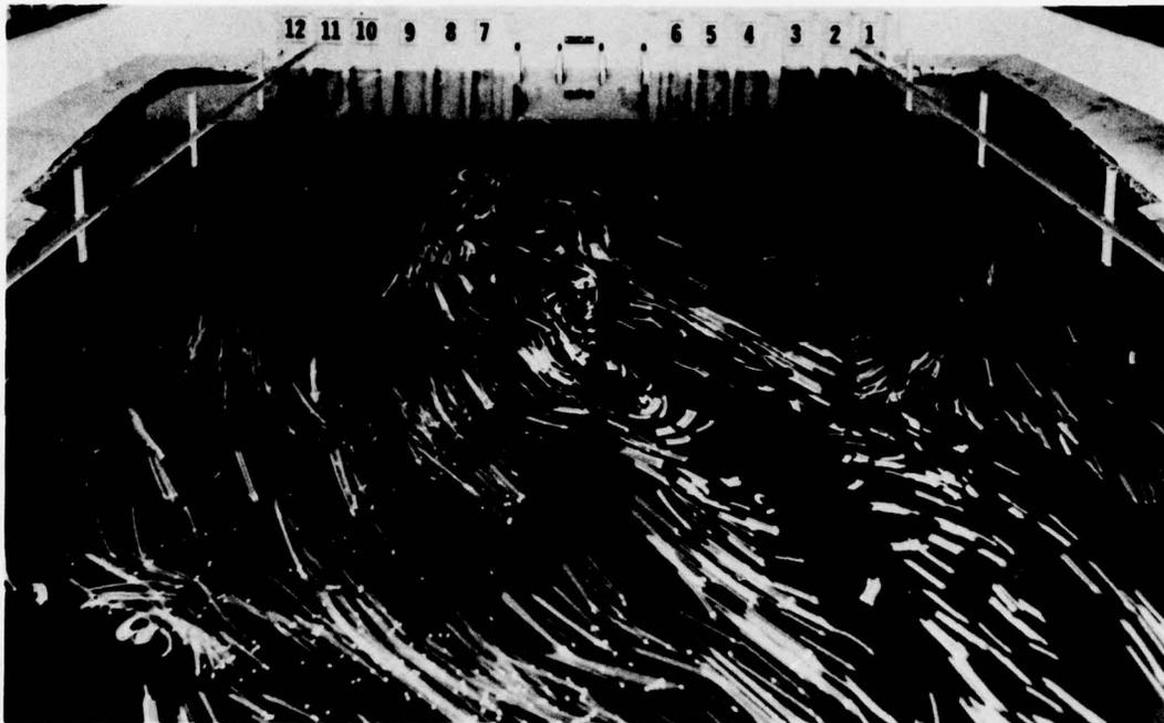
Photo 15. Pumps operating: 2, 4, 6, 7, 9, 11. Discharge per pumps 6 and 7, 250 cfs; pumps 2, 4, 9, 11, 600 cfs; tailwater el 620 ft
