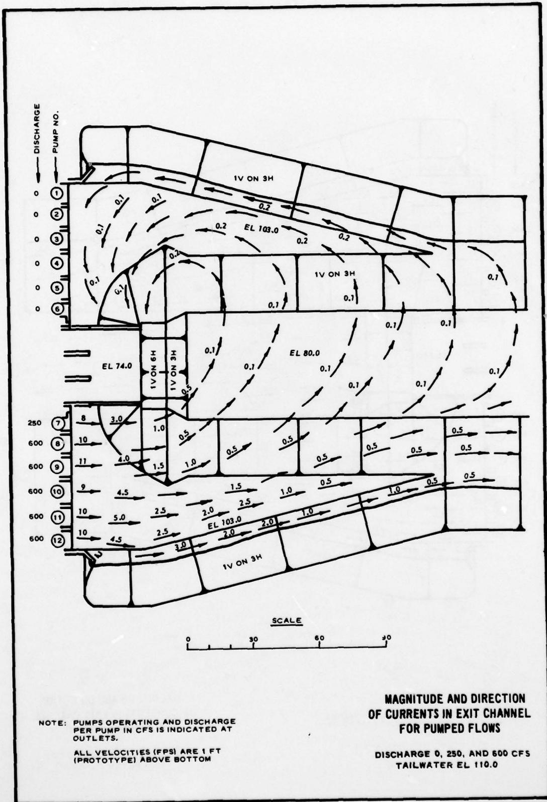
NOTE: PUMPS OPERATING AND DISCHARGE PER PUMP IN CFS IS INDICATED AT OUTLETS.
