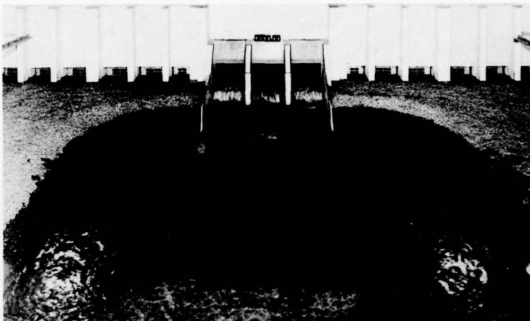
a. Discharge 5,000 cfs, tailwater el 91.0
