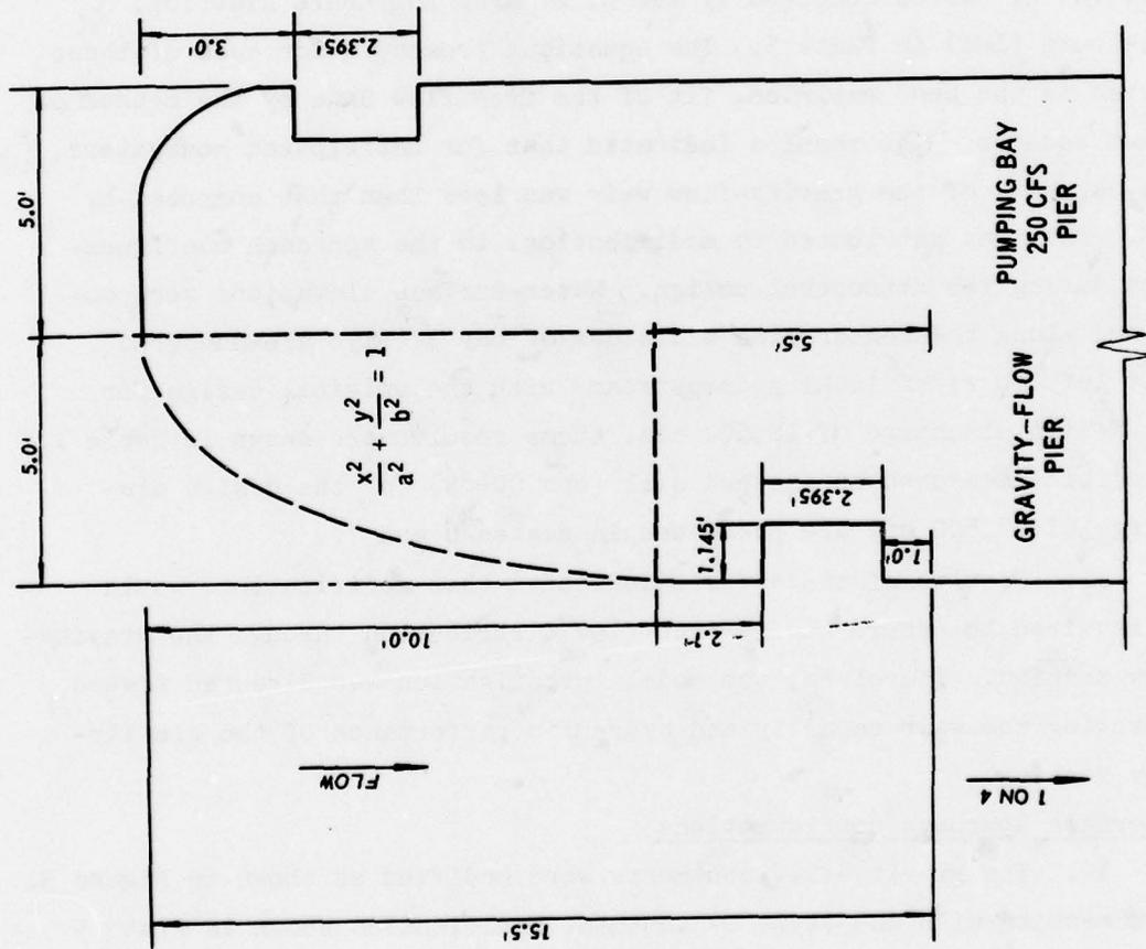
Figure 3. Details of gravity-flow section abutment type 2 modification
