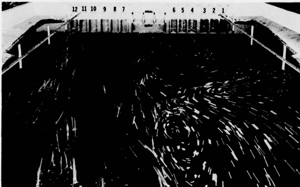
Photo 16. Pumps operating: 7, 8, 9, 10, 11, 12. Discharge per pump 7, 250 cfs; pumps 8, 9, 10, 11, 12, 600 cfs; tailwater el 620 ft
