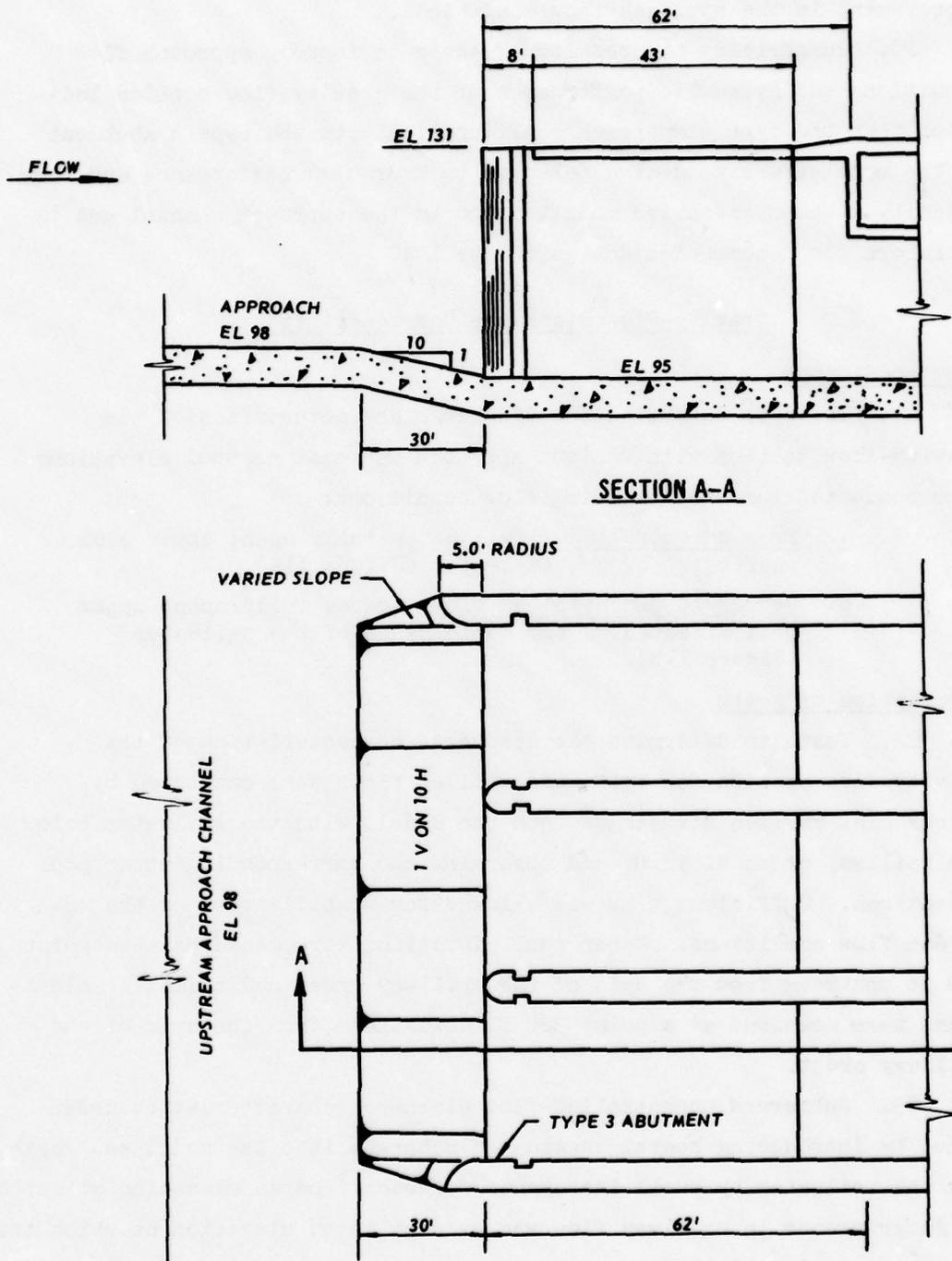
Figure 10. Plan and section of type 8 approach and type 3 abutment
