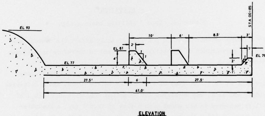
Figure 15. Details of type 7 stilling basin design
