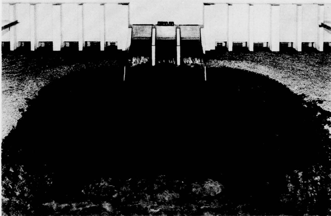
c. Discharge 12,500 cfs, tailwater el 92.8
