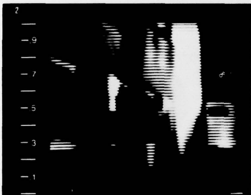
Figure 115. Cooler thermal pattern below the breeching on the chimney.
