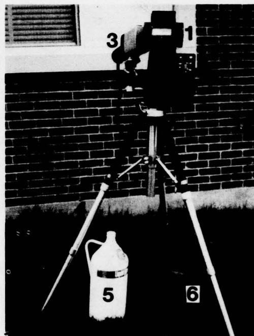
Figure 2. Portable thermal scanner system. 1 — Polaroid camera; 2 — display console; 3 — camera and lens; 4 — tripod; 5 — liquid nitrogen bottle; 6 — battery.
